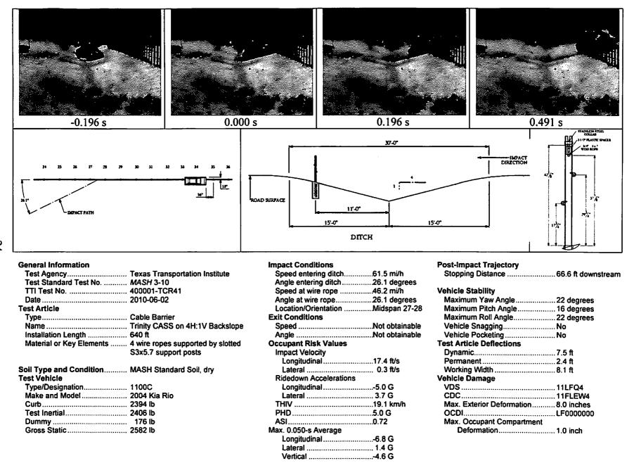
Figure 5.7. Summary of results for MASH test 3-10 on the Trinity CASS on 4H:1V backslope.
