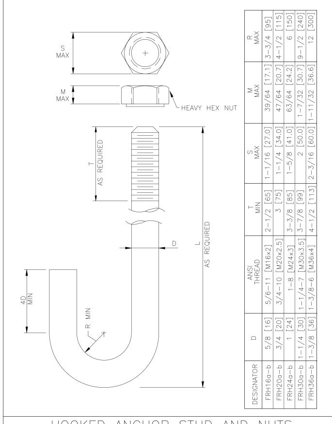
HOOKED ANCHOR STUD AND NUTS
