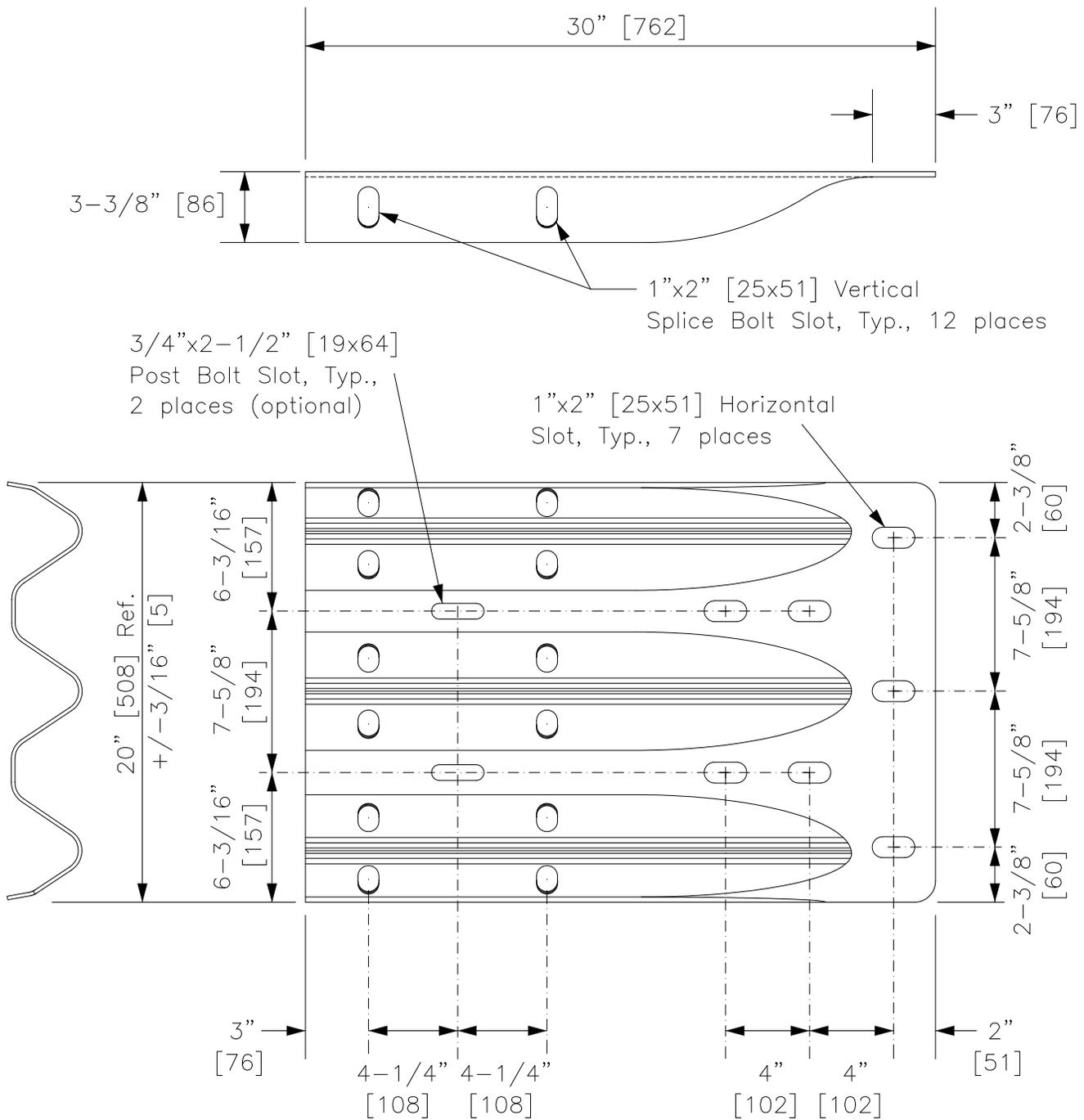
Cross-Section Dimensions are to fit Over or Under Rail Components RTM01a-RTM06b, See RTM01a-02b Sheet 3 of 4 for Details.
