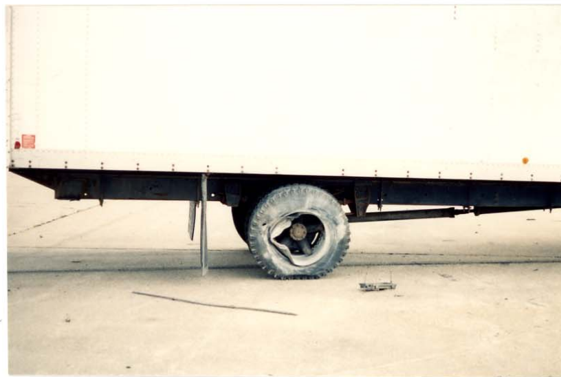
Figure 16. Test Vehicle Damage, Test MN-1.
