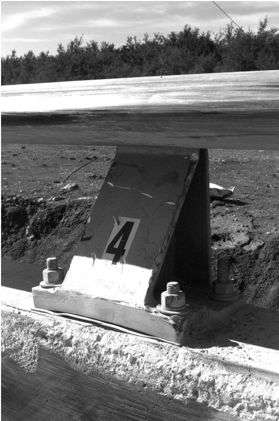
Figure 8. Damage at Post 4 after Test 418049-7.
