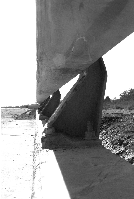
Figure 8. Damage at Post 4 after Test 418049-7.
