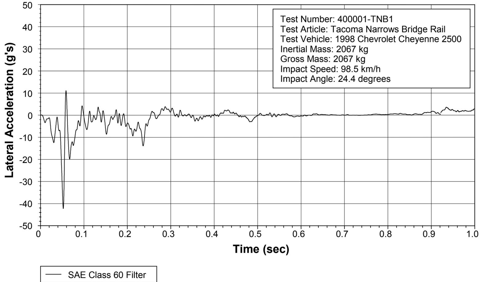
Figure 15. Vehicle lateral accelerometer trace for test 400001-TNB1 (accelerometer located at center of gravity).
