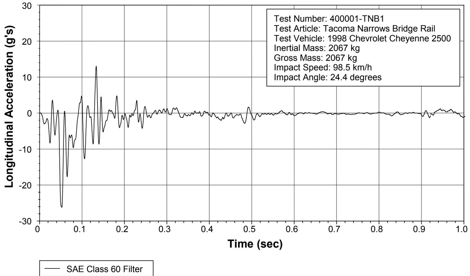
Figure 14. Vehicle longitudinal accelerometer trace for test 400001-TNB1 (accelerometer located at center of gravity).
