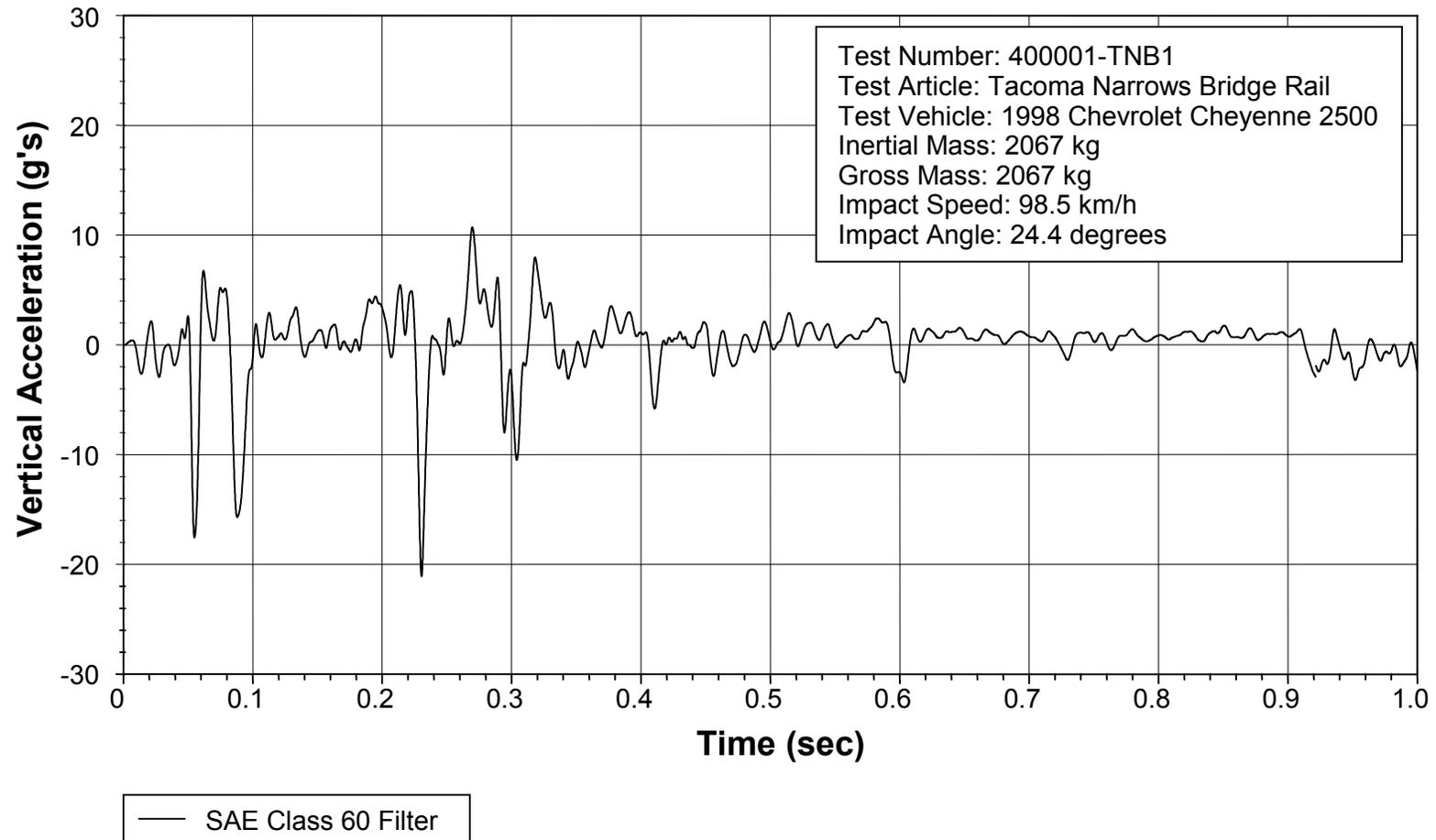
Figure 19. Vehicle vertical accelerometer trace for test 400001-TNB1
