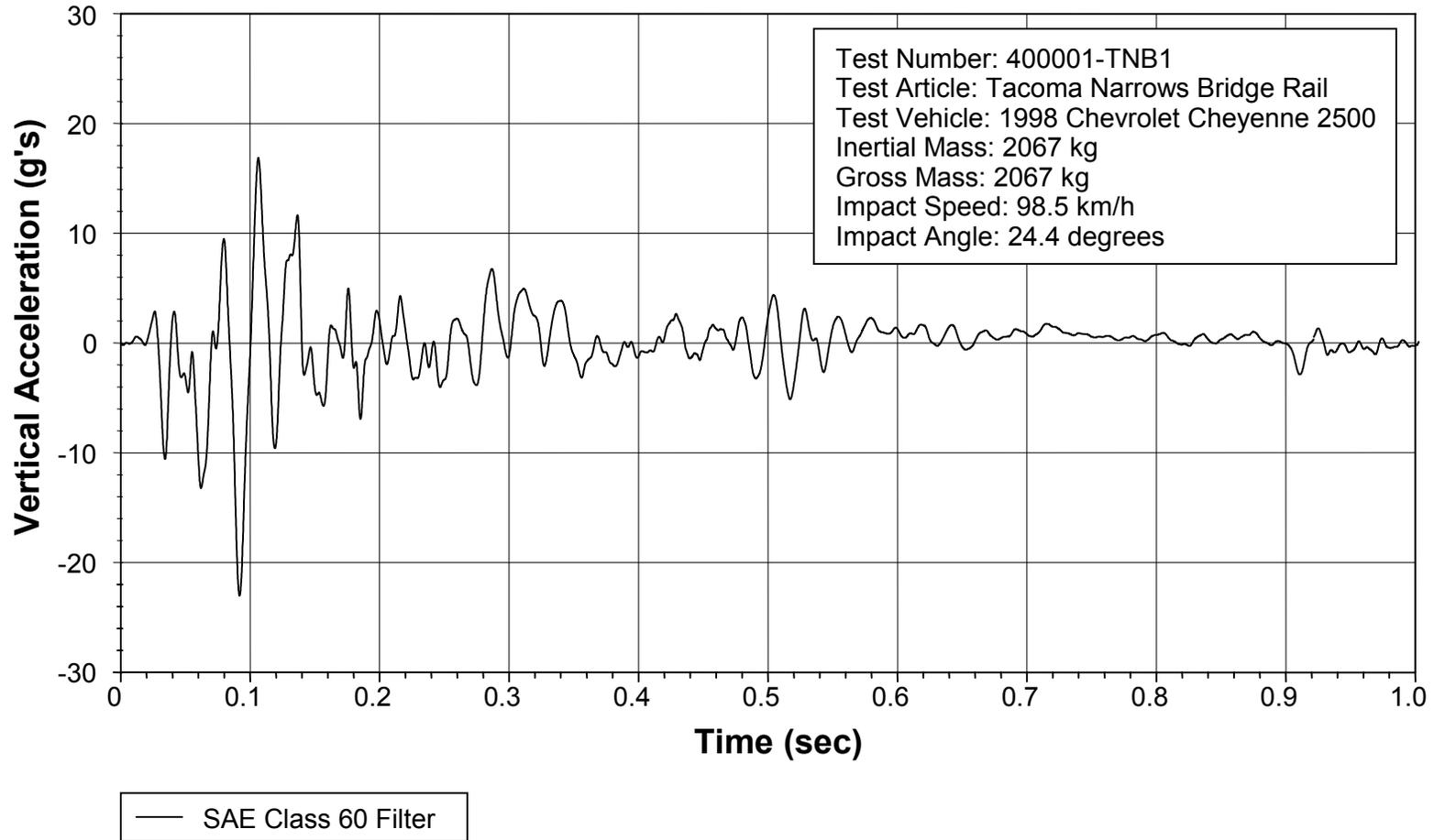
Figure 16. Vehicle vertical accelerometer trace for test 400001-TNB1 (accelerometer located at center of gravity).
