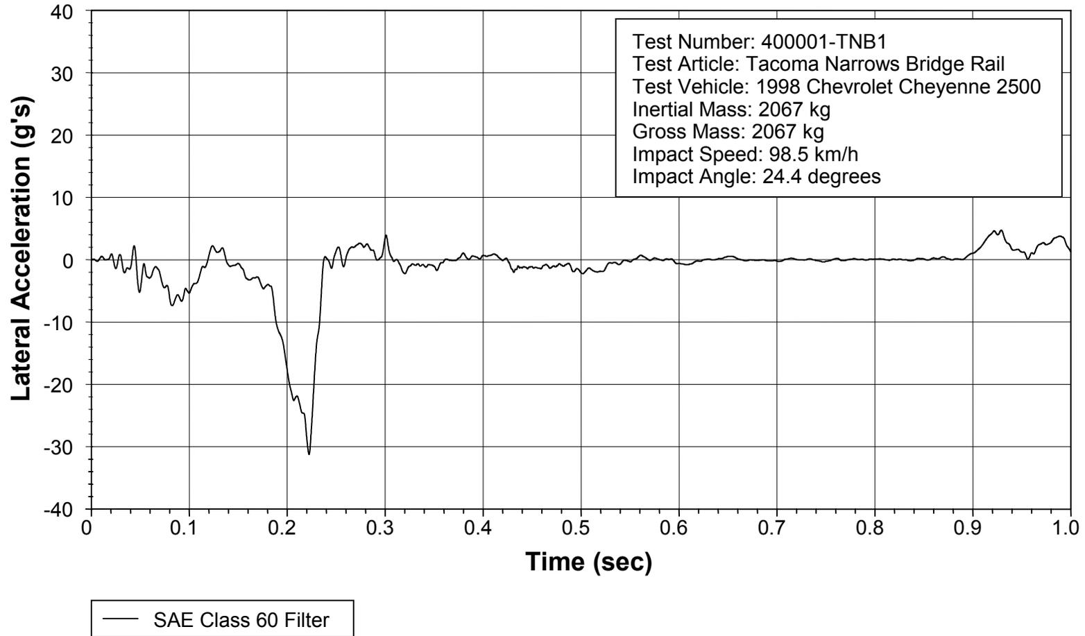
Figure 18. Vehicle lateral accelerometer trace for test 400001-TNB1 (accelerometer located over rear axle).
