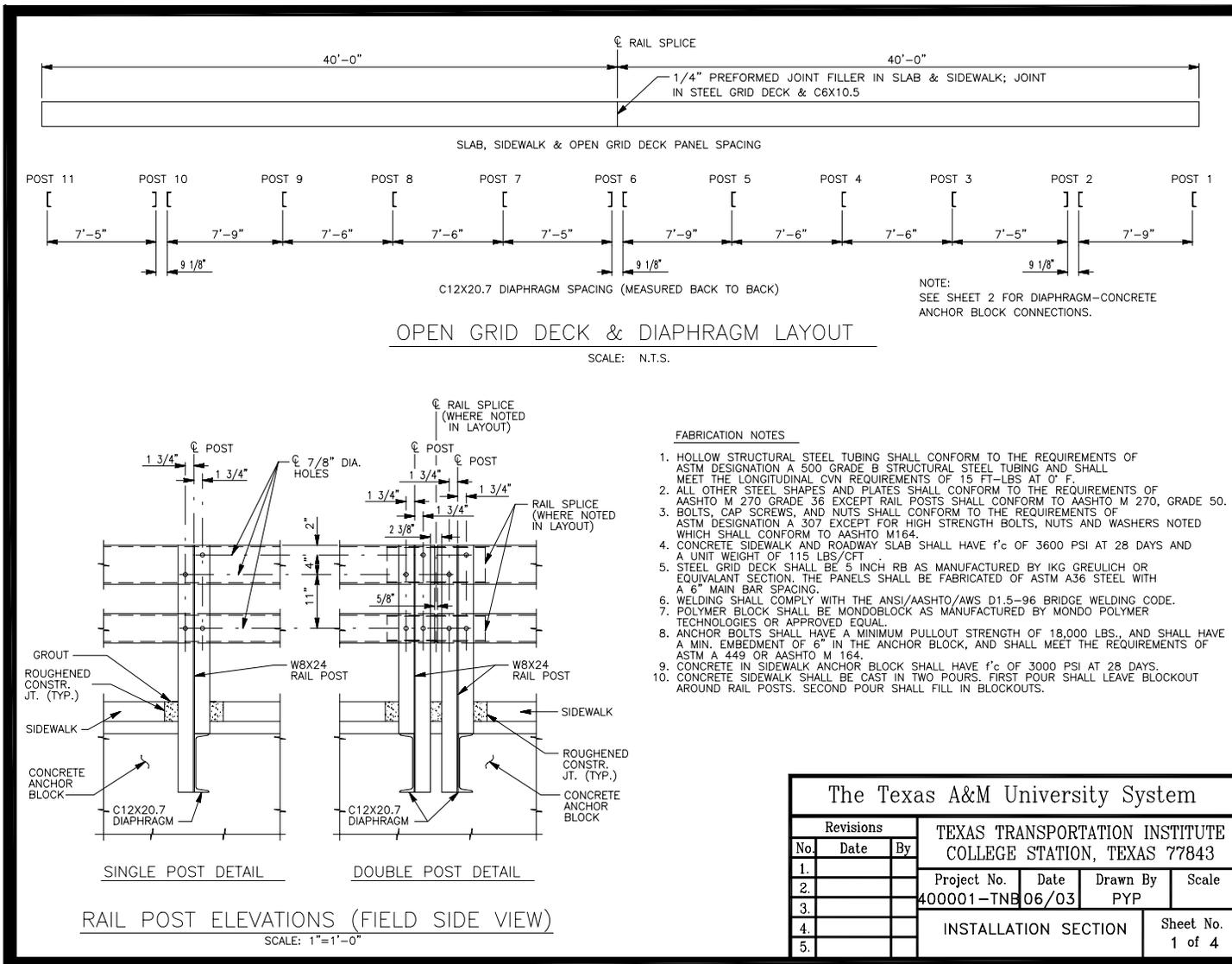
Figure 1. Details of the Tacoma Narrows Bridge Rail.
