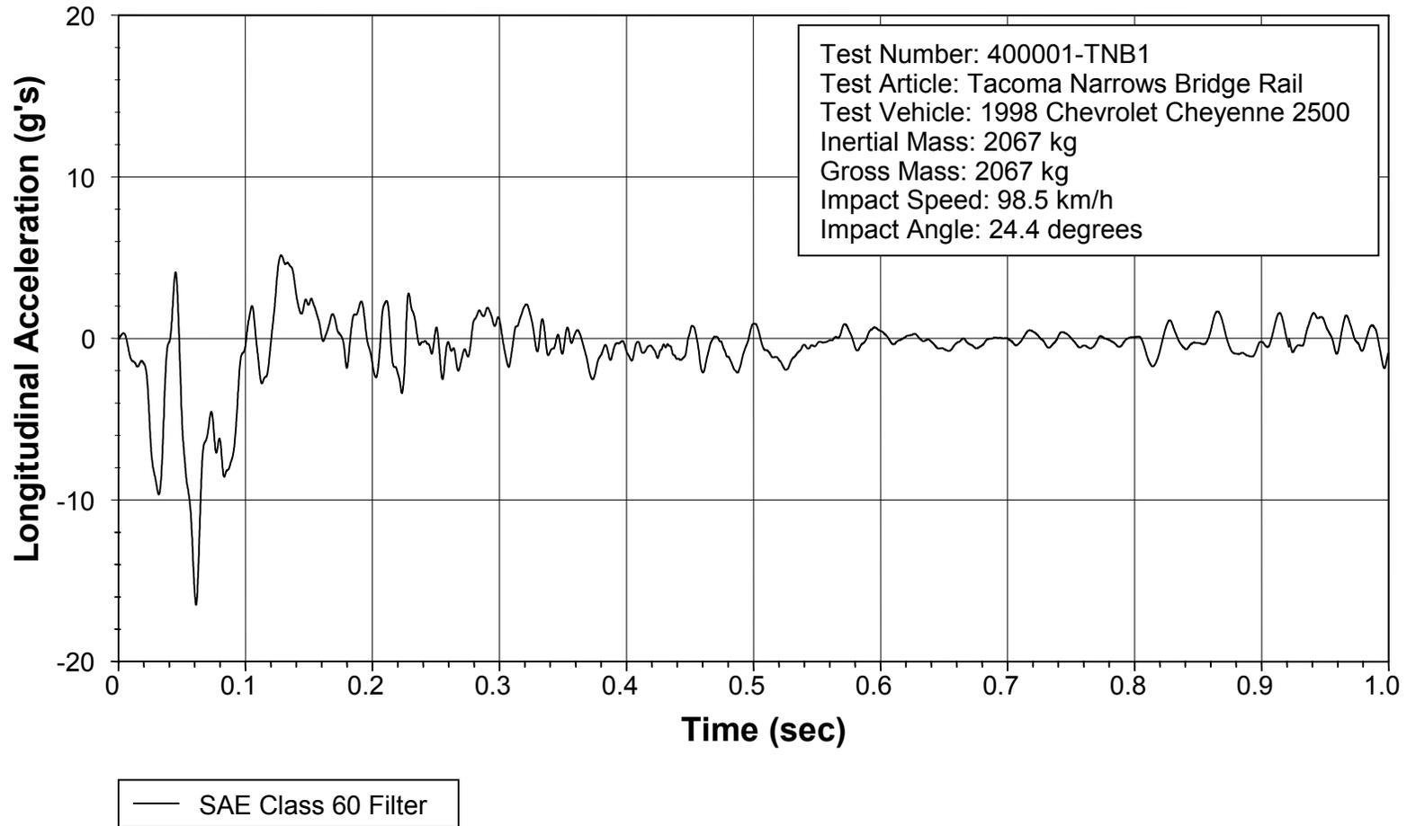
Figure 17. Vehicle longitudinal accelerometer trace for test 400001-TNB1 (accelerometer located over rear axle).
