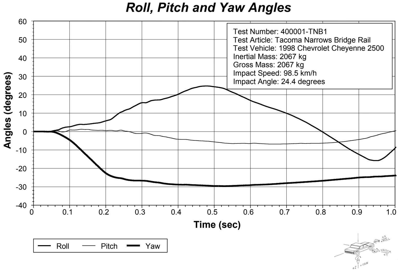
Figure 13. Vehicle angular displacements for test 400001-TNB1.
