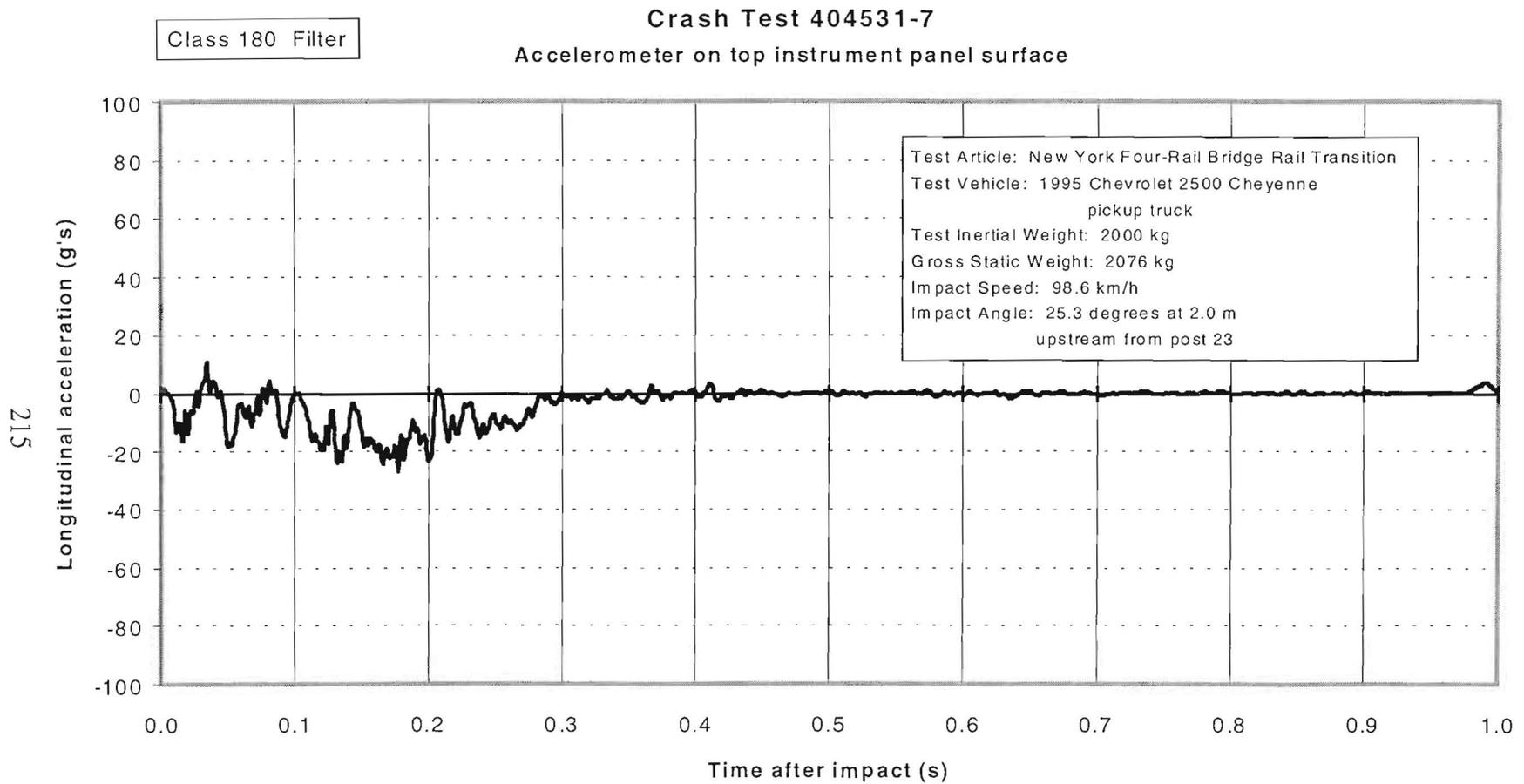
Figure 139. Vehicle longitudinal accelerometer trace for test 404531-7 (accelerometer located on top surface of instrument panel).
