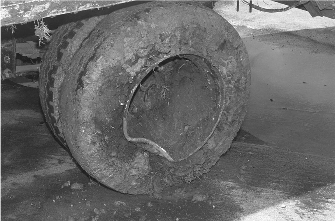
Figure 35. Axle and wheel damage after test 404531-4.
