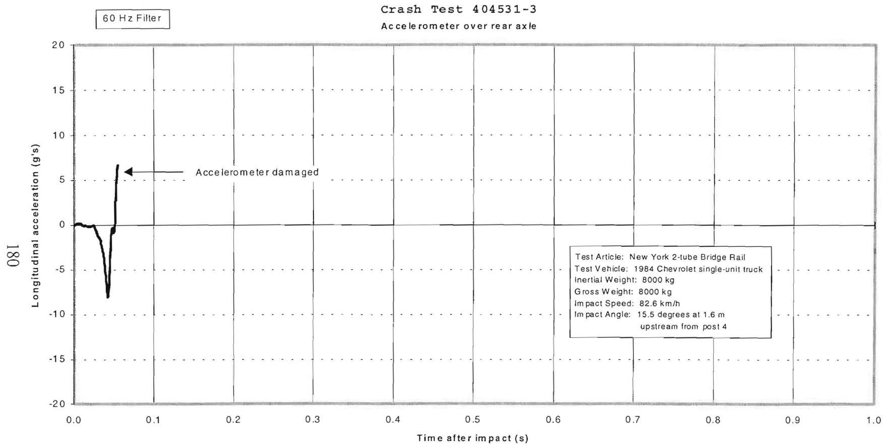
Figure 104. Vehicle longitudinal accelerometer trace for test 404531-3 (accelerometer located in rear of box-van).
