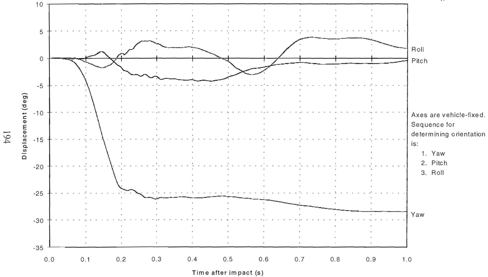
Figure 118. Vehicular angular displacements for test 404531-6.
