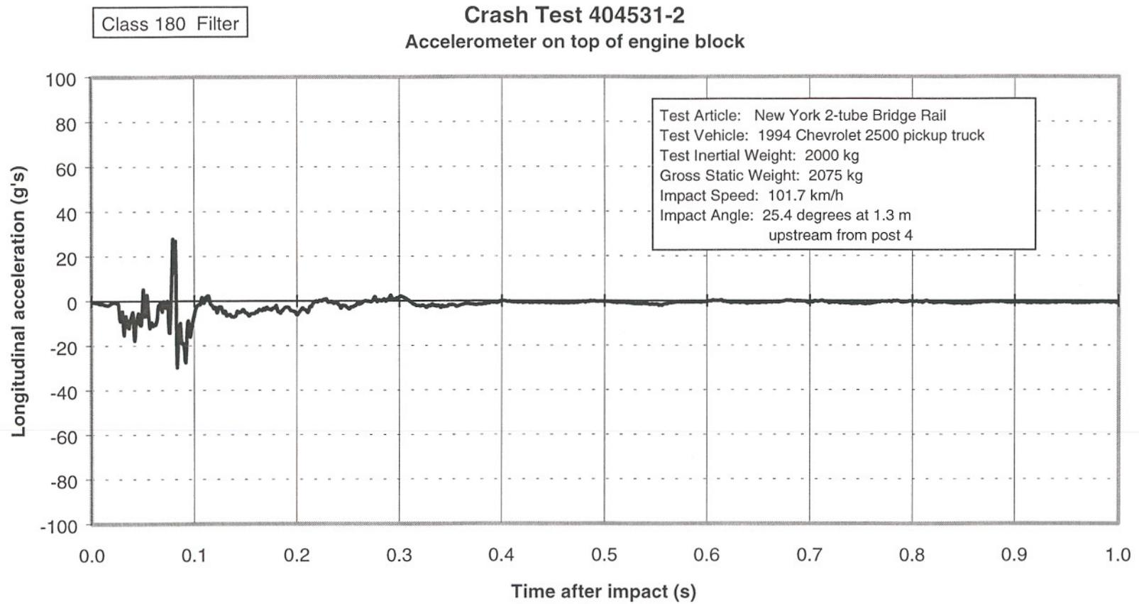
Figure 94. Vehicle longitudinal accelerometer trace for test 404531-2 (accelerometer located on top of engine block).
