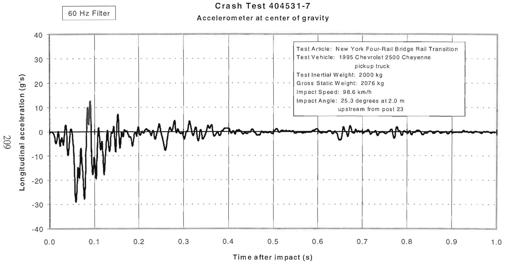
Figure 133. Vehicle longitudinal accelerometer trace for test 404531-7 (accelerometer located at center of gravity).
