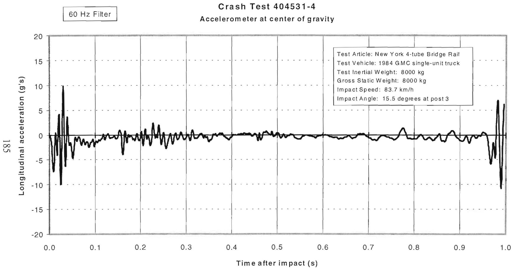
Figure 109. Vehicle longitudinal accelerometer trace for test 404531-4 (accelerometer located at center of gravity).
