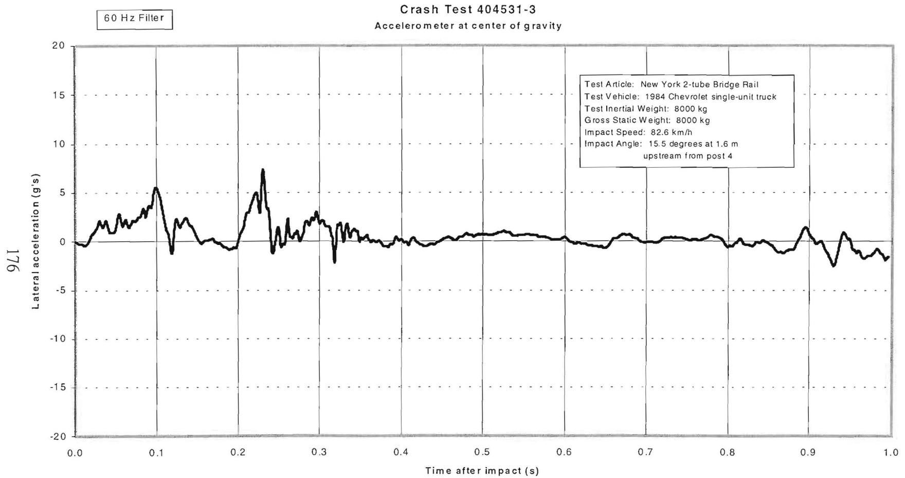
Figure 100. Vehicle lateral accelerometer trace for test 404531-3 (accelerometer located at center of gravity).
