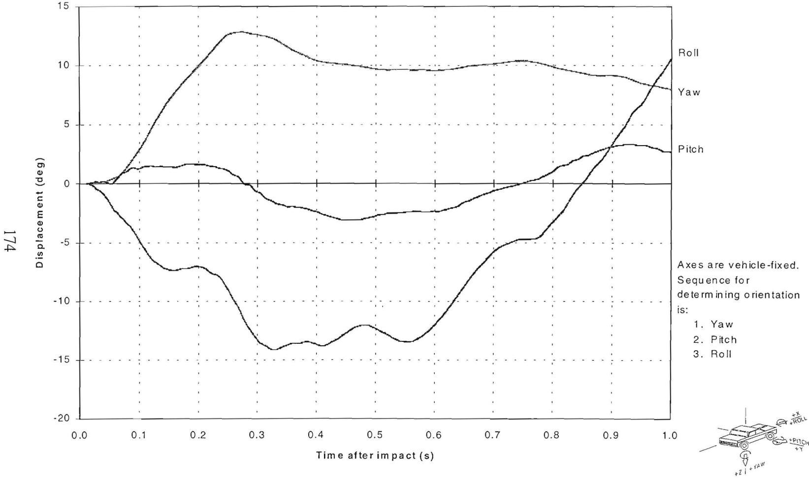
Figure 98. Vehicular angular displacements for test 404531-3.
