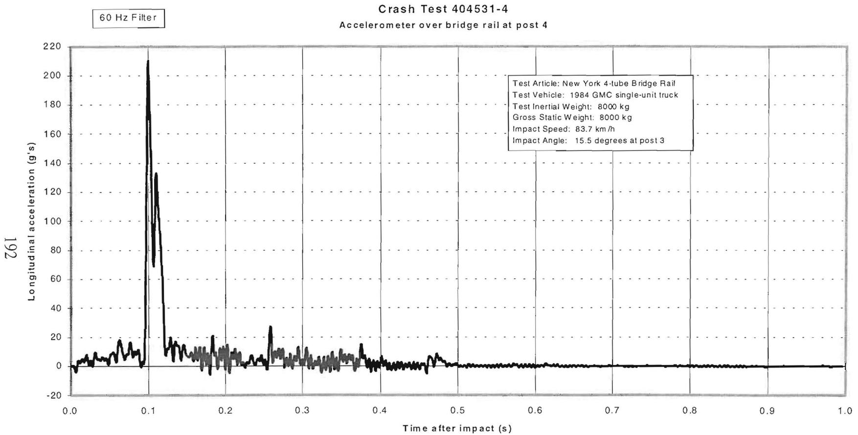
Figure 116. Bridge railing longitudinal accelerometer trace for test 404531-4 (accelerometer located over bridge railing at post 4).
