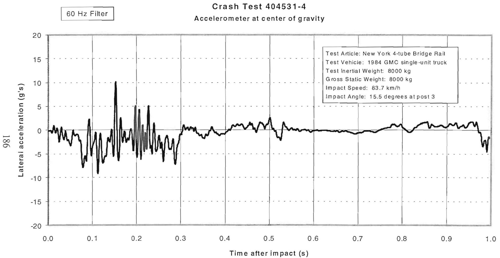
Figure 110. Vehicle lateral accelerometer trace for test 404531-4 (accelerometer located at center of gravity).
