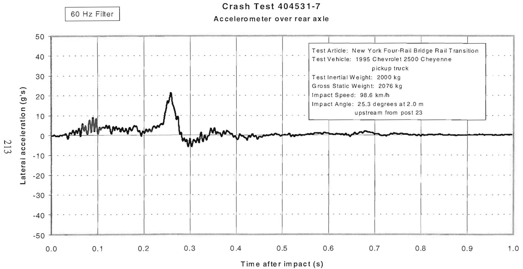
Figure 137. Vehicle lateral accelerometer trace for test 404531-7 (accelerometer located over rear axle).
