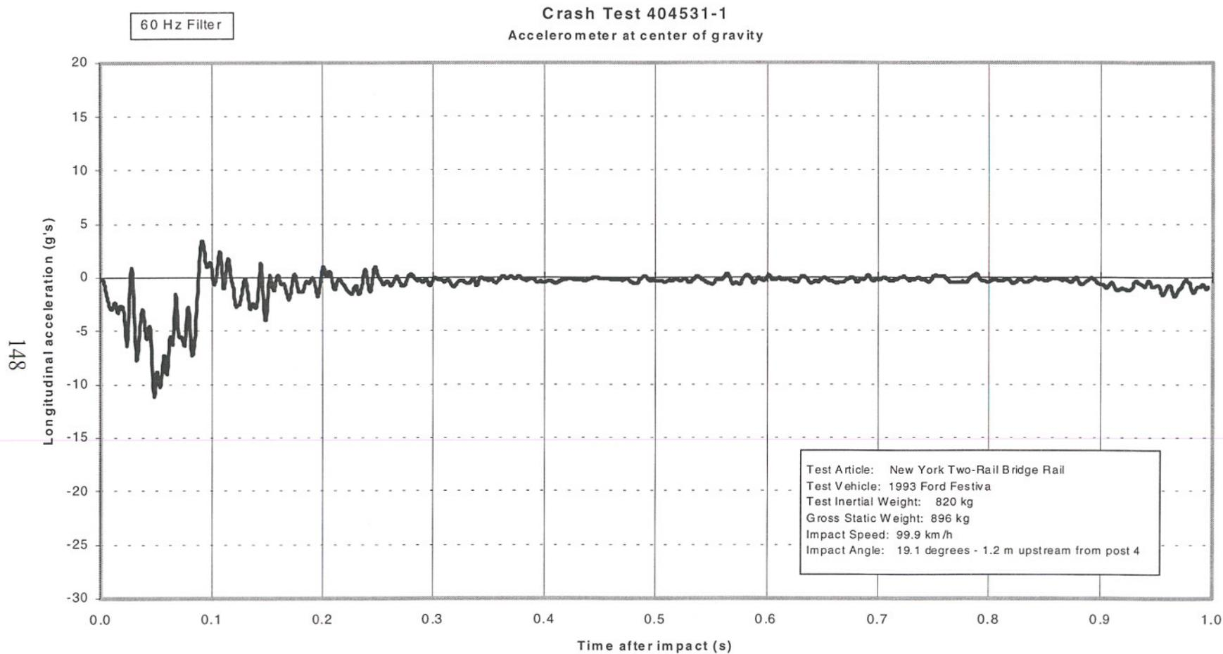
Figure 72. Vehicle longitudinal accelerometer trace for test 404531-1 (accelerometer located at center of gravity).
