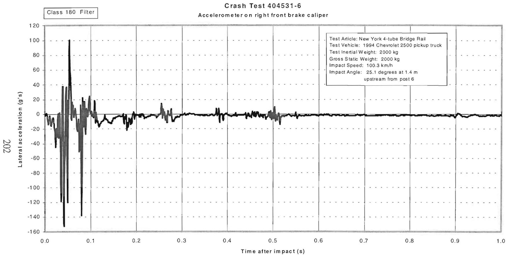
Figure 126. Vehicle lateral accelerometer trace for test 404531-6 (accelerometer located on right front brake caliper).
