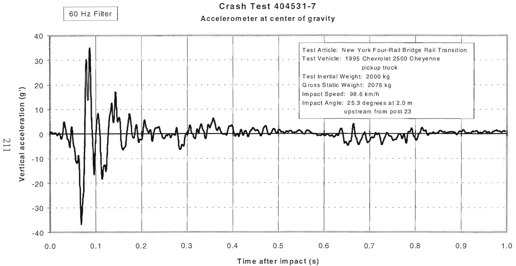
Figure 135. Vehicle vertical accelerometer trace for test 404531-7 (accelerometer located at center of gravity).
