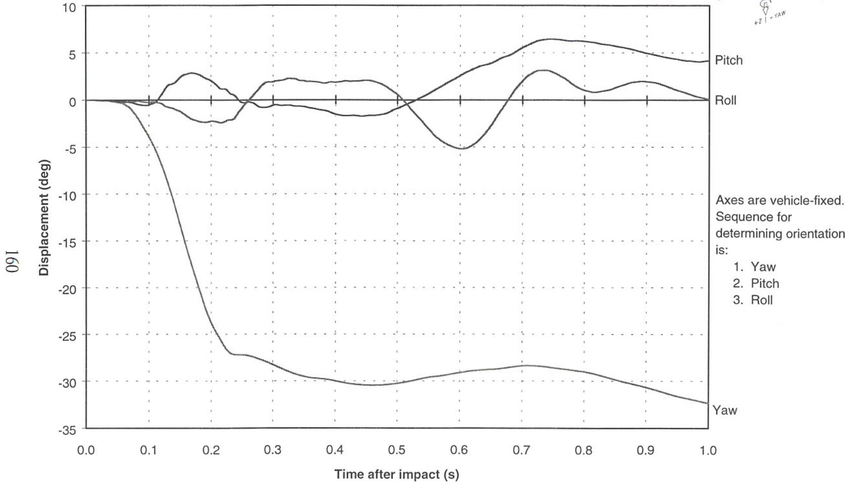
Figure 84. Vehicular angular displacements for test 404531-2.
