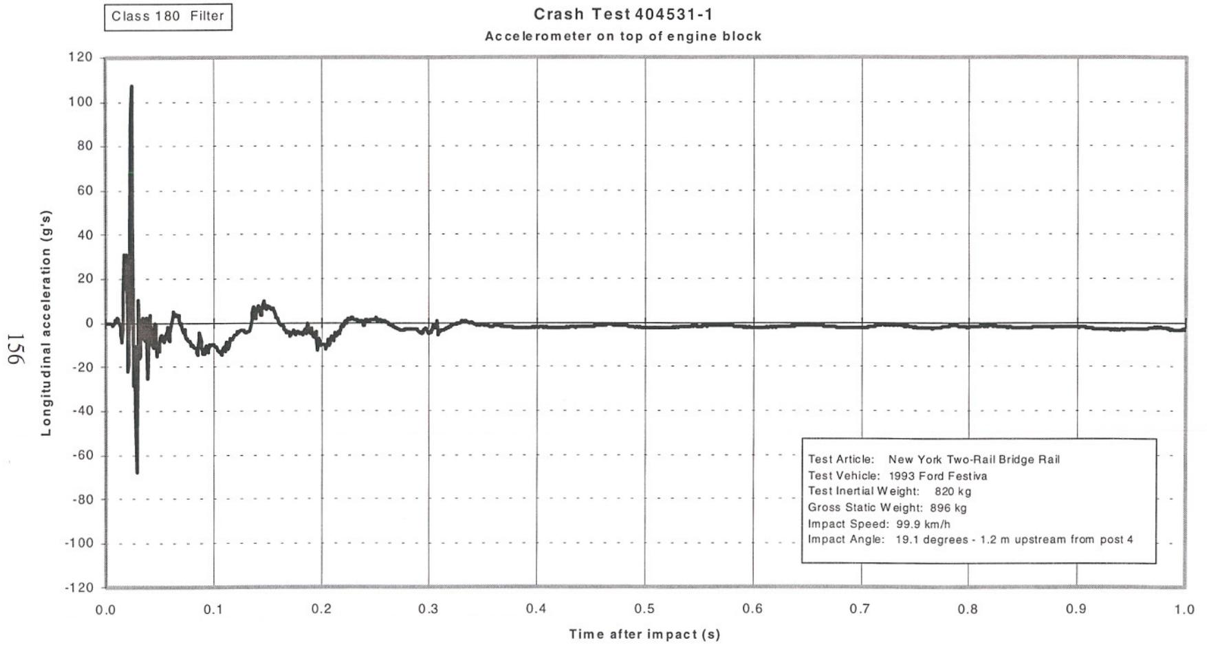
Figure 80. Vehicle longitudinal accelerometer trace for test 404531-1 (accelerometer located on top of engine block).
