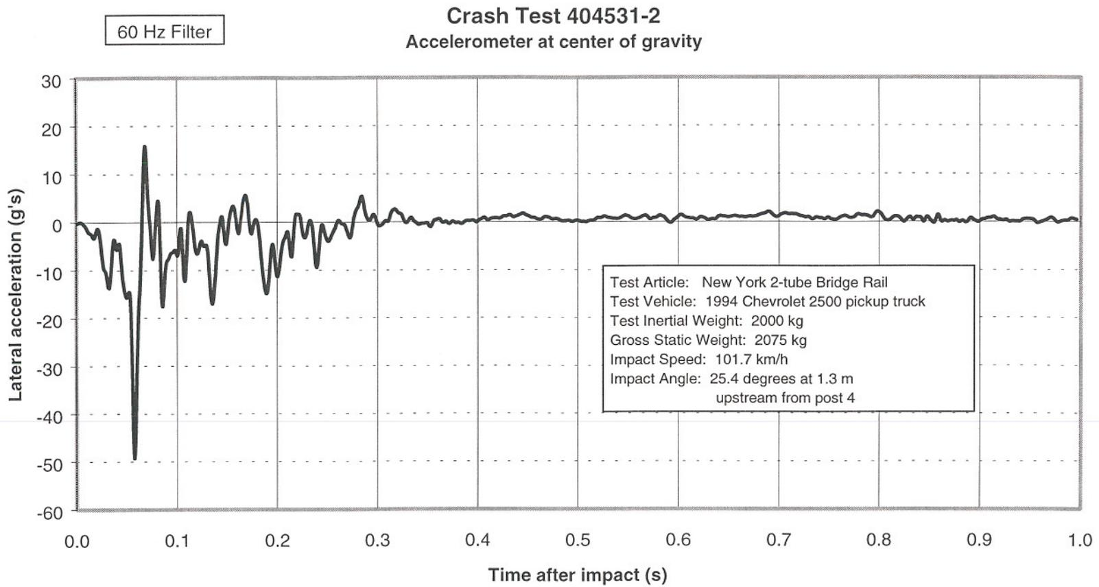
Figure 86. Vehicle lateral accelerometer trace for test 404531-2 (accelerometer located at center of gravity).
