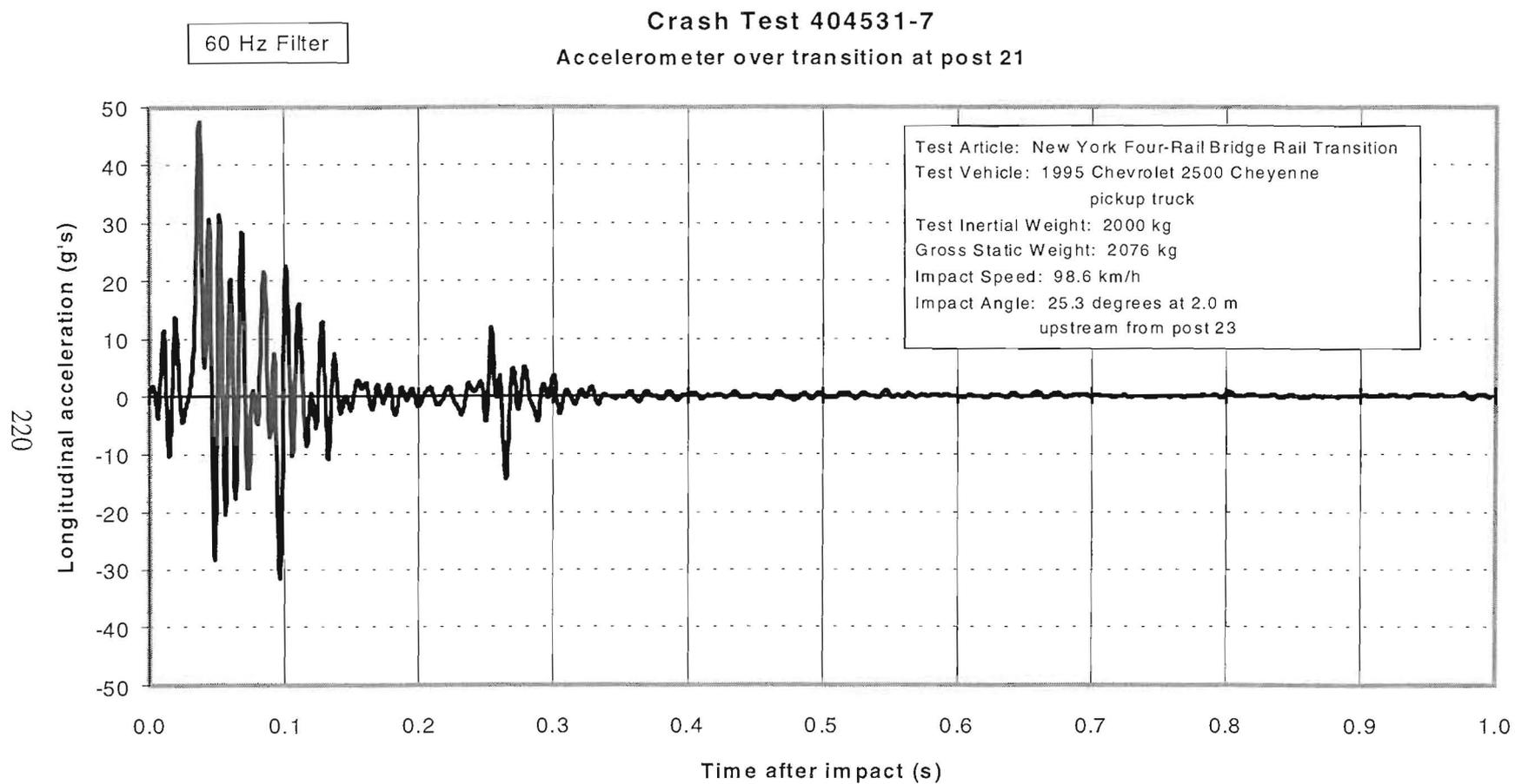
Figure 144. Transition longitudinal accelerometer trace for test 404531-7 (accelerometer located over transition at post 21).
