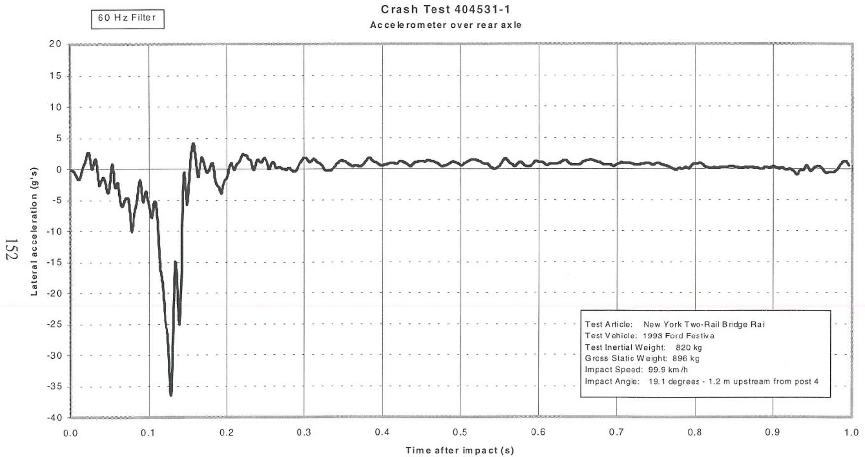
Figure 76. Vehicle lateral accelerometer trace for test 404531-1 (accelerometer located over rear axle).
