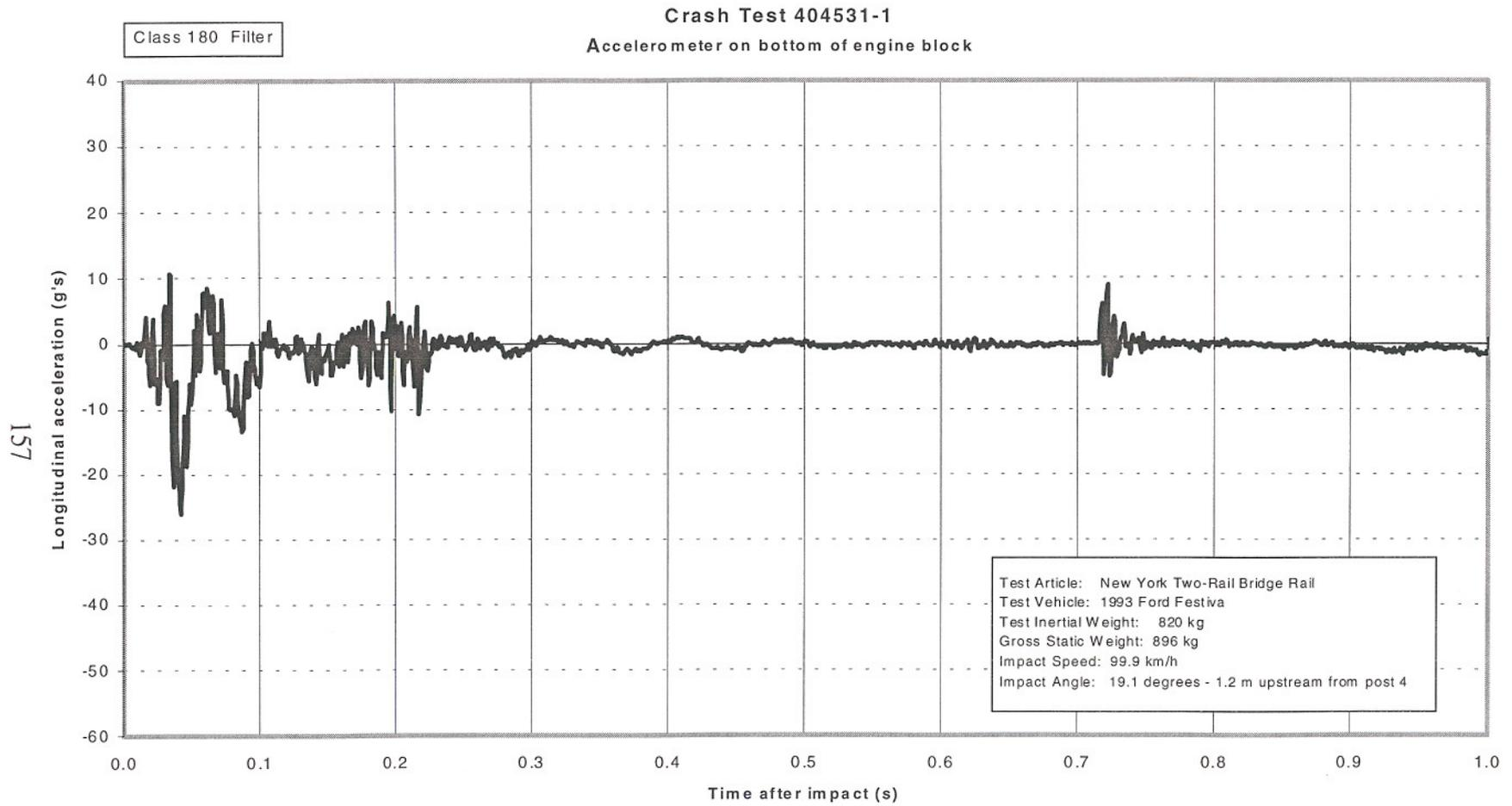
Figure 81. Vehicle longitudinal accelerometer trace for test 404531-1 (accelerometer located on bottom of engine block).
