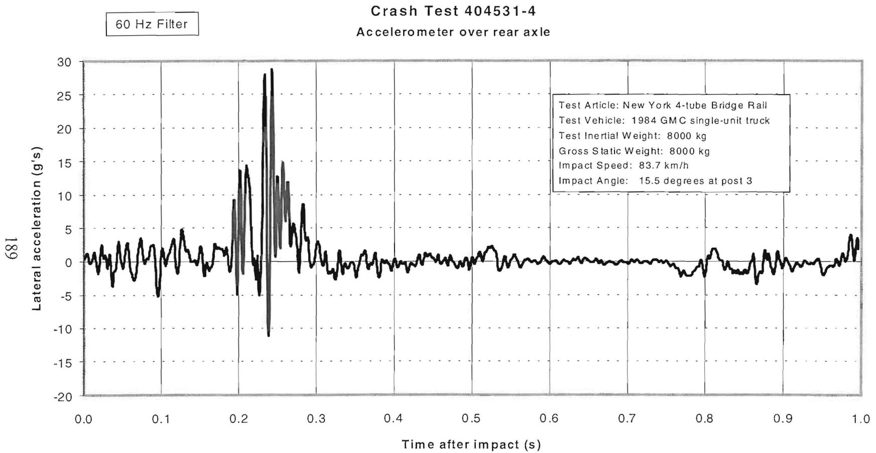
Figure 113. Vehicle lateral accelerometer trace for test 404531-4 (accelerometer located over rear axle).
