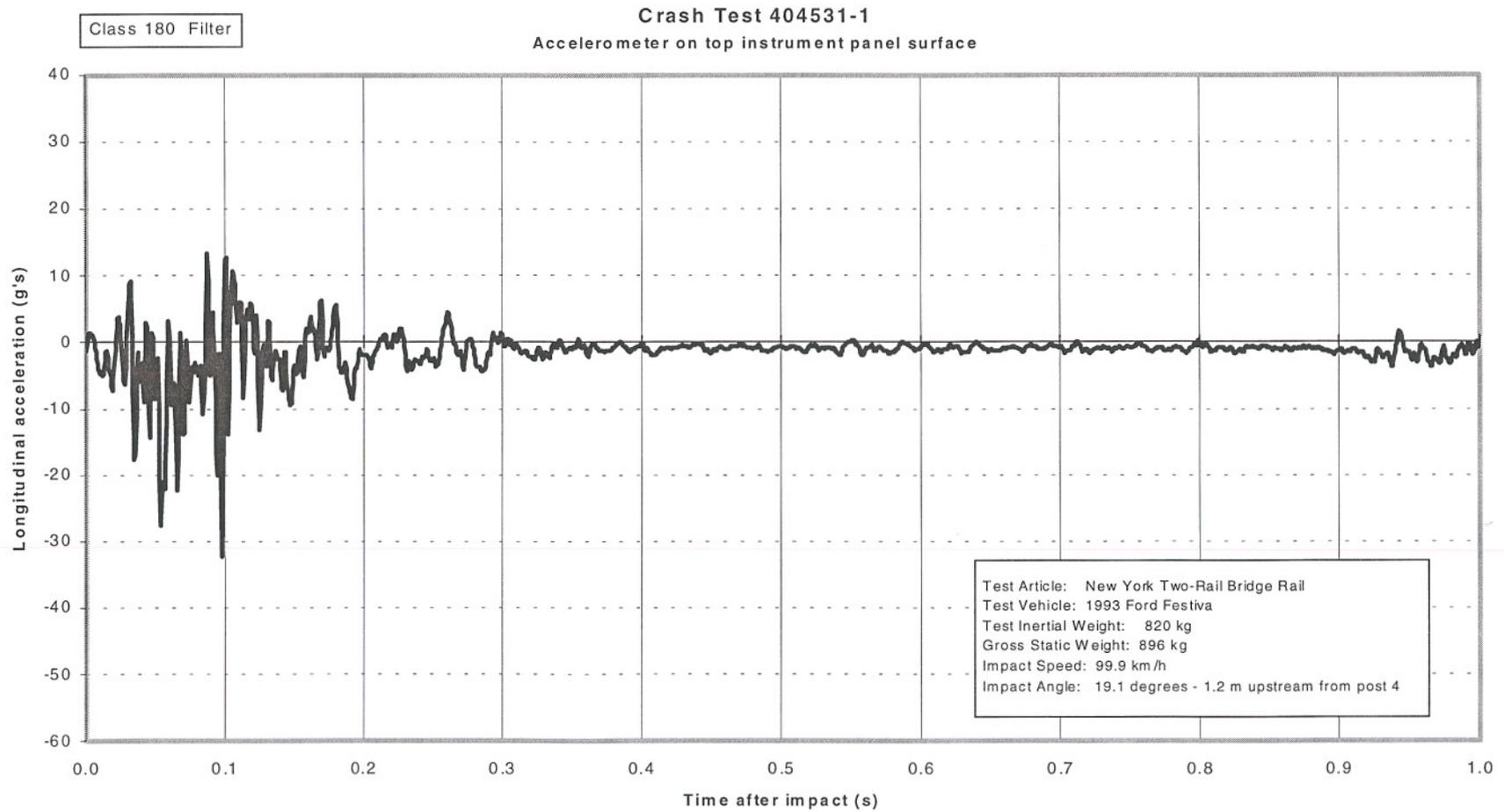
Figure 77. Vehicle longitudinal accelerometer trace for test 404531-1 (accelerometer located on top surface of instrument panel).
