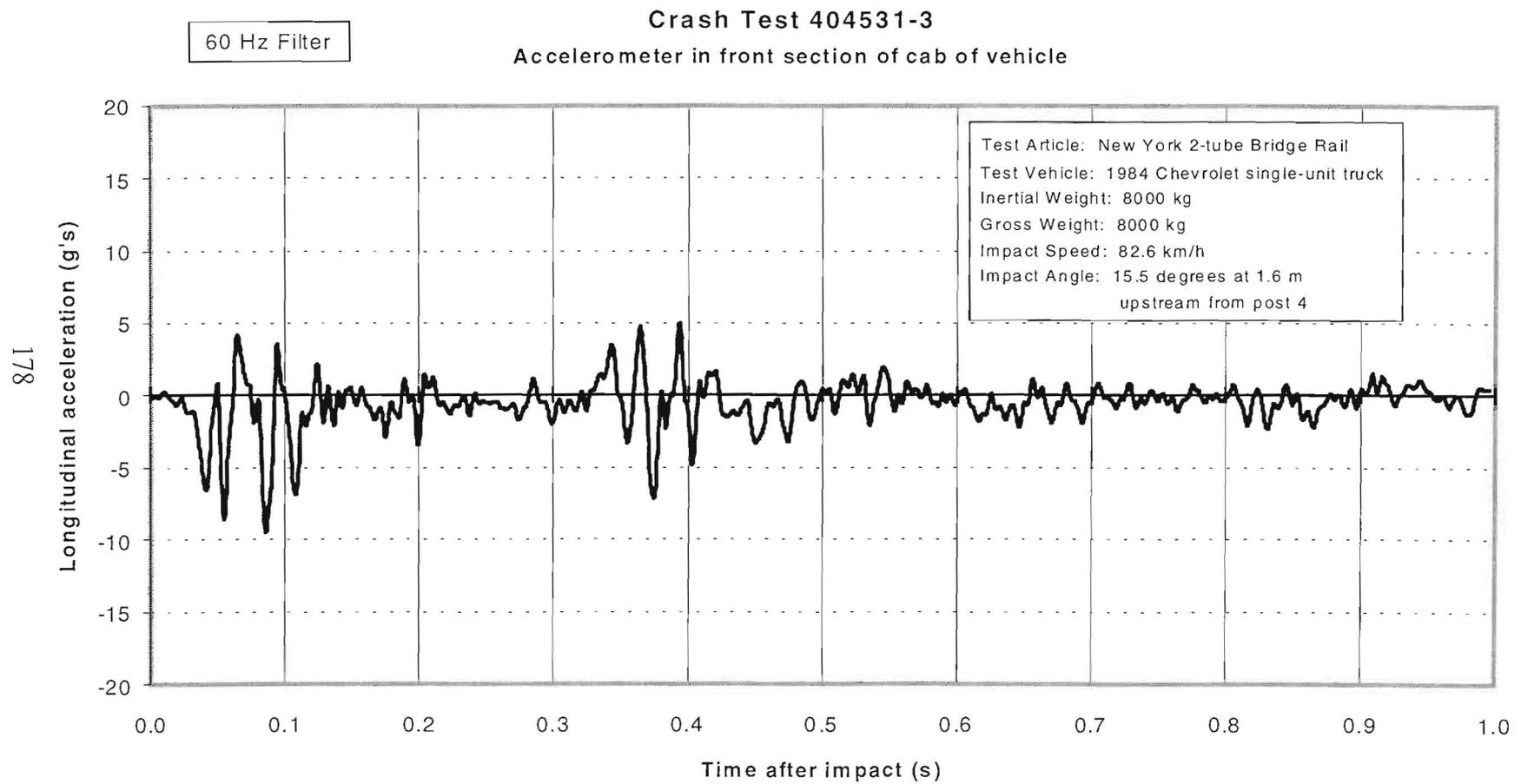
Figure 102. Vehicle longitudinal accelerometer trace for test 404531-3 (accelerometer located in front cab).
