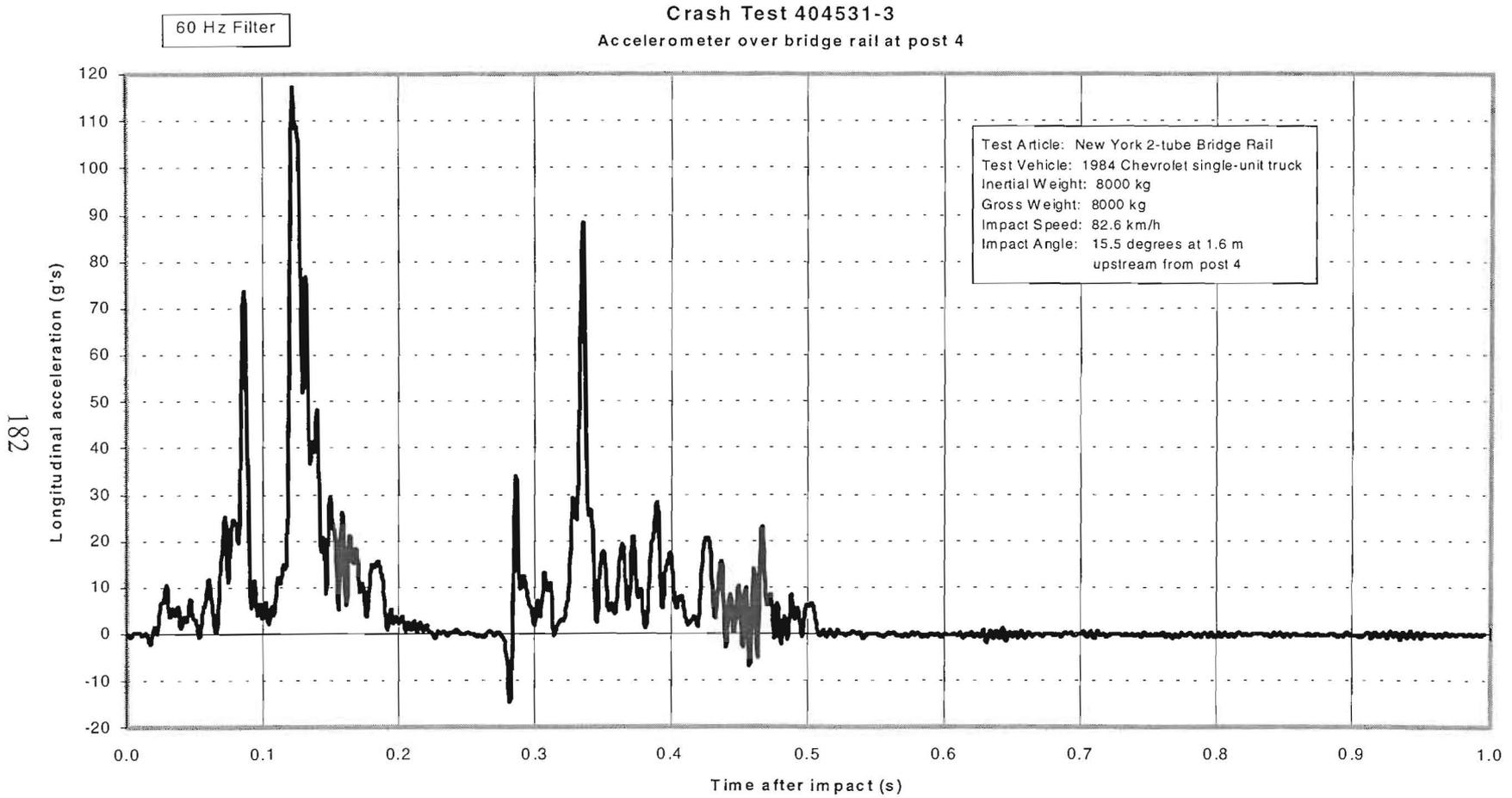
Figure 106. Vehicle longitudinal accelerometer trace for test 404531-3 (accelerometer located on post 4).
