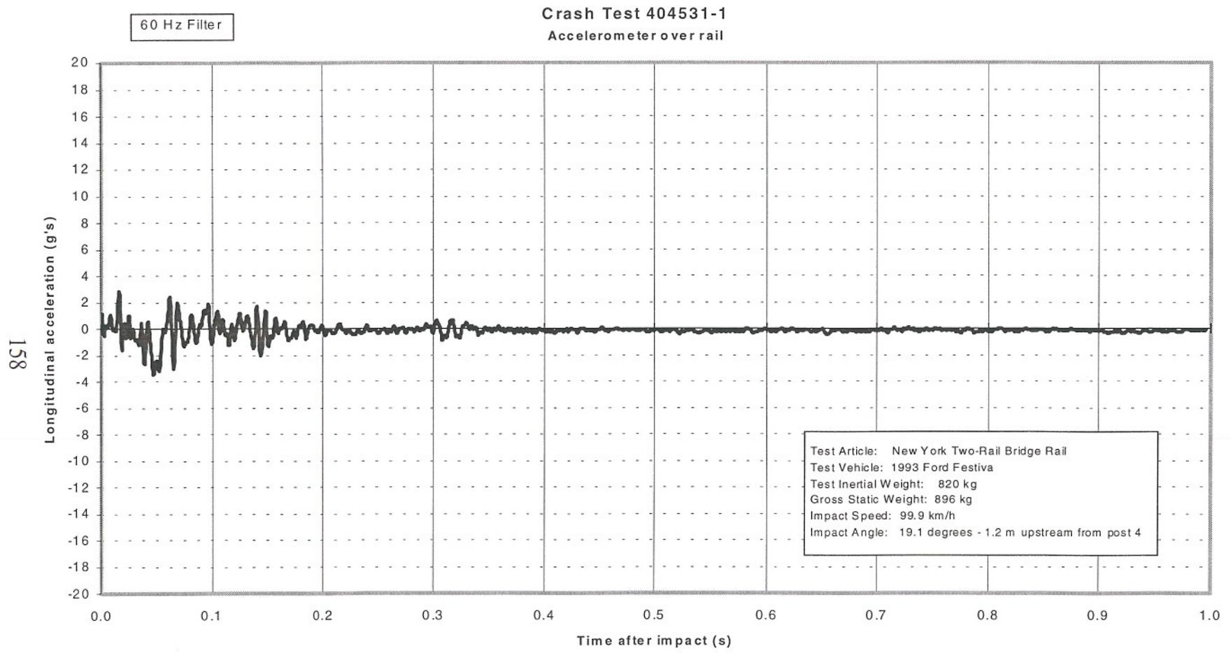
Figure 82. Bridge railing longitudinal accelerometer trace for test 404531-1 (accelerometer located over bridge railing at post 4).
