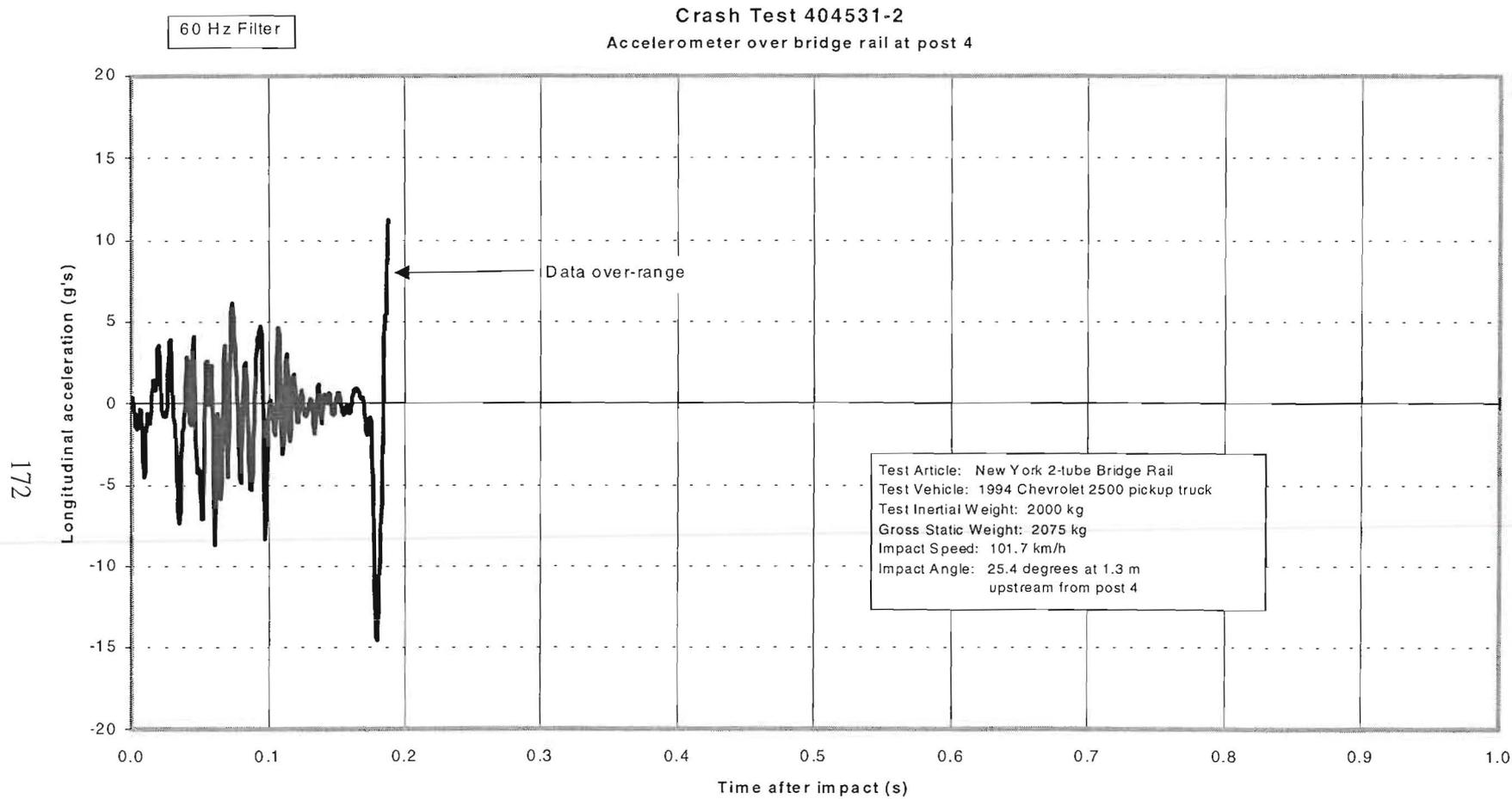
Figure 96. Bridge railing longitudinal accelerometer trace for test 404531-2 (accelerometer located over bridge railing at post 4).
