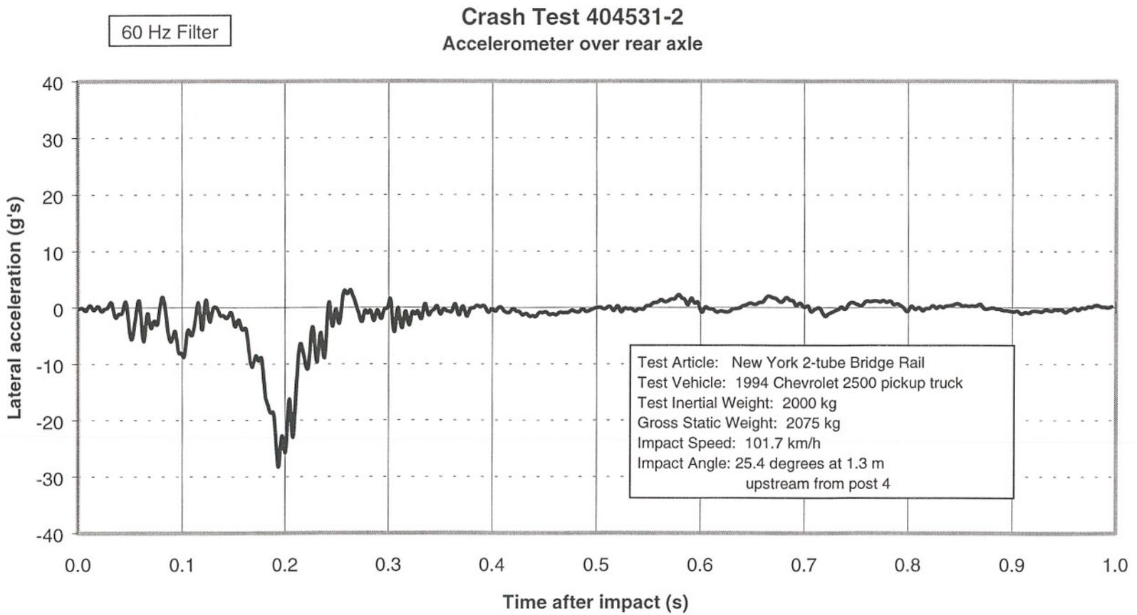
Figure 89. Vehicle lateral accelerometer trace for test 404531-2 (accelerometer located over rear axle).
