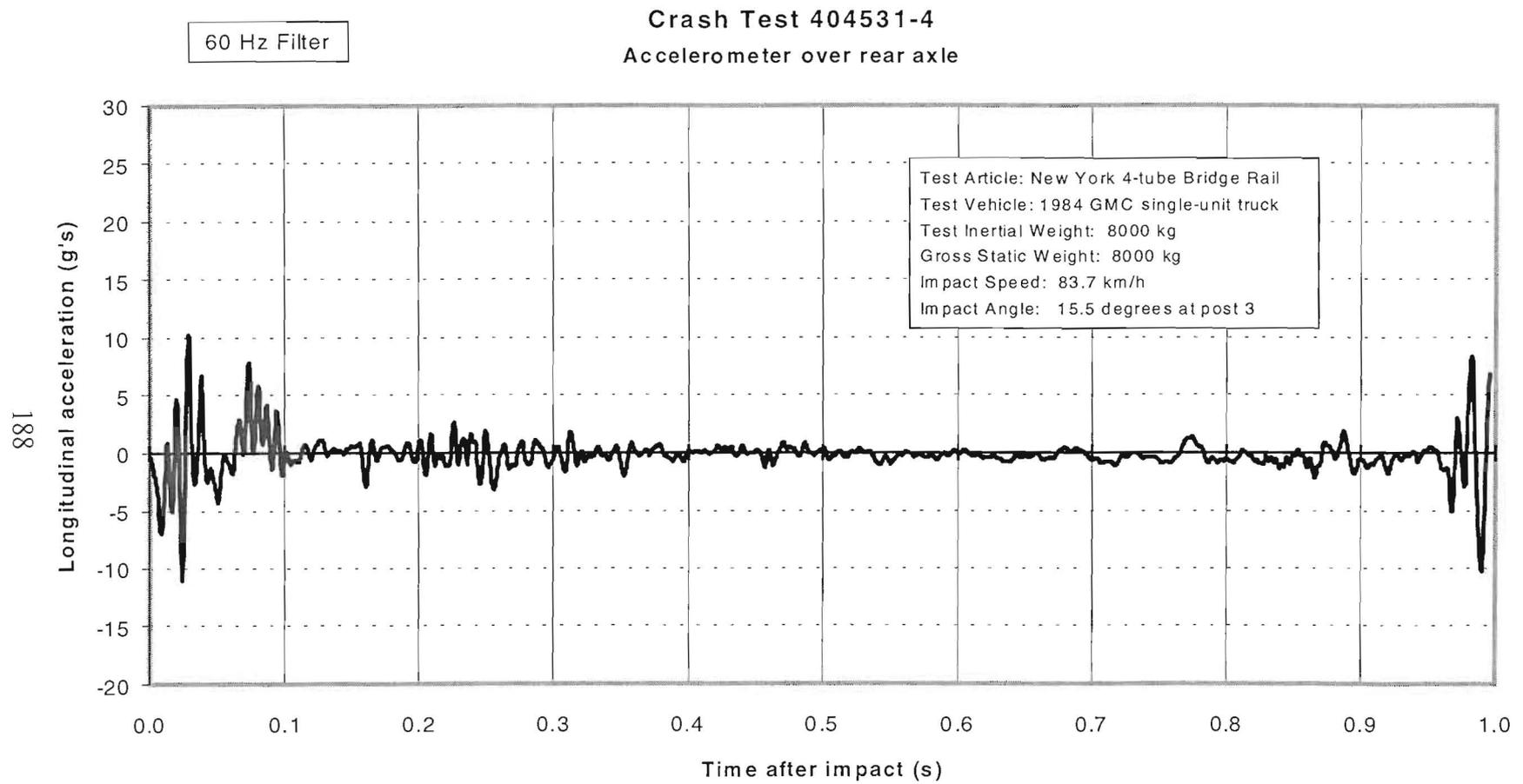
Figure 112. Vehicle longitudinal accelerometer trace for test 404531-4 (accelerometer located over rear axle).
