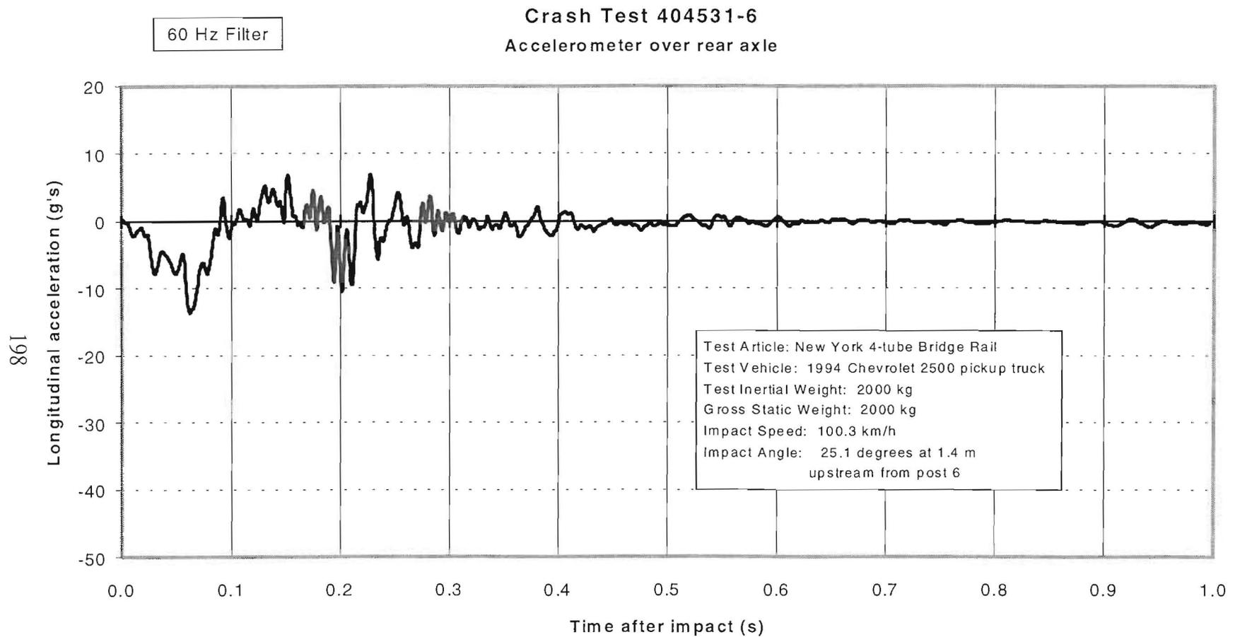
Figure 122. Vehicle longitudinal accelerometer trace for test 404531-6 (accelerometer located over rear axle).
