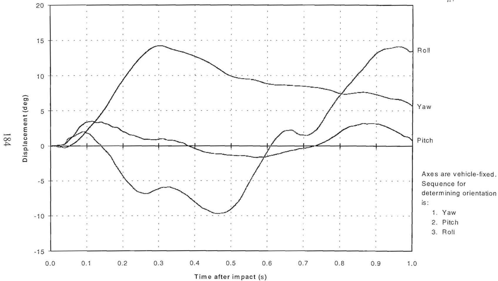
Figure 108. Vehicular angular displacements for test 404531-4.
