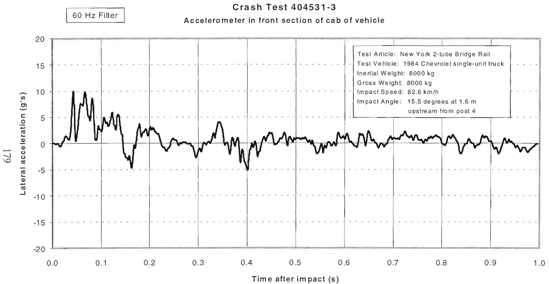
Figure 103. Vehicle lateral accelerometer trace for test 404531-3 (accelerometer located in front cab).
