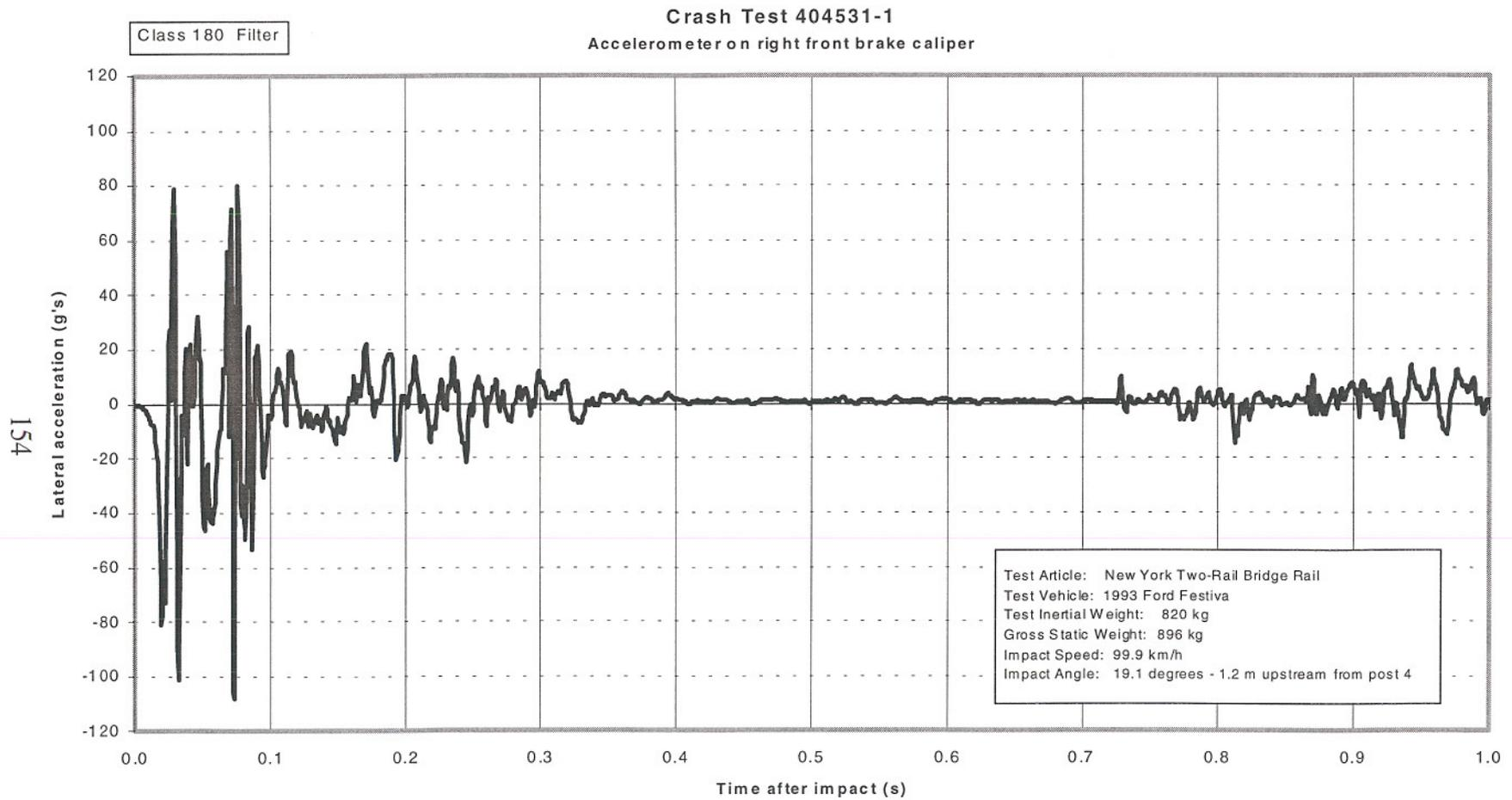
Figure 78. Vehicle lateral accelerometer trace for test 404531-1 (accelerometer located on right front brake caliper).
