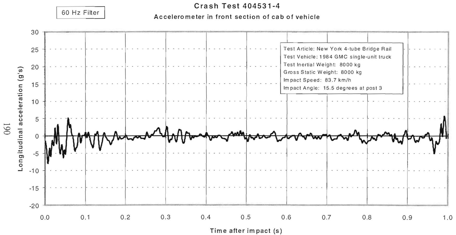
Figure 114. Vehicle longitudinal accelerometer trace for test 404531-4 (accelerometer located in cab of vehicle).
