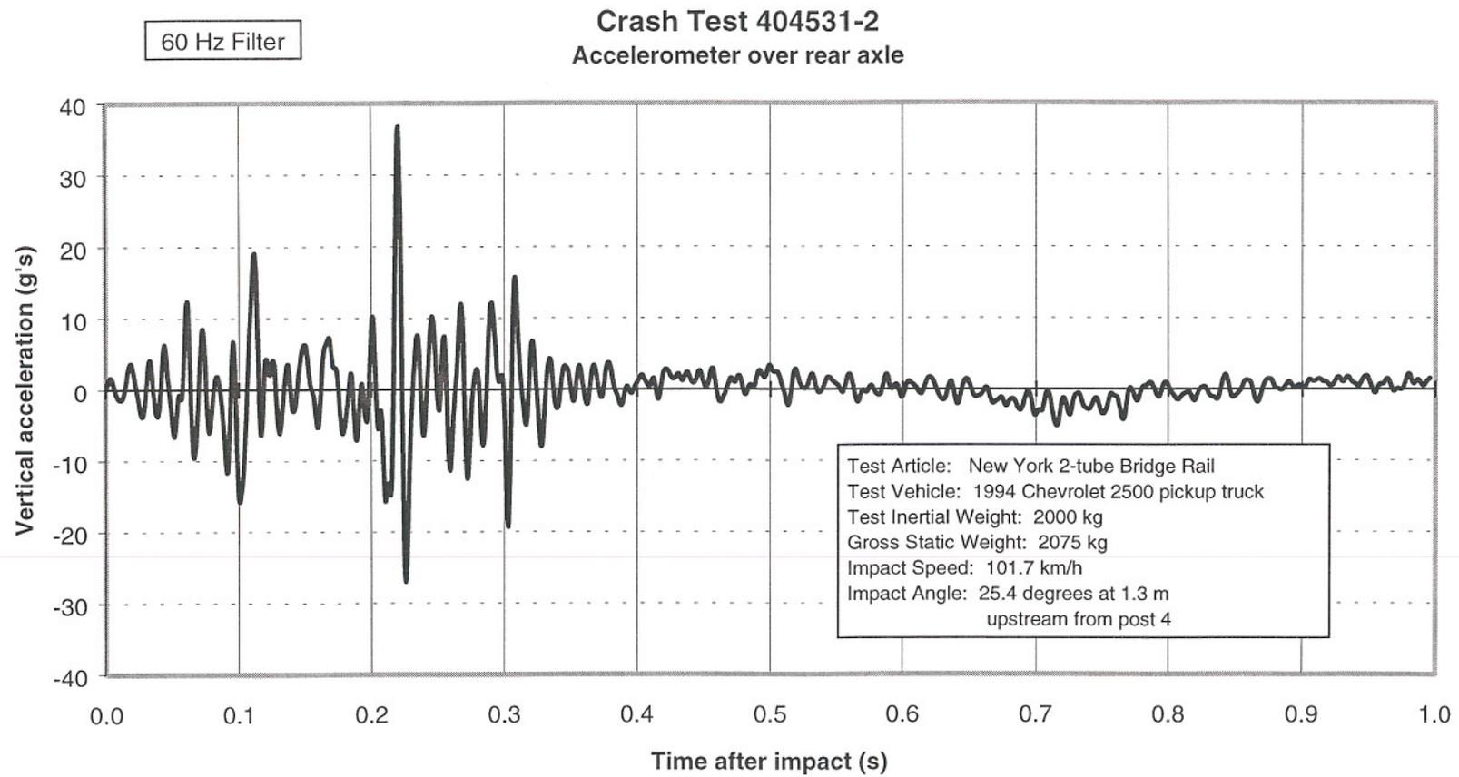
Figure 90. Vehicle vertical accelerometer trace for test 404531-2 (accelerometer located over rear axle).
