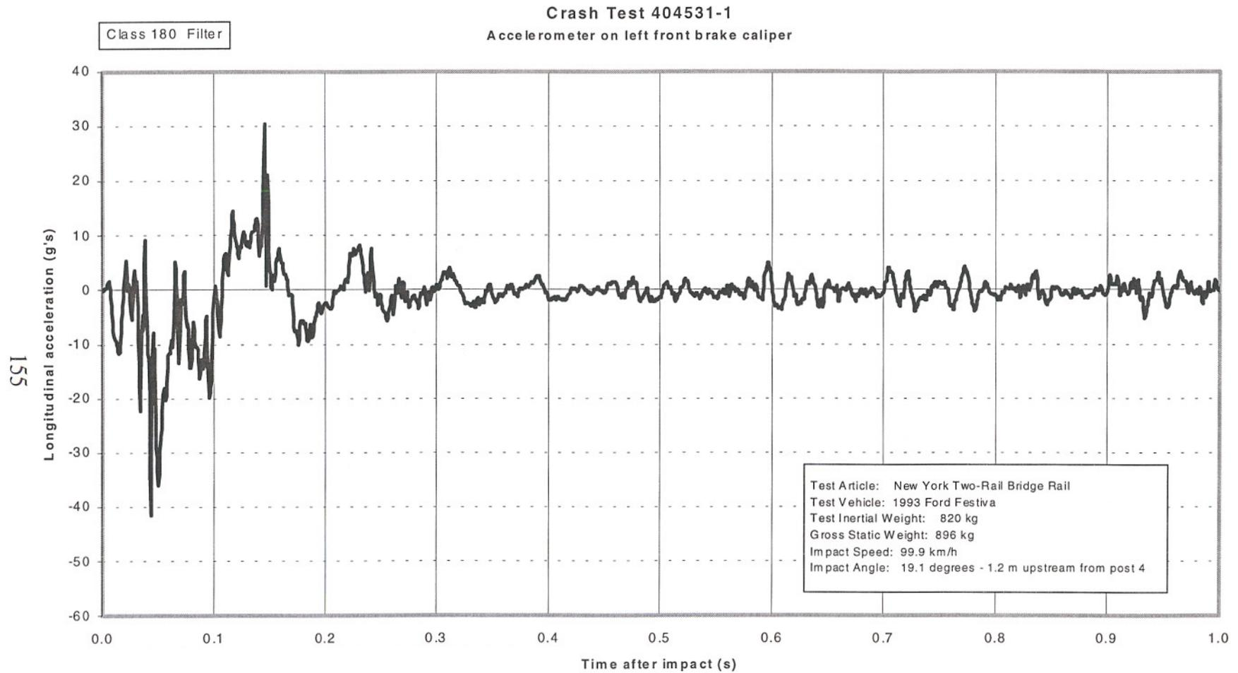
Figure 79. Vehicle longitudinal accelerometer trace for test 404531-1 (accelerometer located on left front brake caliper).
