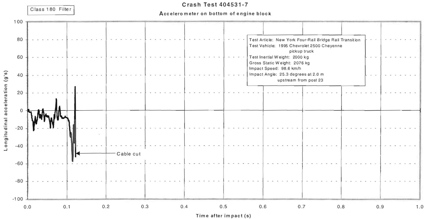
Figure 143. Vehicle longitudinal accelerometer trace for test 404531-7 (accelerometer located on bottom of engine block).
