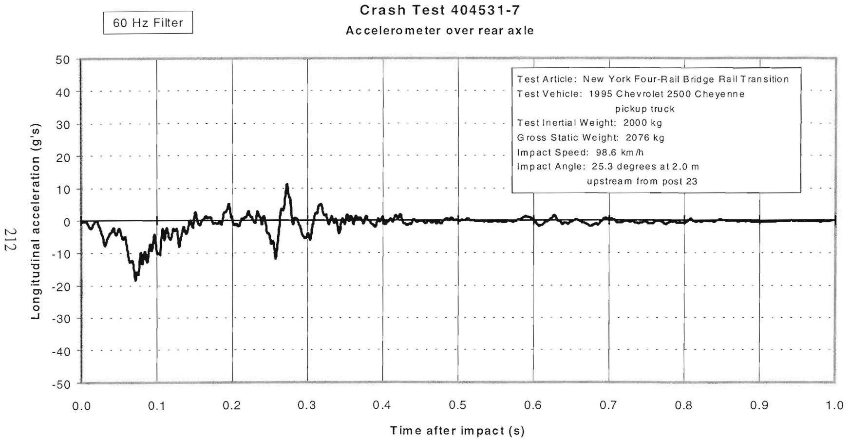
Figure 136. Vehicle longitudinal accelerometer trace for test 404531-7 (accelerometer located over rear axle).
