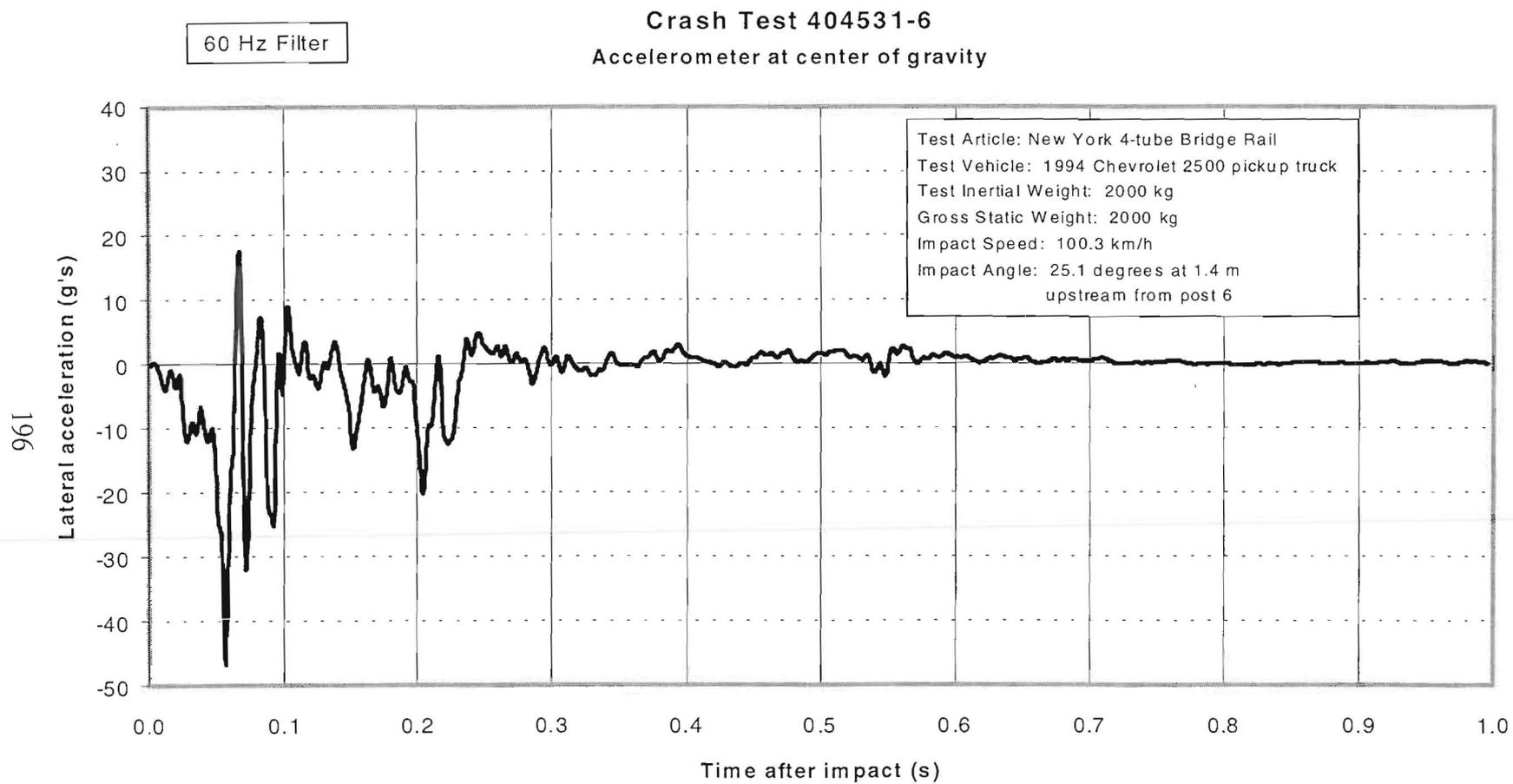
Figure 120. Vehicle lateral accelerometer trace for test 404531-6 (accelerometer located at center of gravity).
