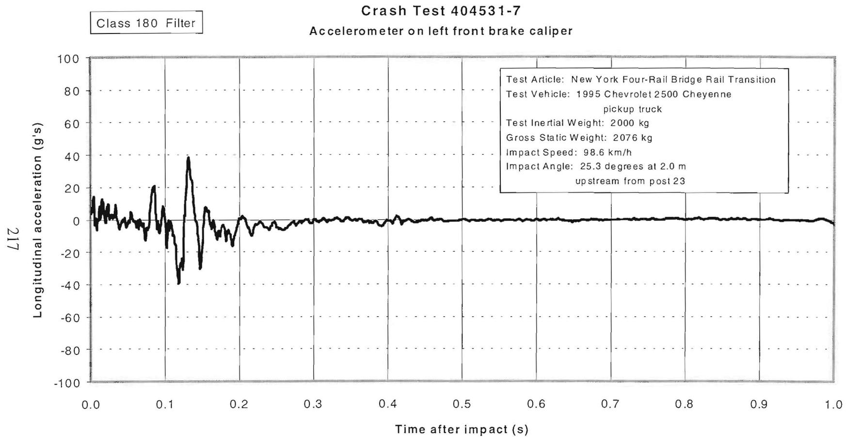
Figure 141. Vehicle longitudinal accelerometer trace for test 404531-7 (accelerometer located on left front brake caliper).
