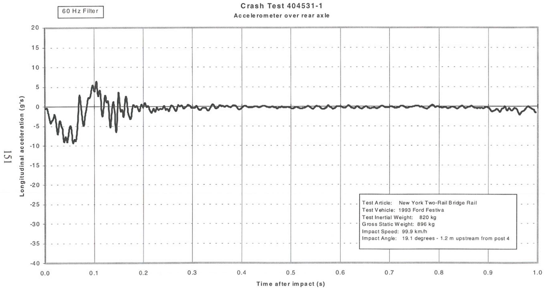
Figure 75. Vehicle longitudinal accelerometer trace for test 404531-1 (accelerometer located over rear axle).
