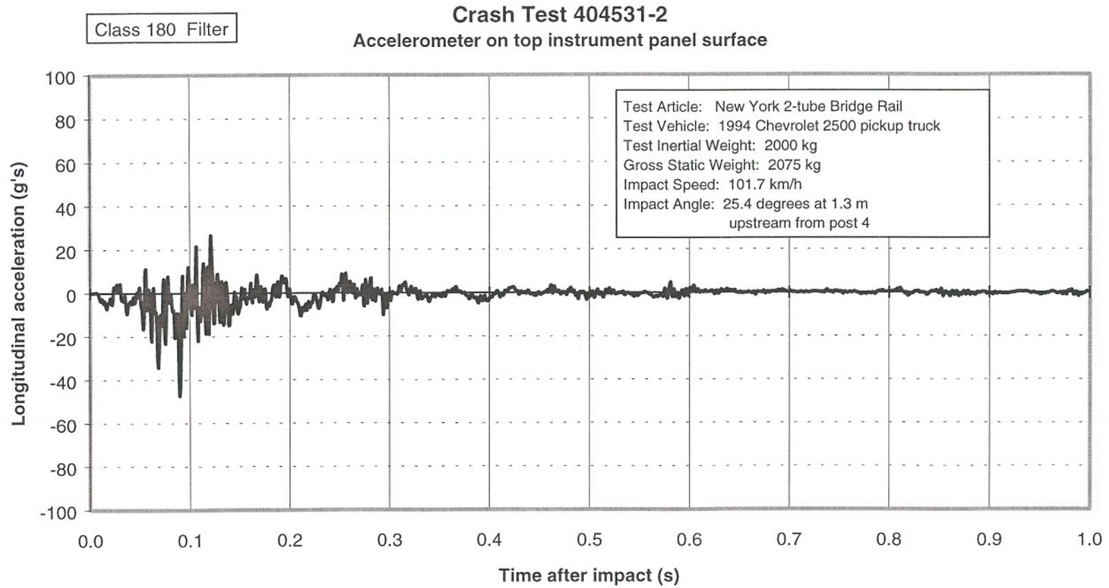
Figure 91. Vehicle longitudinal accelerometer trace for test 404531-2 (accelerometer located on top surface of instrument panel).
