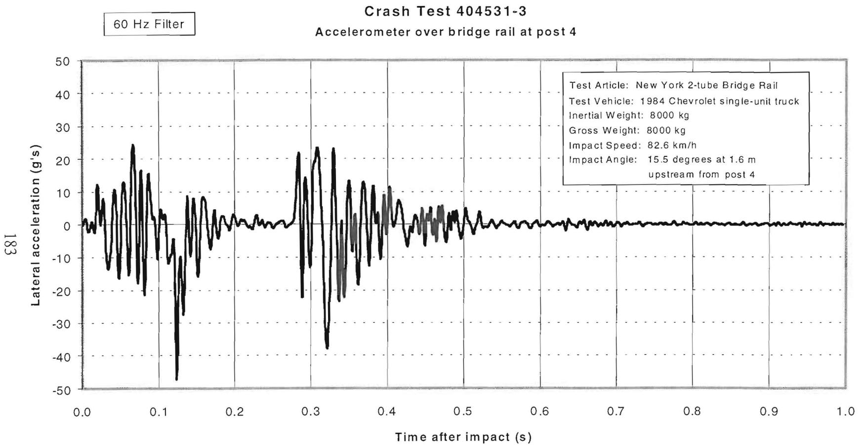
Figure 107. Vehicle lateral accelerometer trace for test 404531-3 (accelerometer located on post 4).
