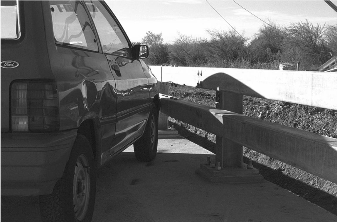
Figure 6. Vehicle/installation geometrics for test 404531-1.
