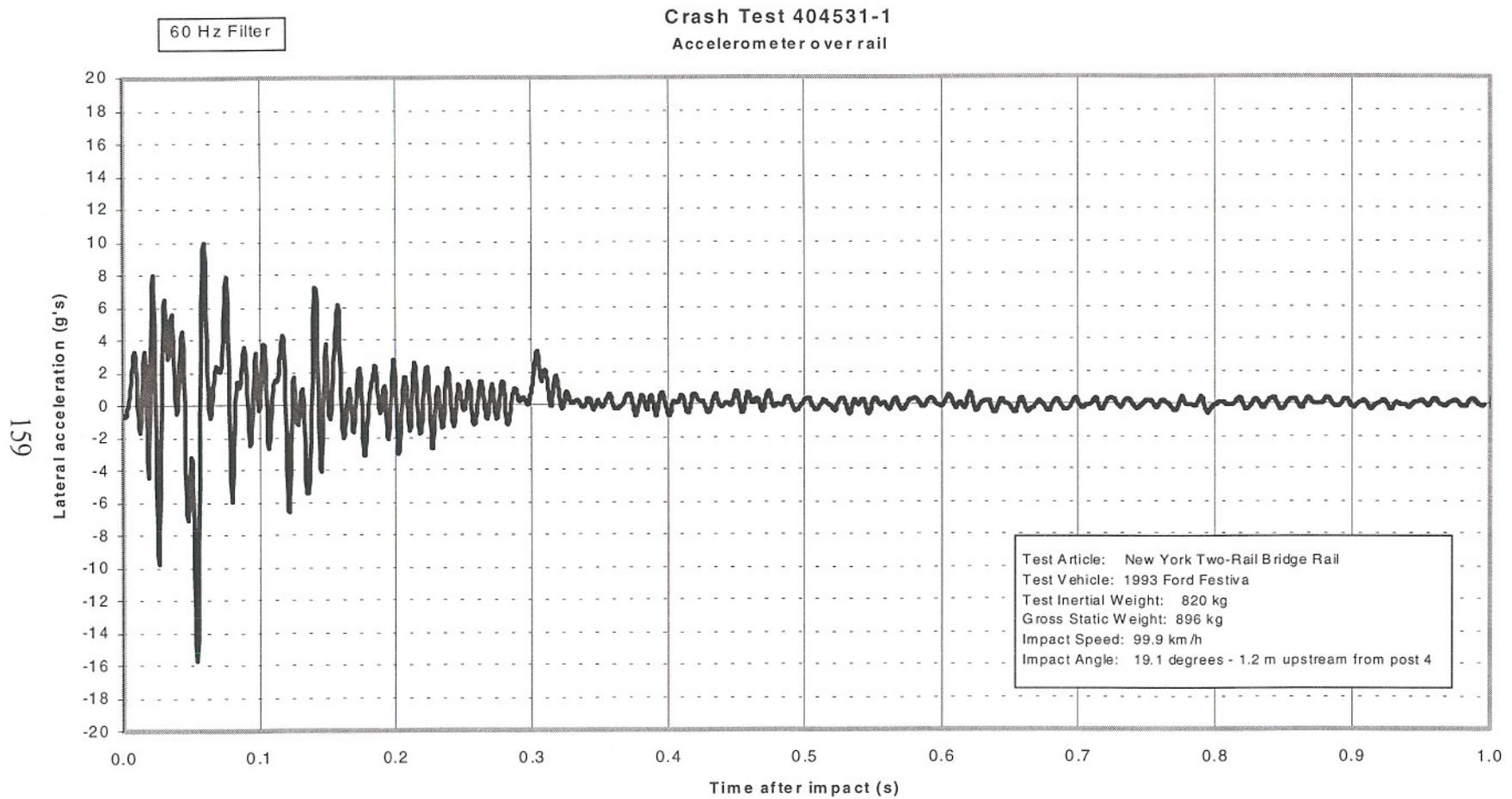
Figure 83. Bridge railing lateral accelerometer trace for test 404531-1
