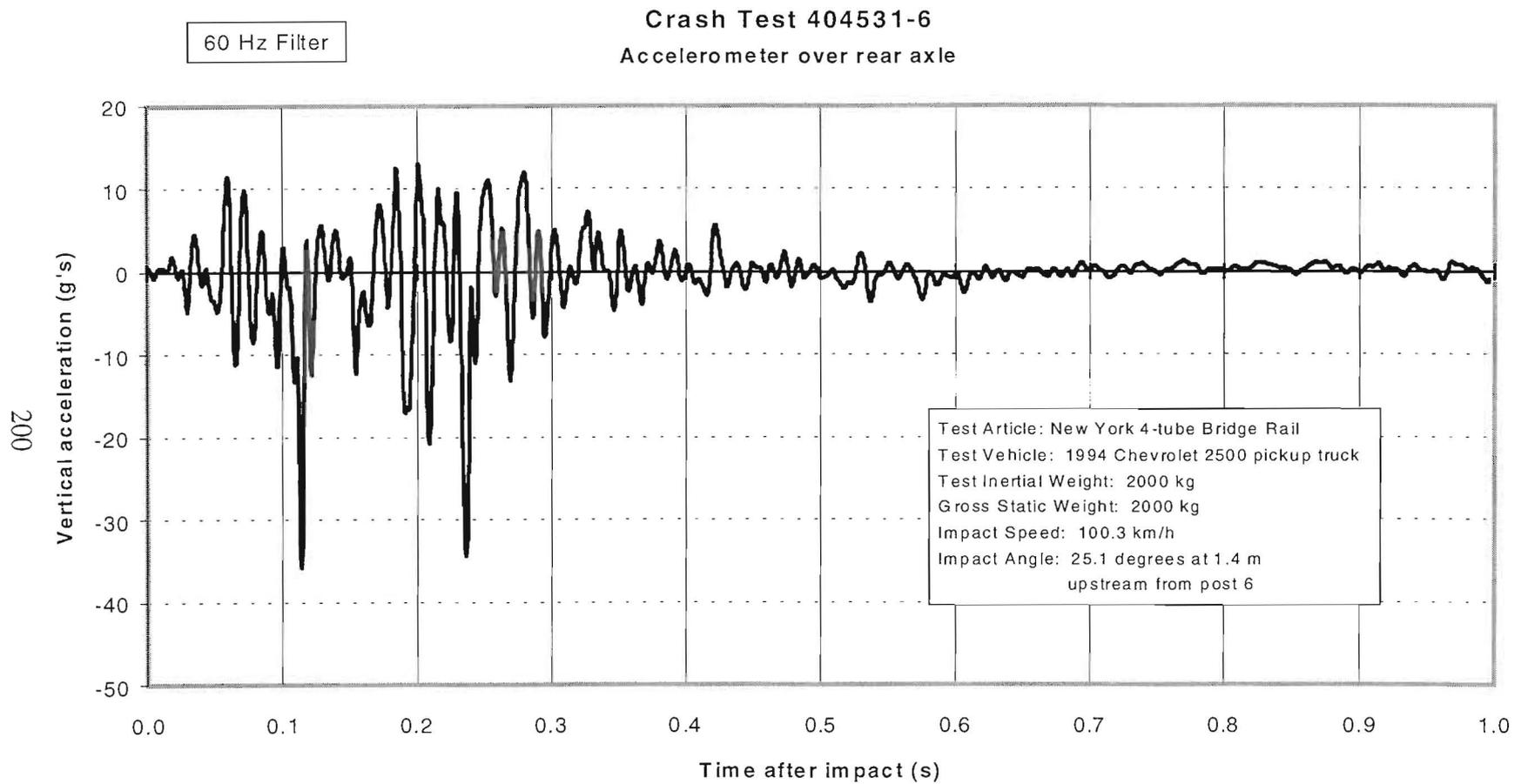
Figure 124. Vehicle vertical accelerometer trace for test 404531-6 (accelerometer located over rear axle).
