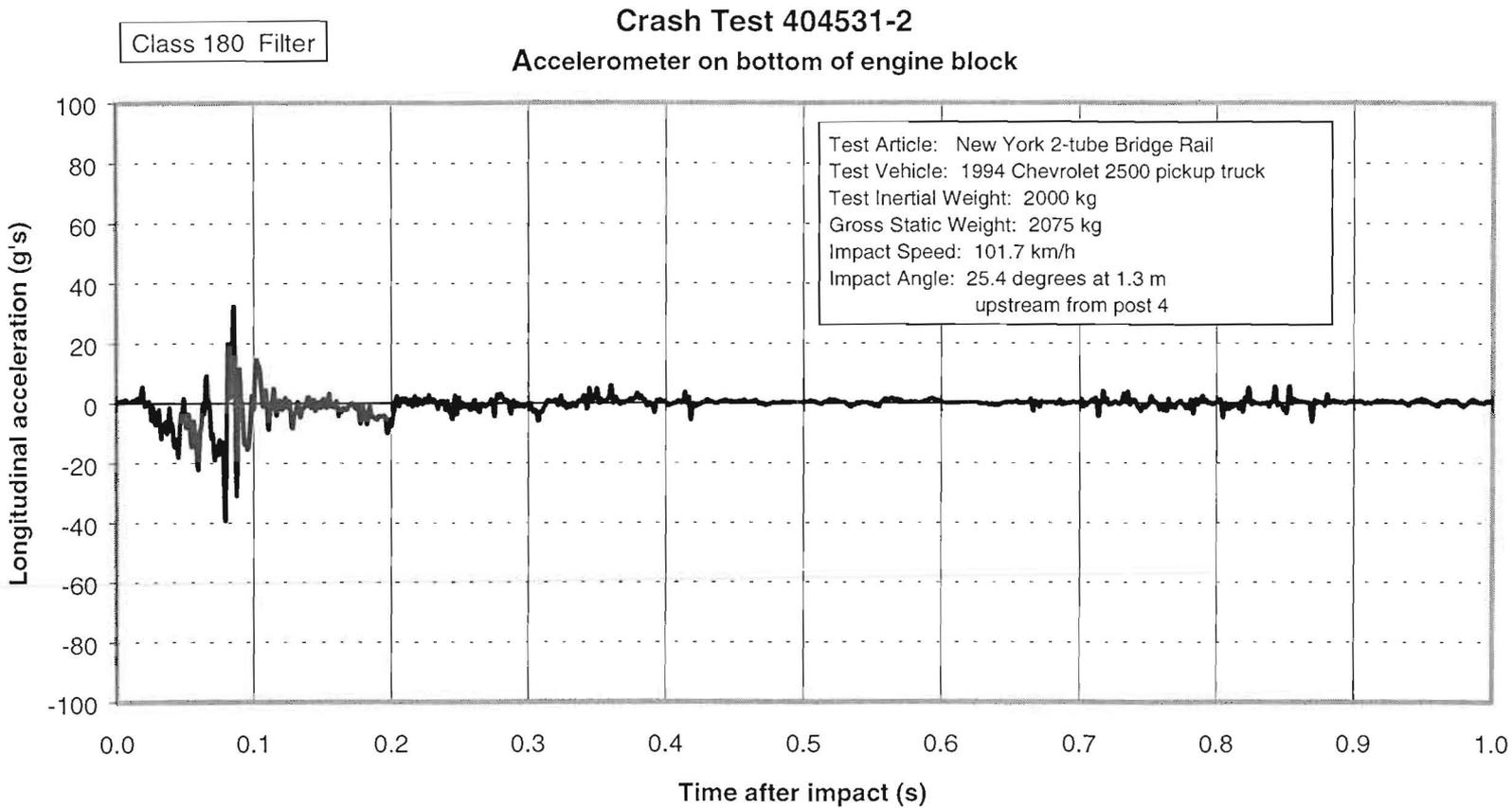
Figure 95. Vehicle longitudinal accelerometer trace for test 404531-2 (accelerometer located on bottom of engine block).
