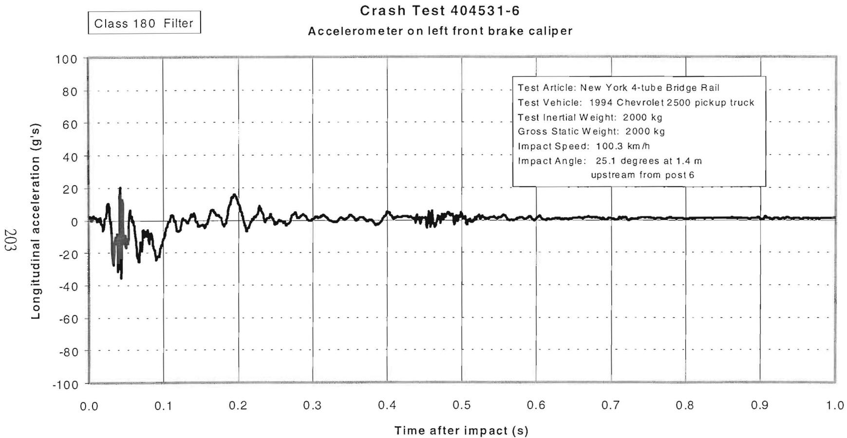
Figure 127. Vehicle longitudinal accelerometer trace for test 404531-6 (accelerometer located on left front brake caliper).
