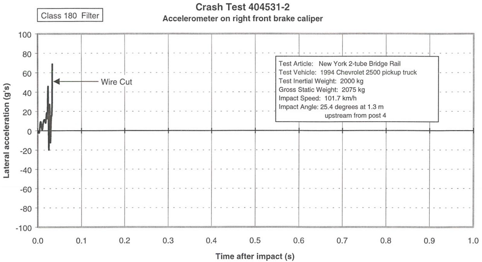
Figure 92. Vehicle lateral accelerometer trace for test 404531-2 (accelerometer located on right front brake caliper).
