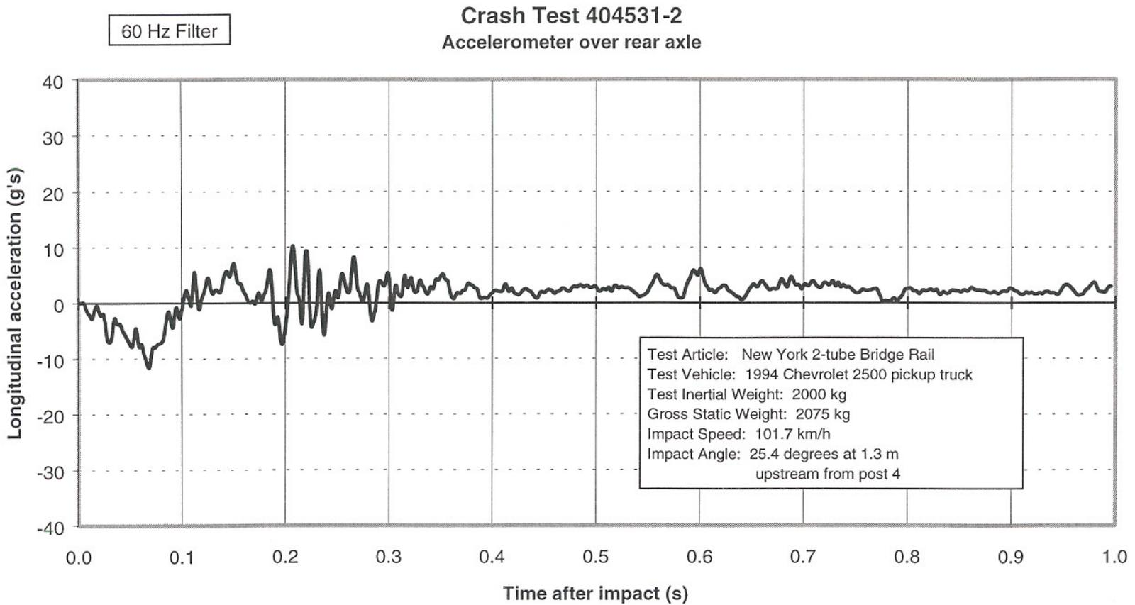
Figure 88. Vehicle longitudinal accelerometer trace for test 404531-2 (accelerometer located over rear axle).
