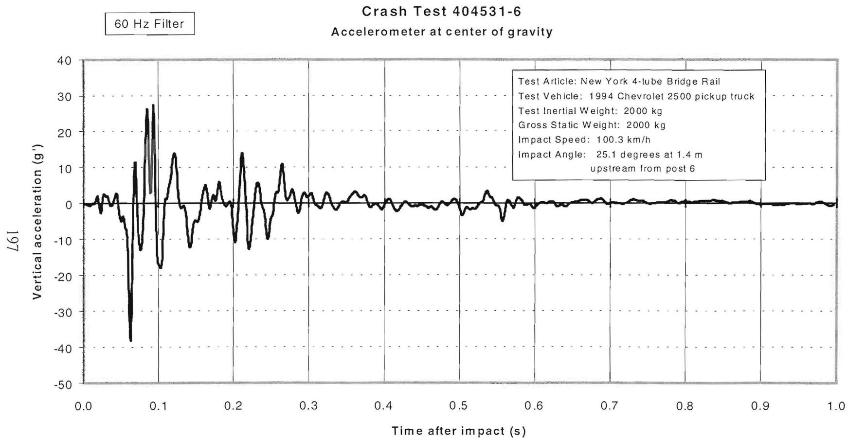
Figure 121. Vehicle vertical accelerometer trace for test 404531-6 (accelerometer located at center of gravity).
