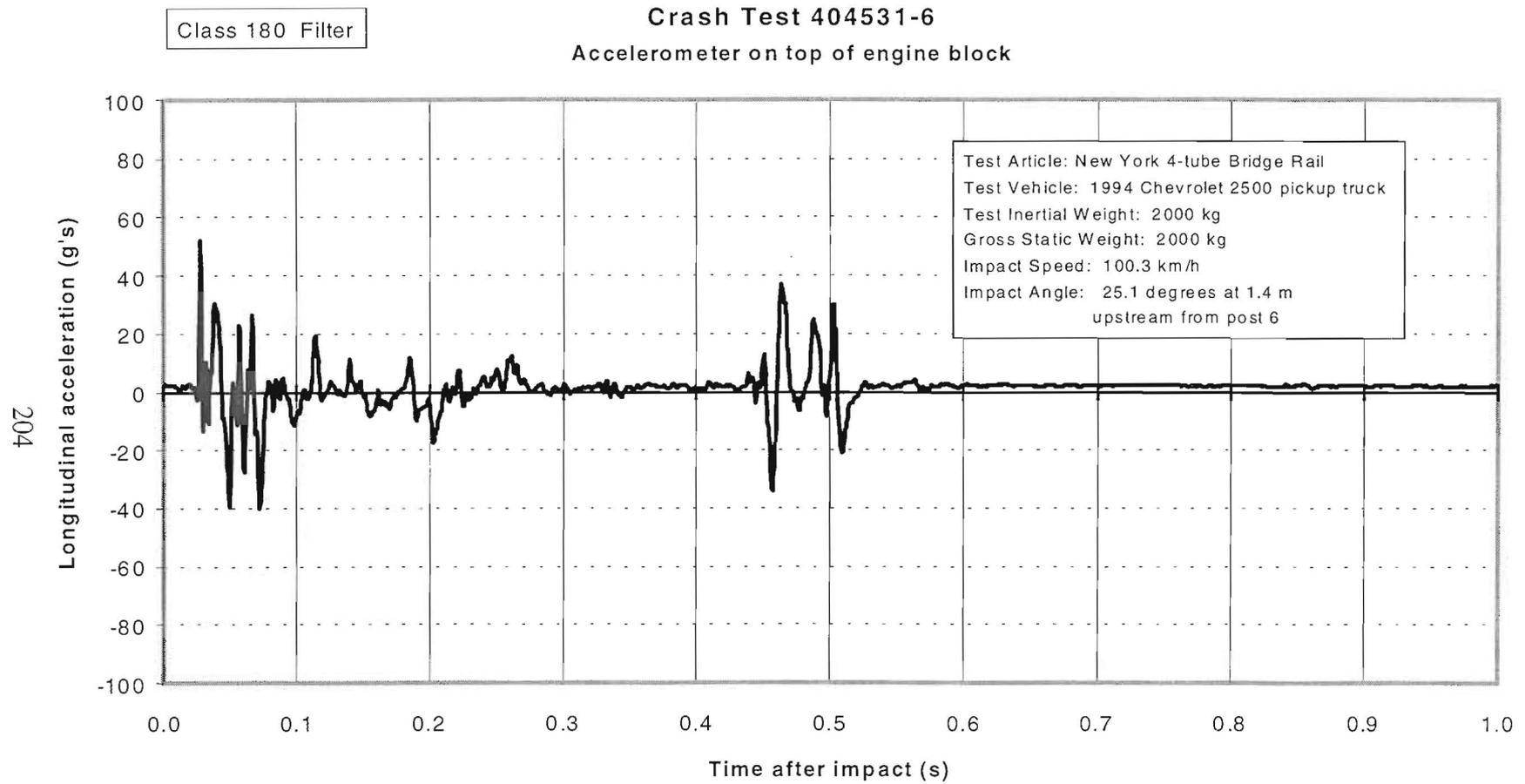
Figure 128. Vehicle longitudinal accelerometer trace for test 404531-6 (accelerometer located on top of engine block).
