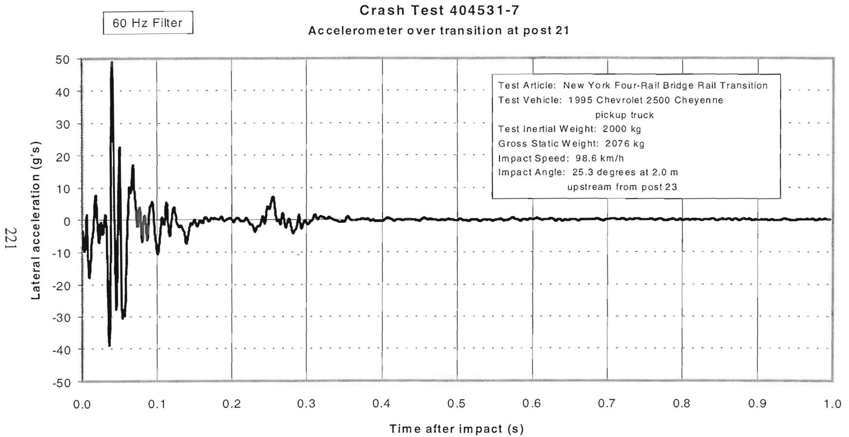
Figure 145. Transition lateral accelerometer trace for test 404531-7 (accelerometer located over transition at post 21).
