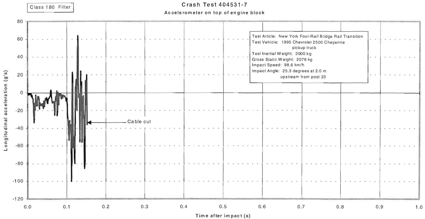
Figure 142. Vehicle longitudinal accelerometer trace for test 404531-7 (accelerometer located on top of engine block).
