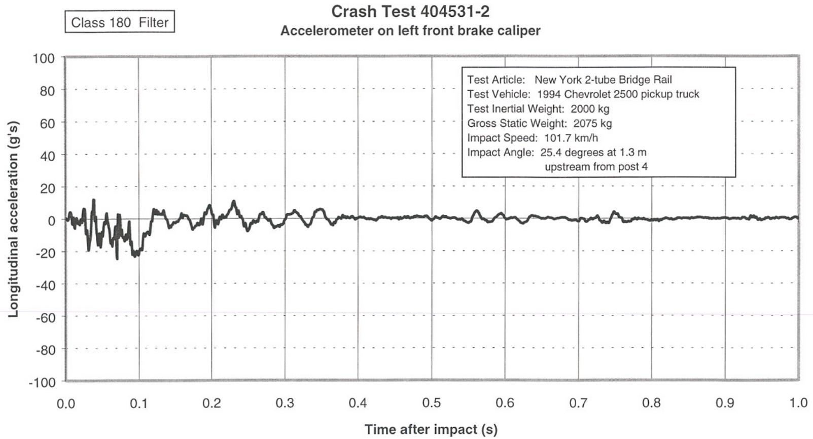
Figure 93. Vehicle longitudinal accelerometer trace for test 404531-2 (accelerometer located on left front brake caliper).
