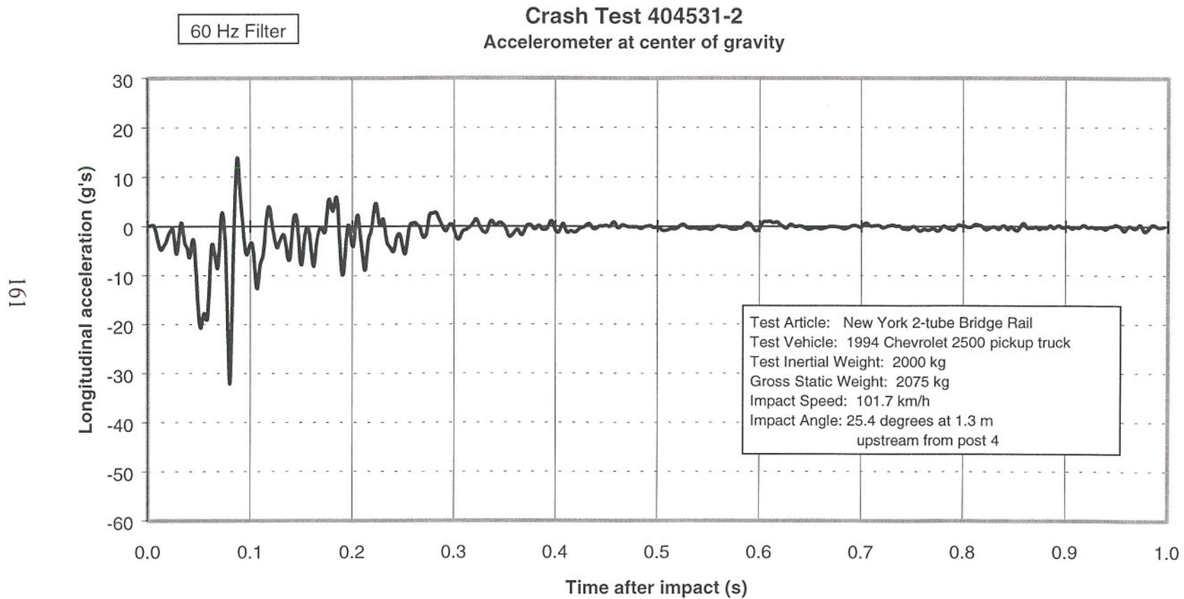
Figure 85. Vehicle longitudinal accelerometer trace for test 404531-2 (accelerometer located at center of gravity).
