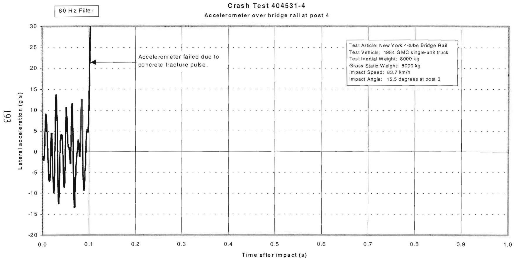
Figure 117. Bridge railing lateral accelerometer trace for test 404531-4 (accelerometer located over bridge railing at post 4).
