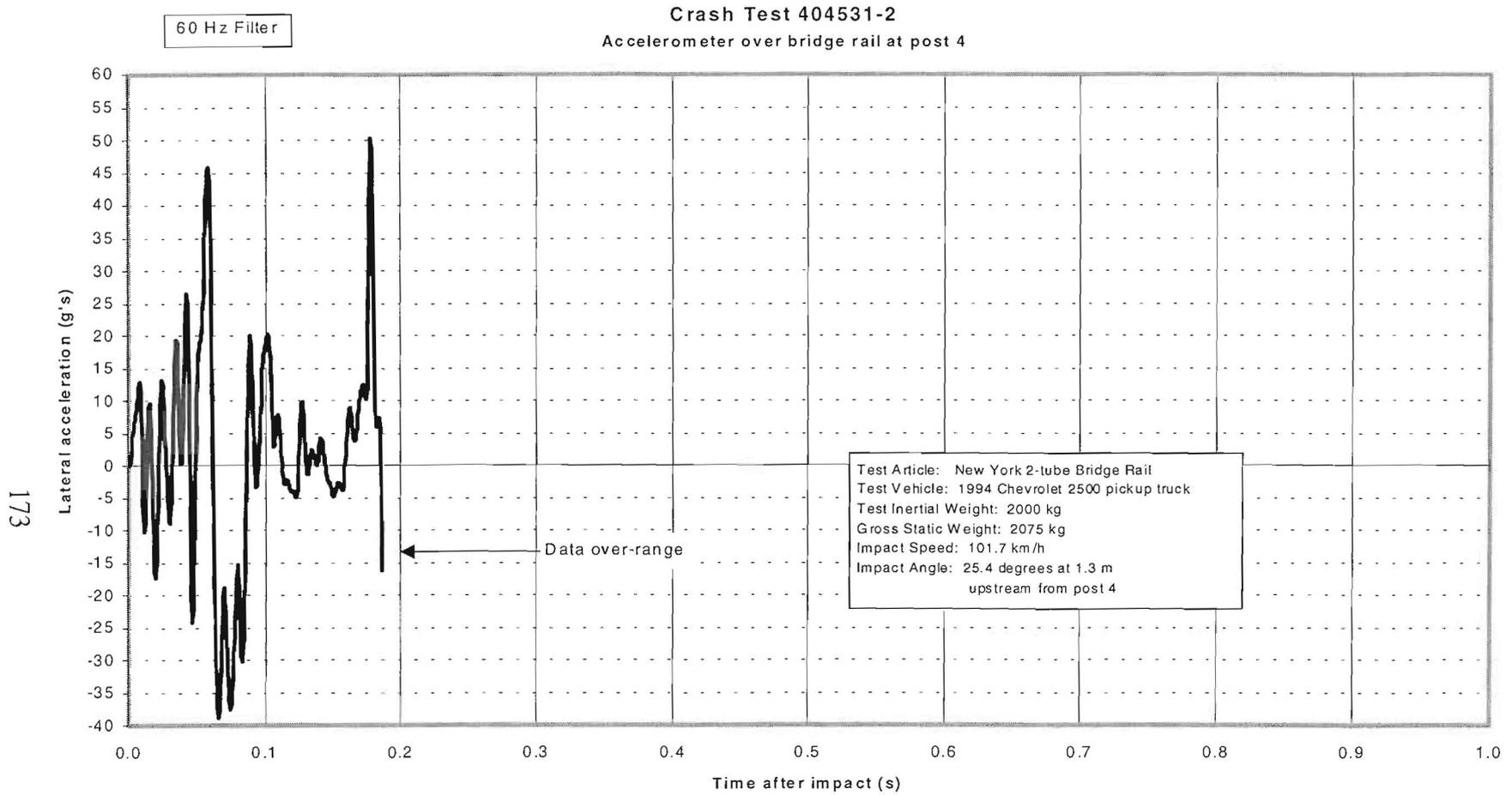
Figure 97. Bridge railing lateral accelerometer trace for test 404531-2 (accelerometer located over bridge railing at post 4).
