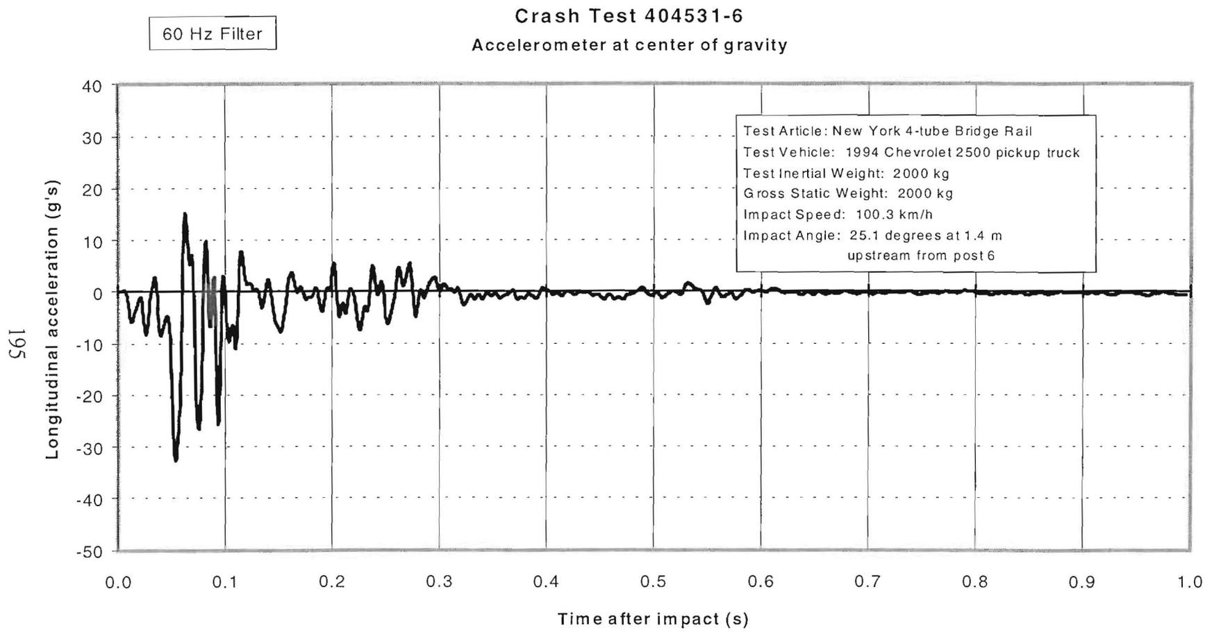
Figure 119. Vehicle longitudinal accelerometer trace for test 404531-6 (accelerometer located at center of gravity).
