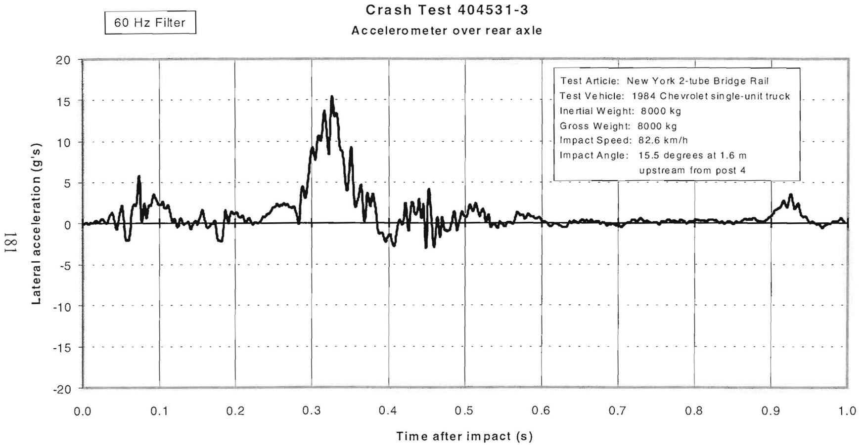
Figure 105. Vehicle lateral accelerometer trace for test 404531-3 (accelerometer located in rear of box-van).
