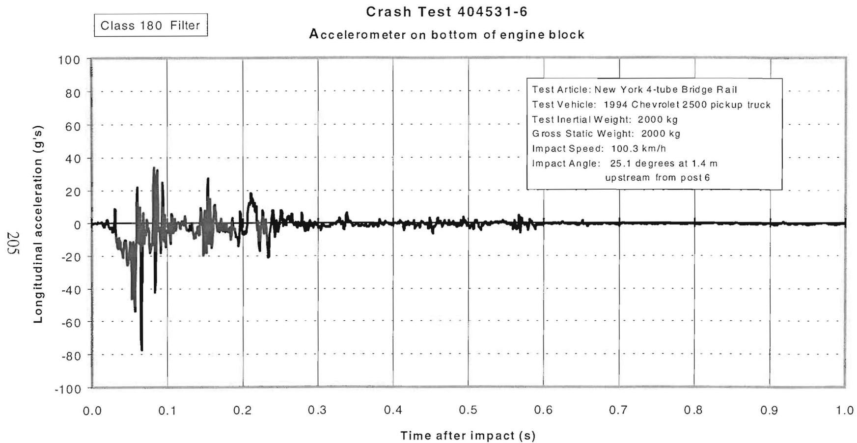
Figure 129. Vehicle longitudinal accelerometer trace for test 404531-6 (accelerometer located on bottom of engine block).
