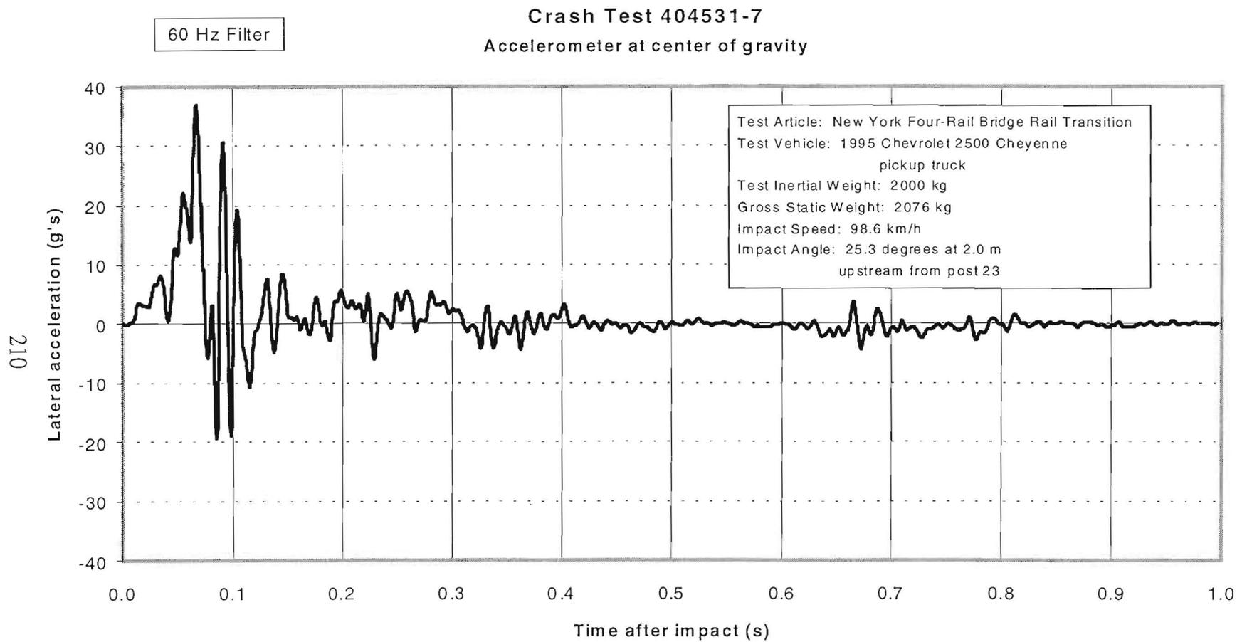
Figure 134. Vehicle lateral accelerometer trace for test 404531-7 (accelerometer located at center of gravity).
