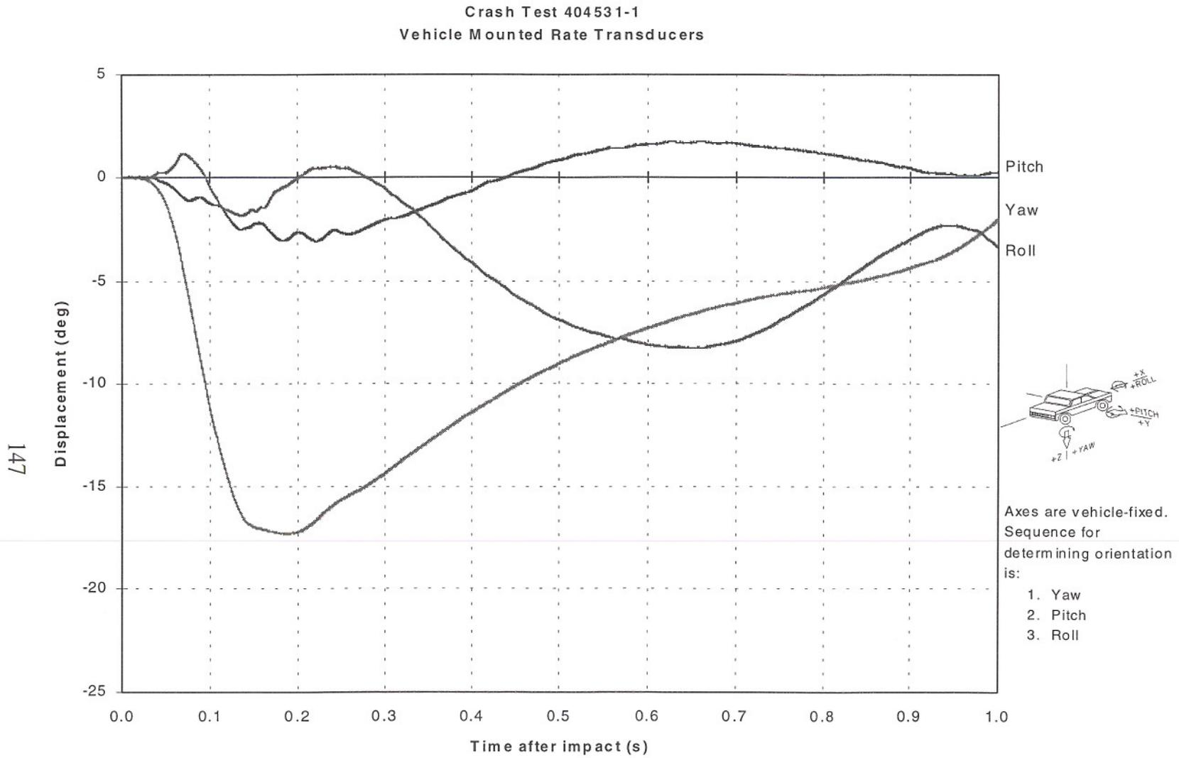
Figure 71. Vehicular angular displacements for test 404531-1.
