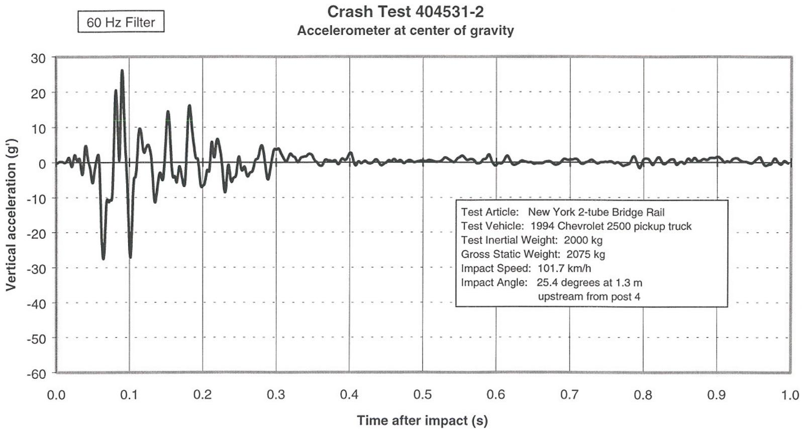
Figure 87. Vehicle vertical accelerometer trace for test 404531-2 (accelerometer located at center of gravity).
