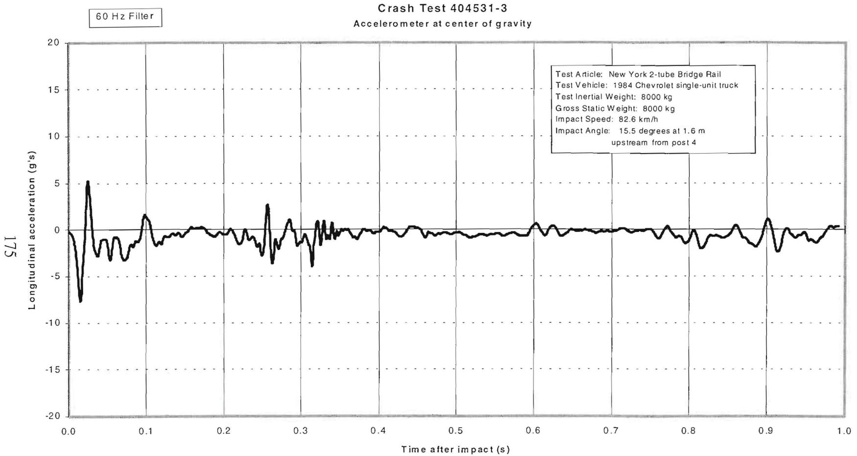
Figure 99. Vehicle longitudinal accelerometer trace for test 404531-3 (accelerometer located at center of gravity).
