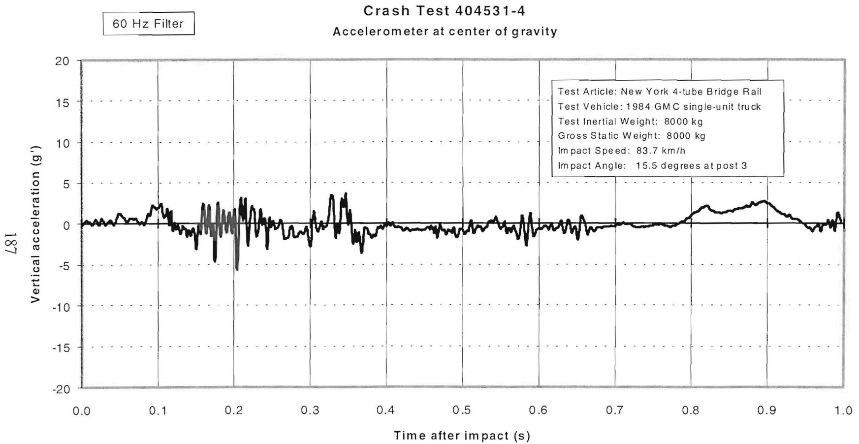
Figure 111. Vehicle vertical accelerometer trace for test 404531-4 (accelerometer located at center of gravity).
