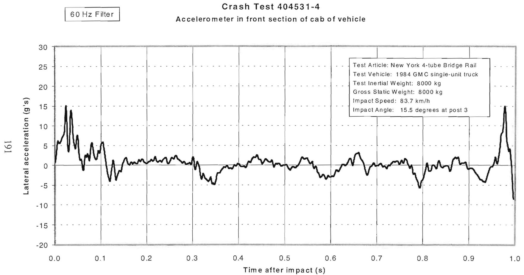
Figure 115. Vehicle lateral accelerometer trace for test 404531-4 (accelerometer located in cab of vehicle).
