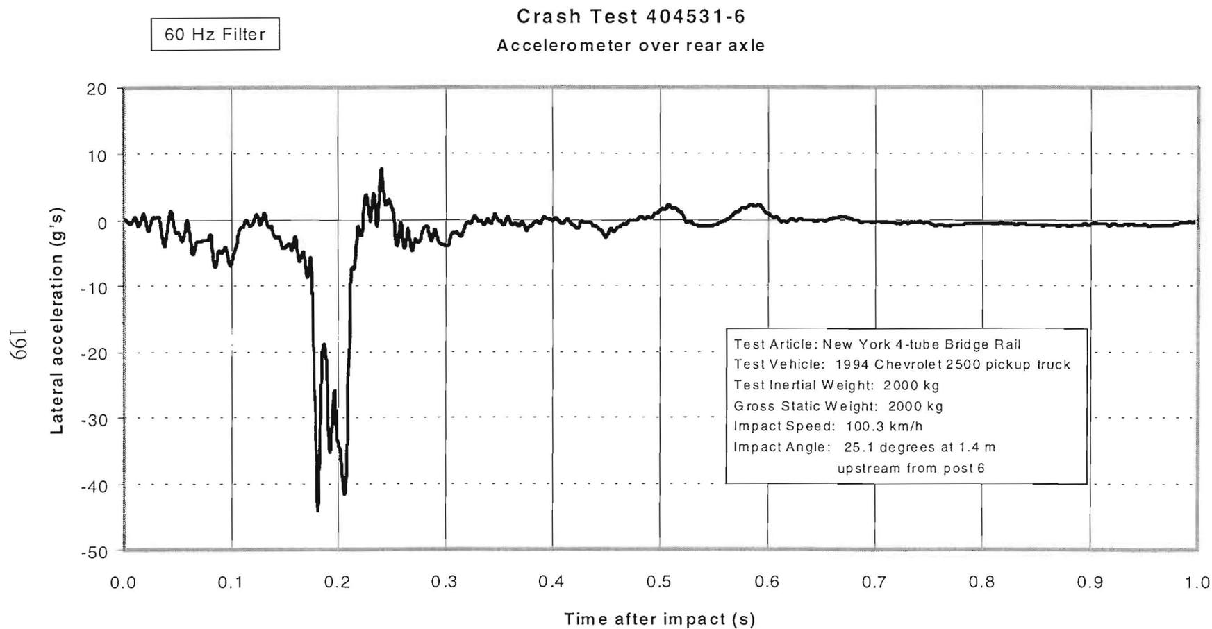
Figure 123. Vehicle lateral accelerometer trace for test 404531-6 (accelerometer located over rear axle).
