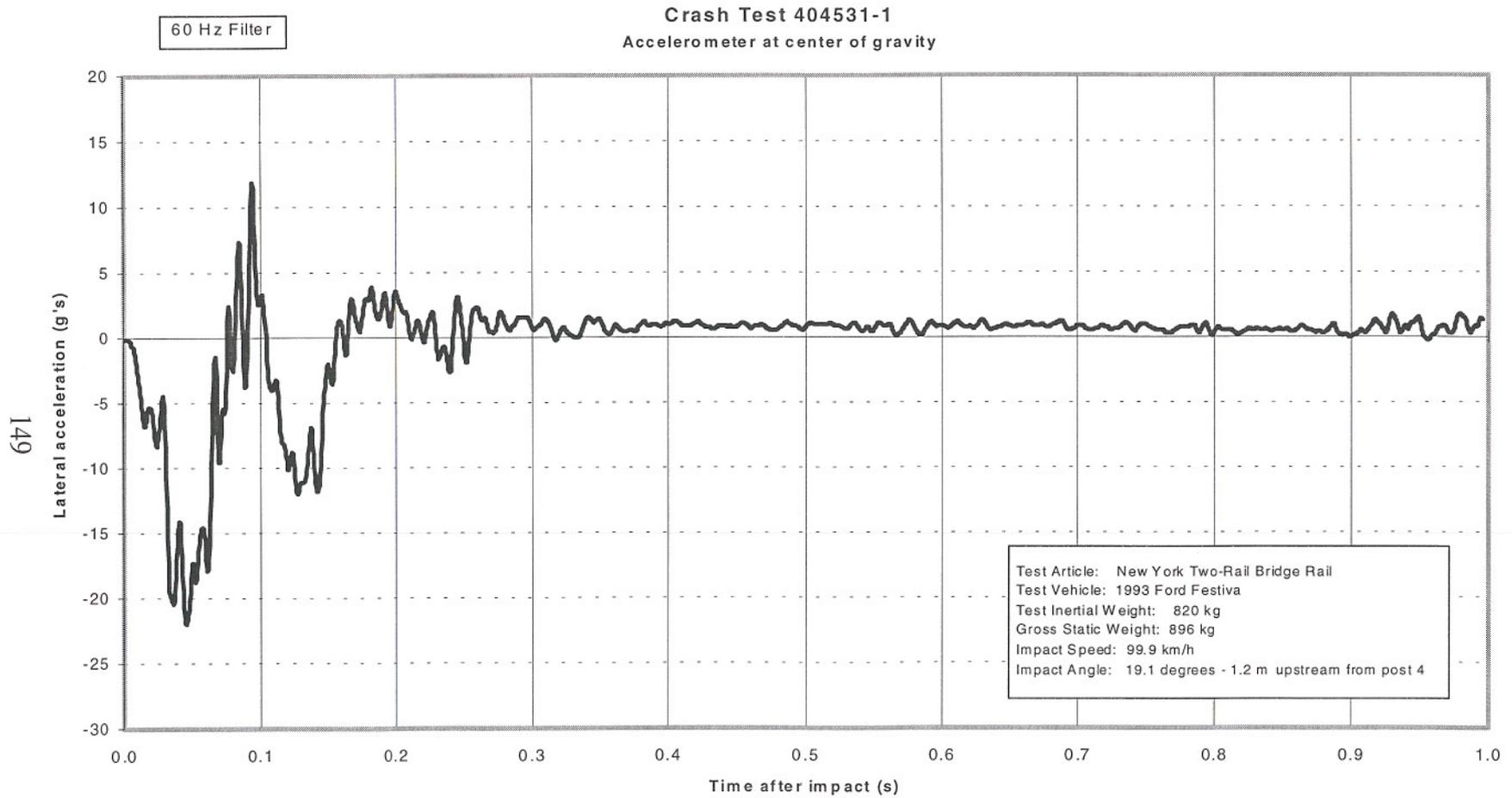
Figure 73. Vehicle lateral accelerometer trace for test 404531-1 (accelerometer located at center of gravity).
