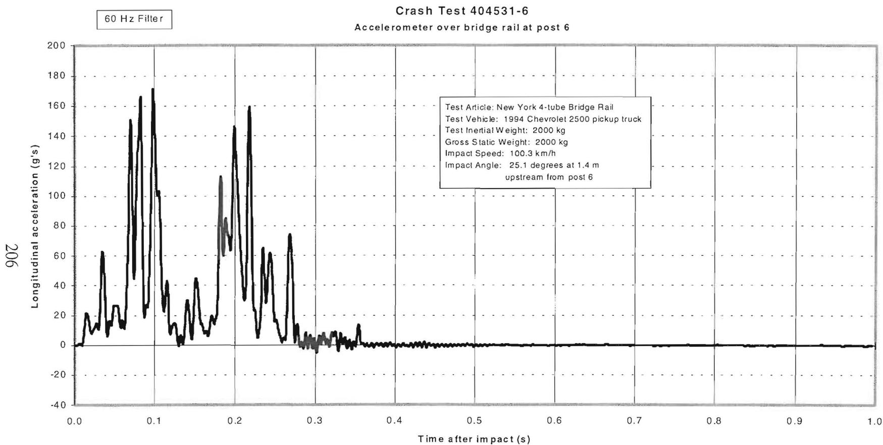
Figure 130. Bridge railing longitudinal accelerometer trace for test 404531-6 (accelerometer located over bridge railing at post 6).
