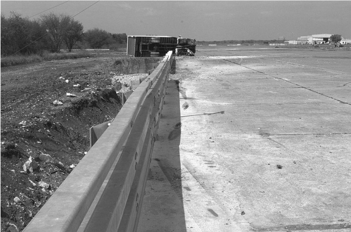
Figure 31. Vehicle trajectory path after test 404531-4.
