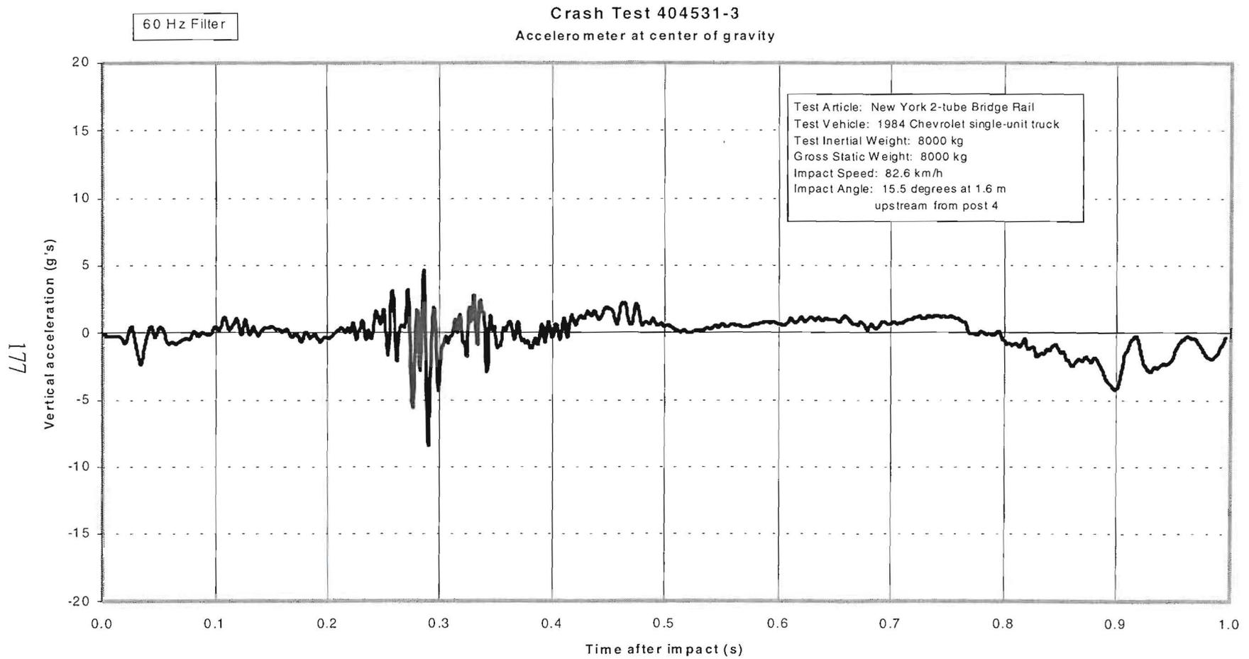
Figure 101. Vehicle vertical accelerometer trace for test 404531-3
