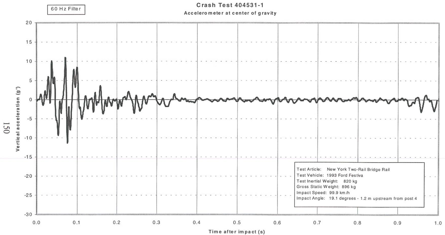
Figure 74. Vehicle vertical accelerometer trace for test 404531-1 (accelerometer located at center of gravity).
