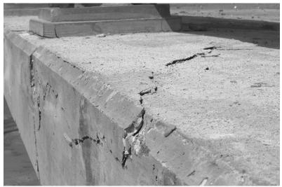
Figure 33. Damage to deck at post 3 after test 404531-4.
