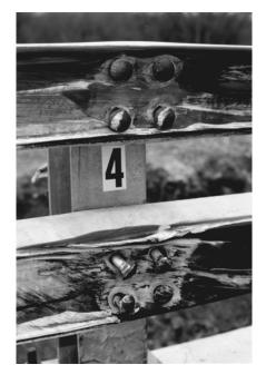
Figure 24. Damage at post 4 after test 404531-3.
