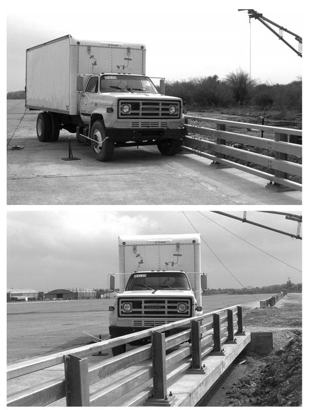
Figure 29. Vehicle/installation geometrics for test 404531-4.
