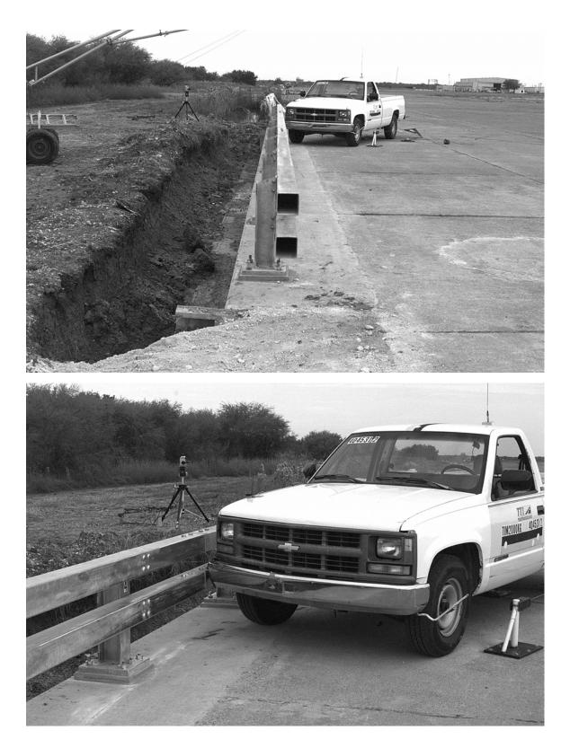
Figure 13. Vehicle/installation geometrics for test 404531-2.
