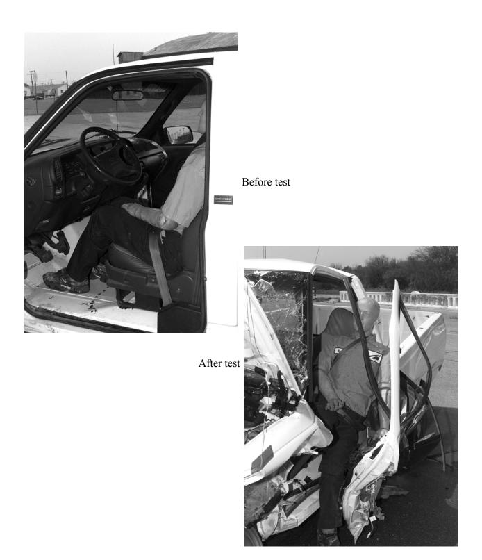
Figure 50. Interior of vehicle for test 404531-7.
