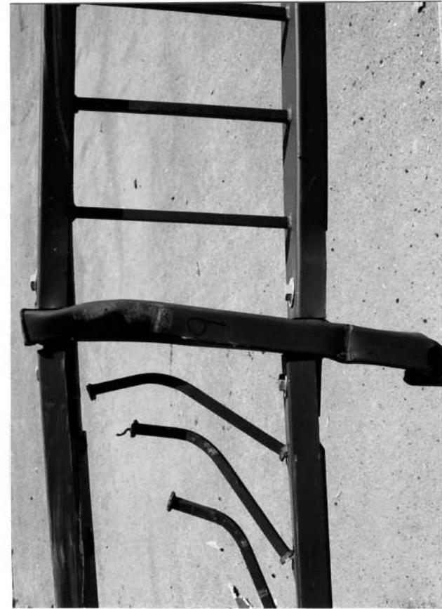
Figure 38. Post Damage, Test MNPD-2 (Continued)
