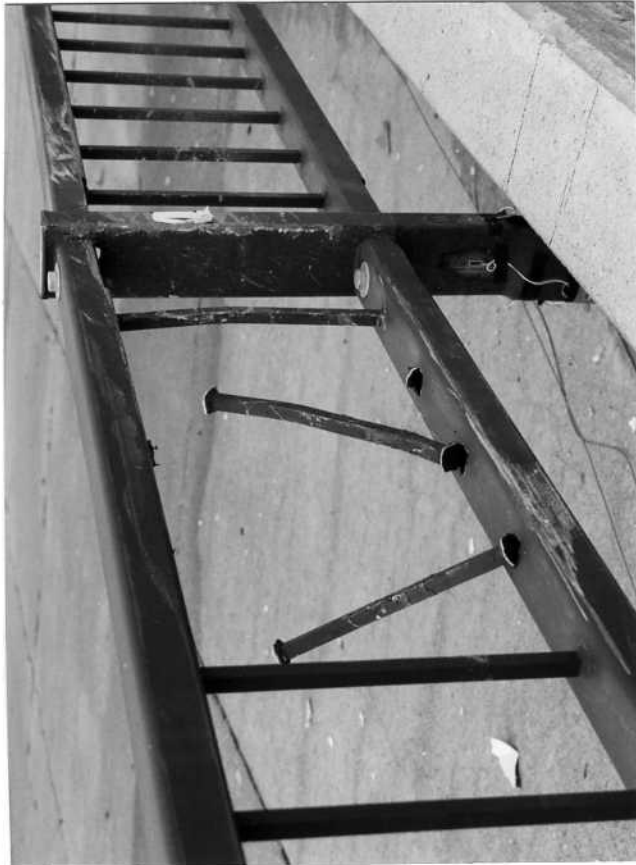
Figure 25. Barrier Damage, Test MNP-1 (Continued)
