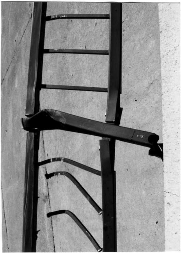
Figure 37. Post Damage, Test MNPD-2
