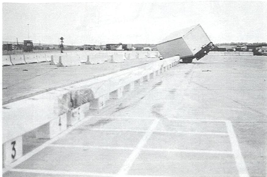
FIGURE 21. Bridge Rail Damage, Test NEOCR-3
