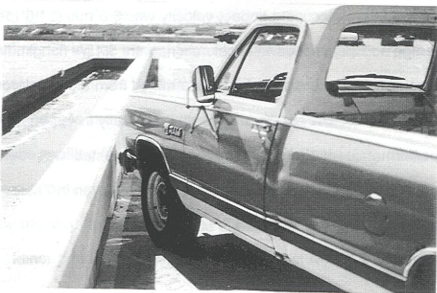
FIGURE 38. Impact Location, Test NEOCR-6
