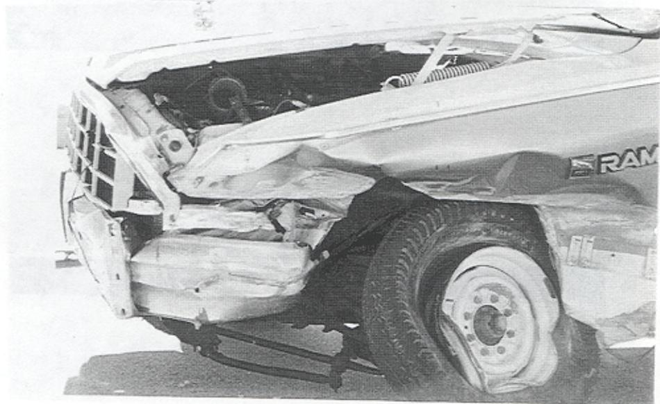
FIGURE 44. Vehicle Damage, Test NEOCR-6
