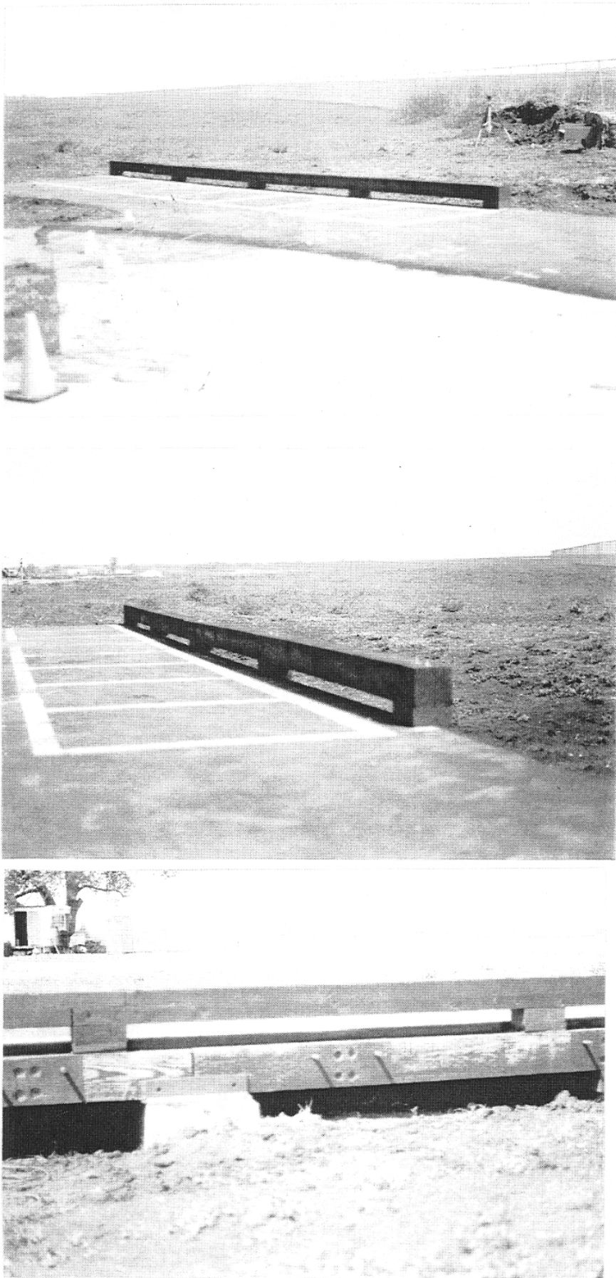
Figure 28. Square-Shape Timber Curb Rail, Test LVCS-4
