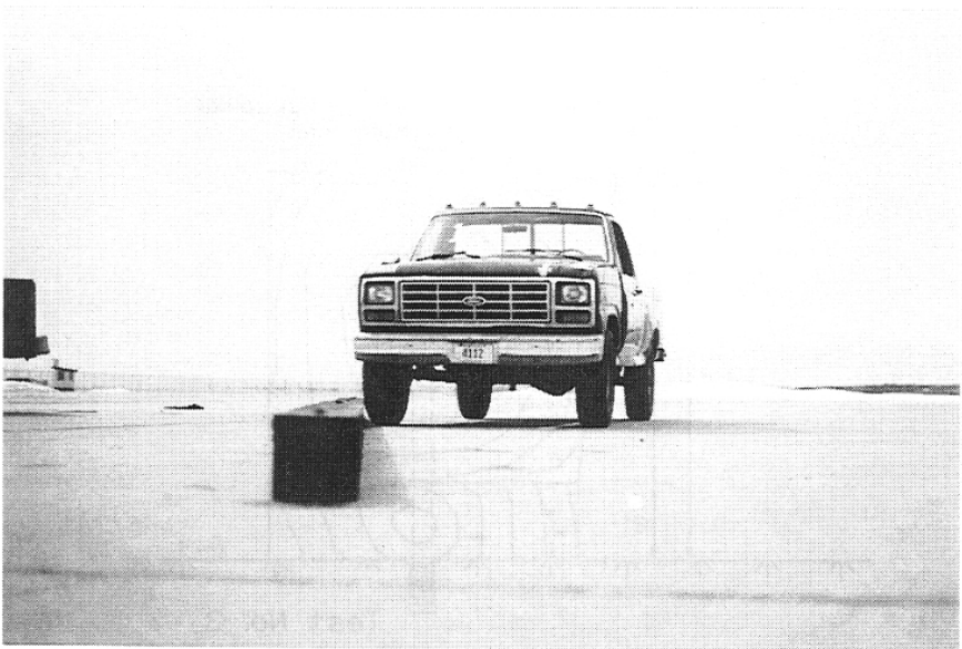
Figure 13. Square Curb Rail Attached to Concrete Apron
