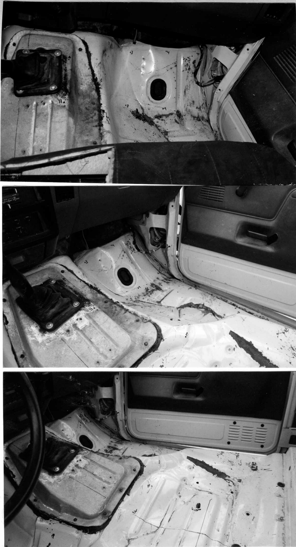
Figure 152. Occupant Compartment Deformations, Test STTR-1
