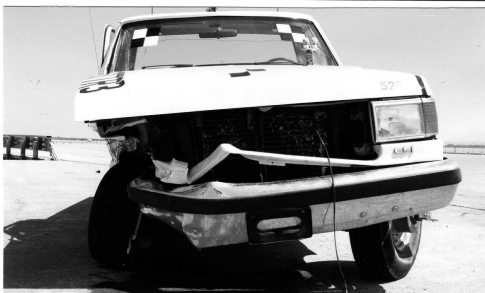
Figure 175. Vehicle Damage, Test STTR-3
