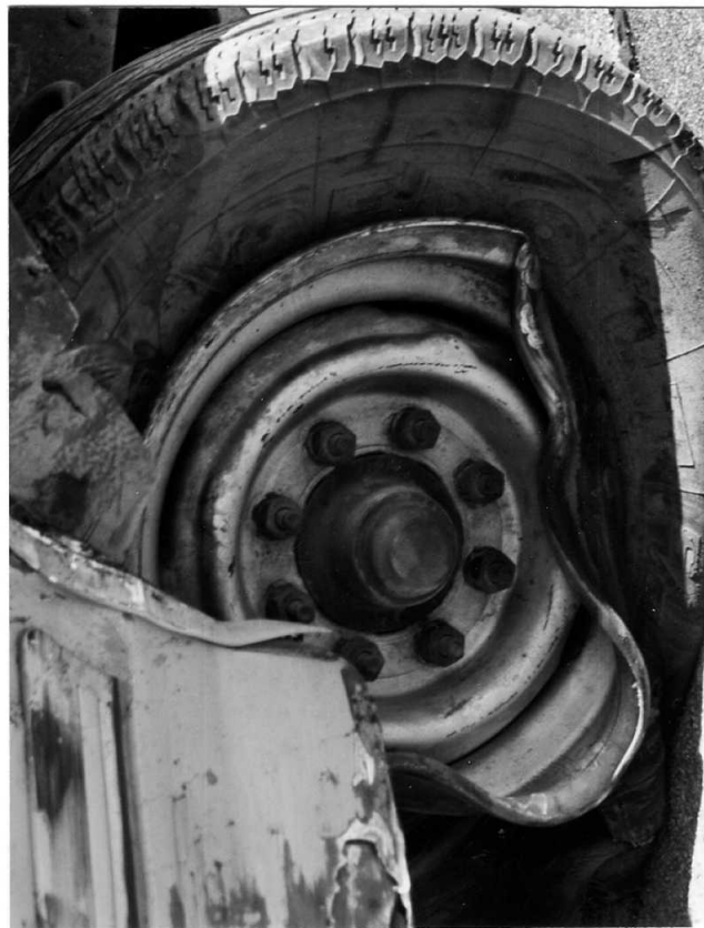
Figure 90. Front and Rear Wheel Assembly Damage, Test TRBR-2
