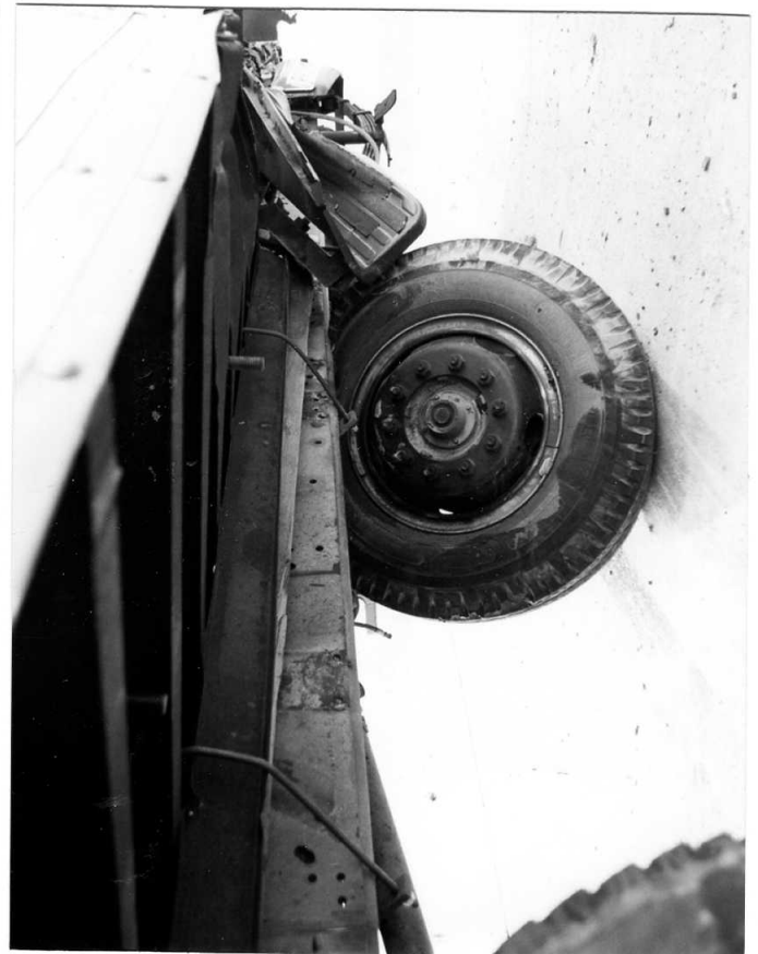
Figure 78. Damage to Truck Box Attachment Hardware, Test TRBR-1
