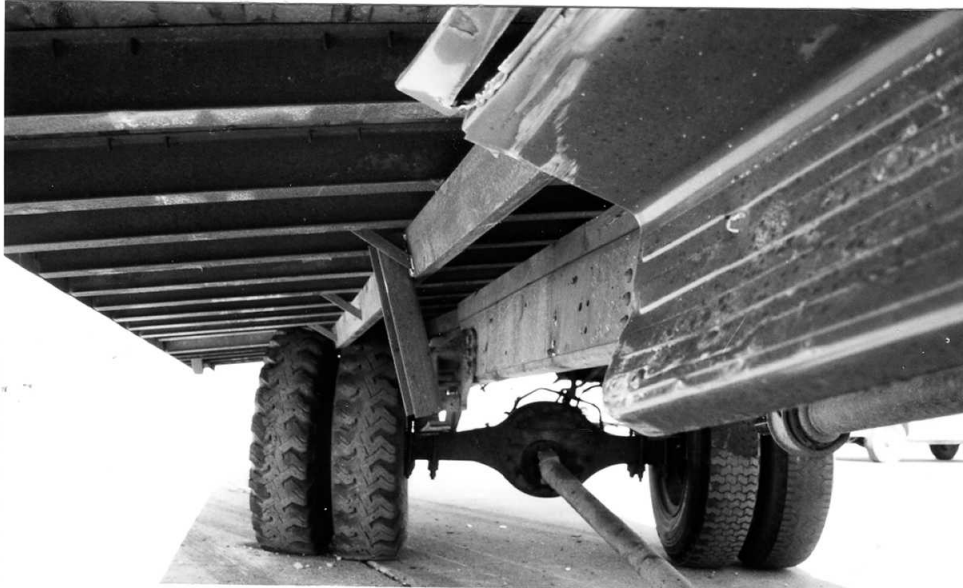
Figure 162. Truck Box and Frame Damage, Test STTR-2
