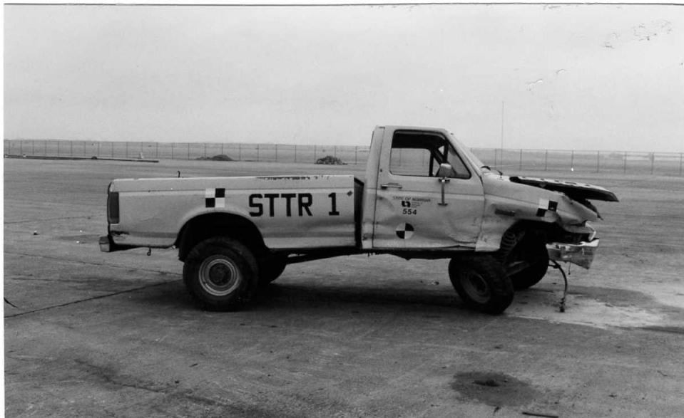
Figure 150. Vehicle Damage, Test STTR-1
