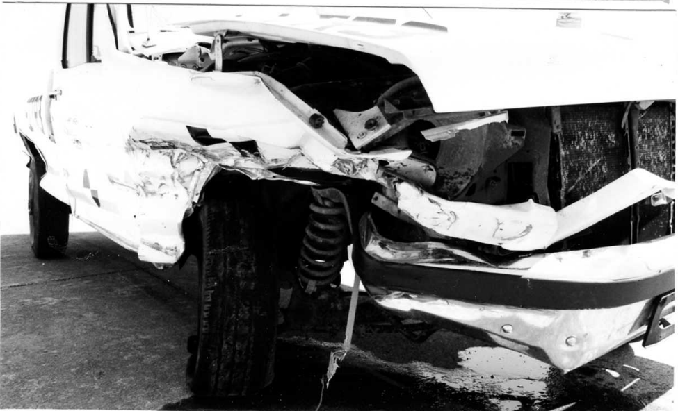
Figure 176. Vehicle Damage, Test STTR-3
