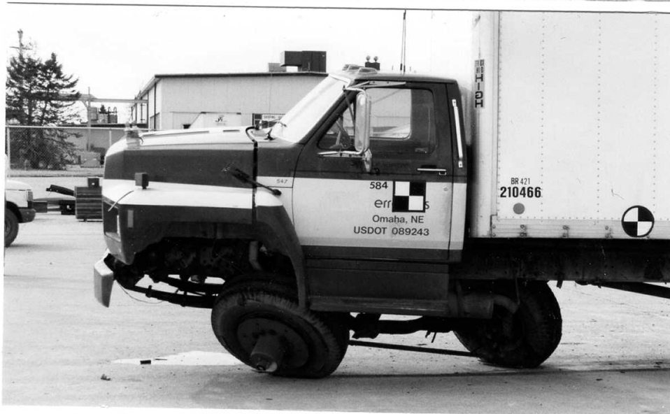
Figure 77. Front and Rear Wheel Assembly Damage, Test TRBR-1
