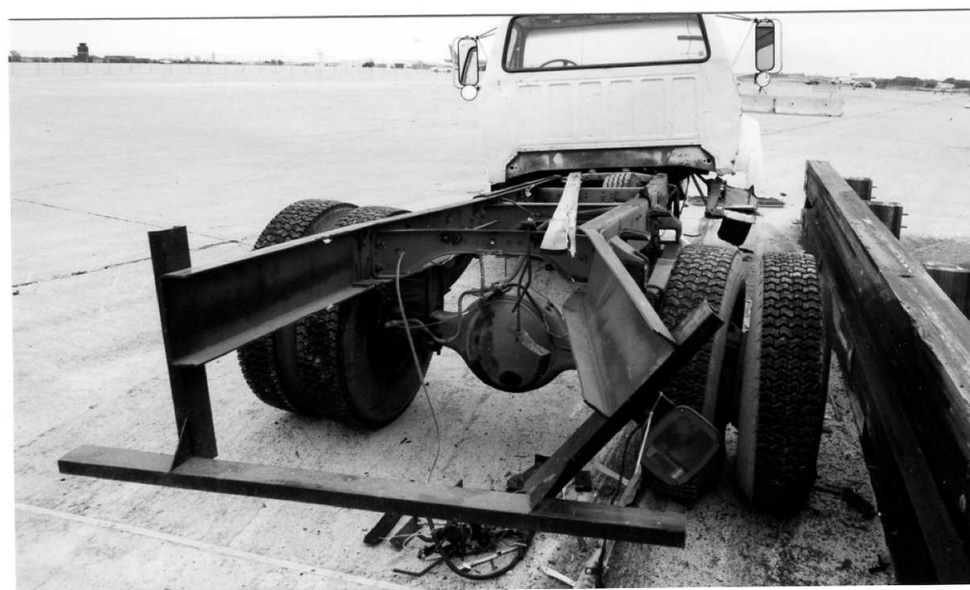
Figure 115. Vehicle Damage, Test TRBR-4
