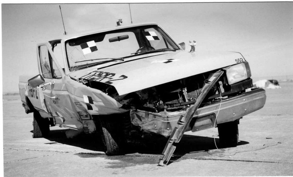
Figure 89. Vehicle Damage, Test TRBR-2
