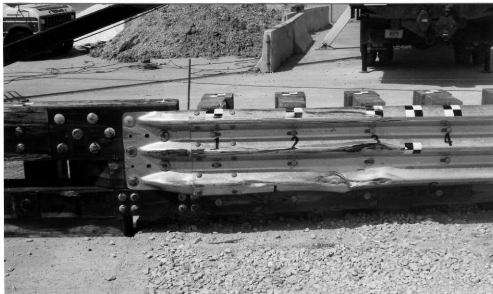
Figure 99. Barrier Damage, Test TRBR-3
