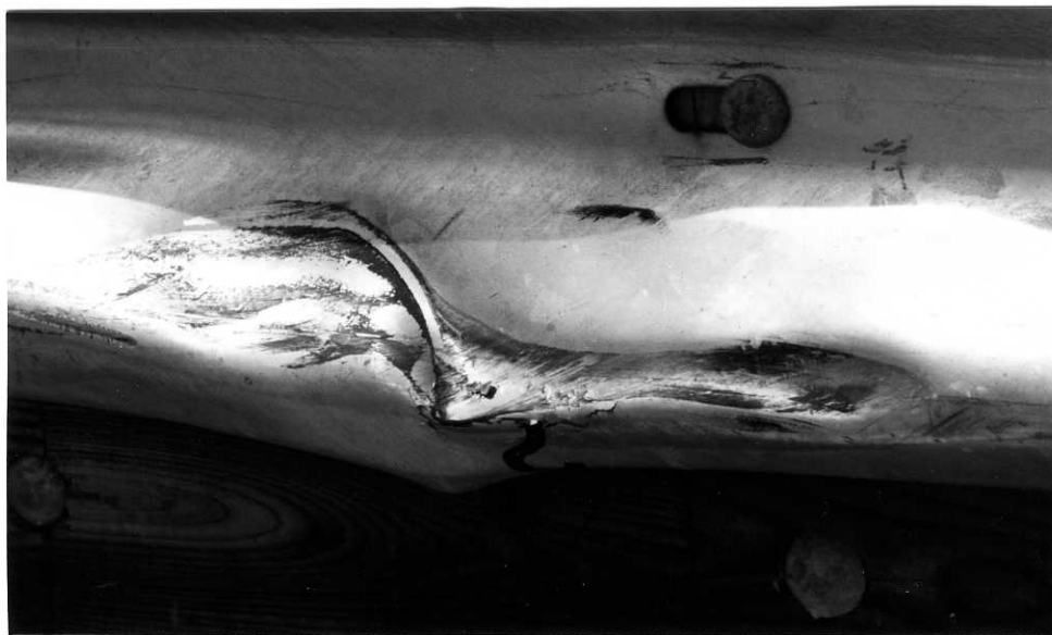
Figure 100. Thrie Beam Rail Damage, Test TRBR-3
