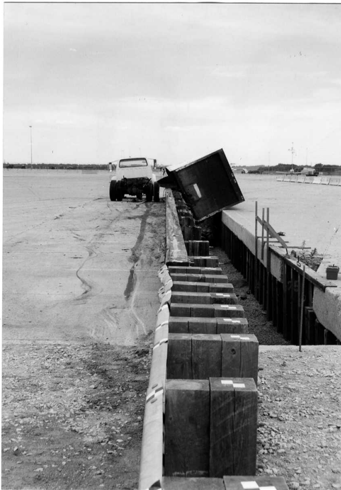
Figure 111. Final Vehicle Position, Test TRBR-4
