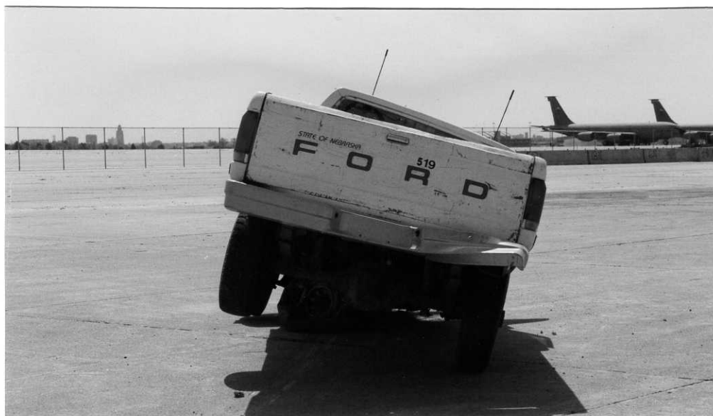
Figure 102. Vehicle Damage, Test TRBR-3
