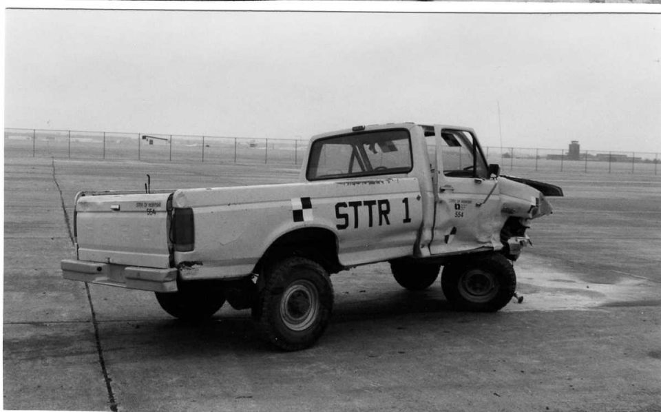
Figure 151. Vehicle Damage, Test STTR-1
