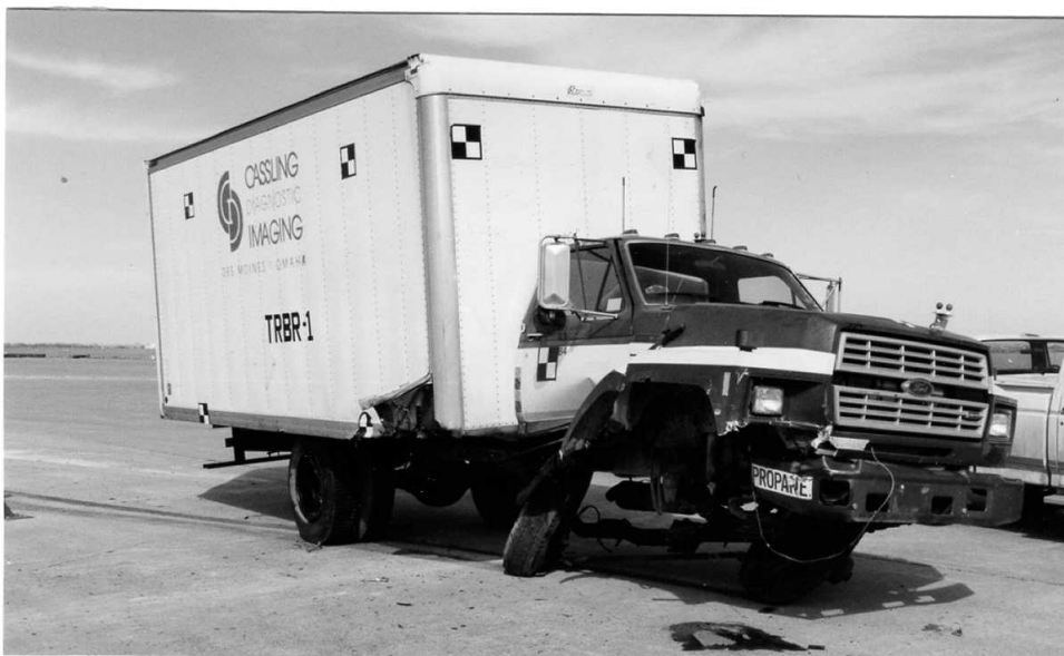
Figure 76. Vehicle Damage, Test TRBR-1
