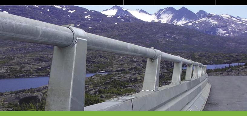
MDS bridge railing system can be utilized for new bridge construction projects or on rehabilitation bridge projects. The unique energy dissipating slip base connectors, anchored with mechanical or chemical anchors, may reduce deck damage by minimizing the force from impacts transmitted to bridge deck.
