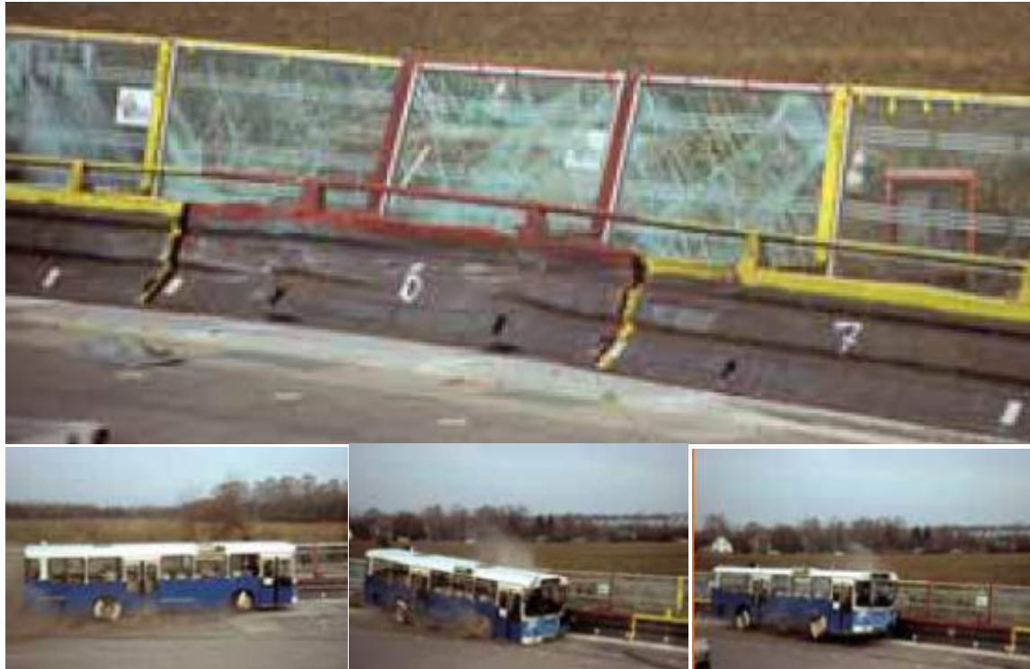
Figure 4. 13,000-kg 70 km/hr 20 degree intercity bus test of the MDS-4 barrier showing (top) barrier damage and (bottom) the vehicle-barrier interaction.
