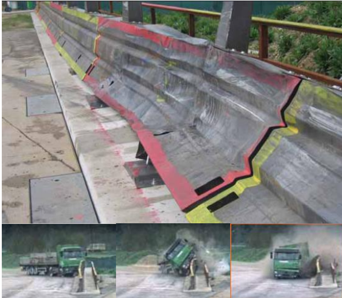
Figure 6. 38,000-kg 65-km/hr 20-degree tractor trailer truck test of the MDS-5 barrier showing (top) barrier damage and (bottom) the vehicle-barrier interaction.
