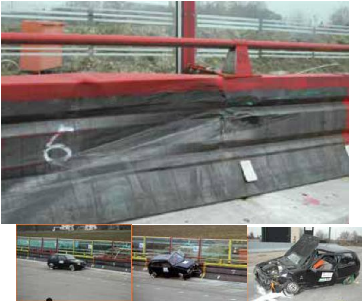
Figure 3. 900-kg 100 km/hr 20 degree small car test of the MDS-4 barrier showing (top) barrier damage, (bottom left and middle) vehicle-barrier interaction and (bottom right) vehicle damage.
