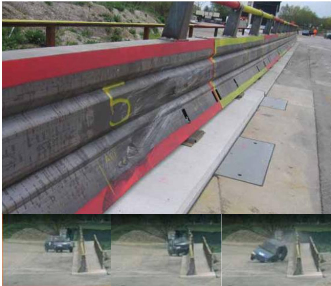
Figure 5. 900-kg 100 km/hr 20 degree small car test of the MDS-5 barrier showing (top) barrier damage and (bottom) the vehicle-barrier interaction.
