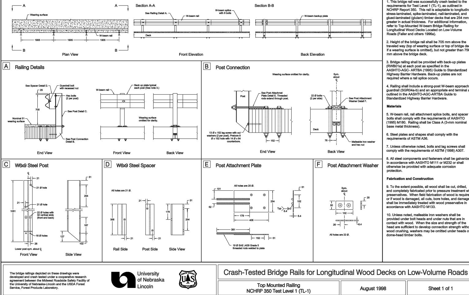
2. Height of the bridge rail shall be 705 mm above the traveled way (top of wearing surface or top of bridge deck if a wearing surface is omitted), but not greater than 756mm above the bridge deck.
