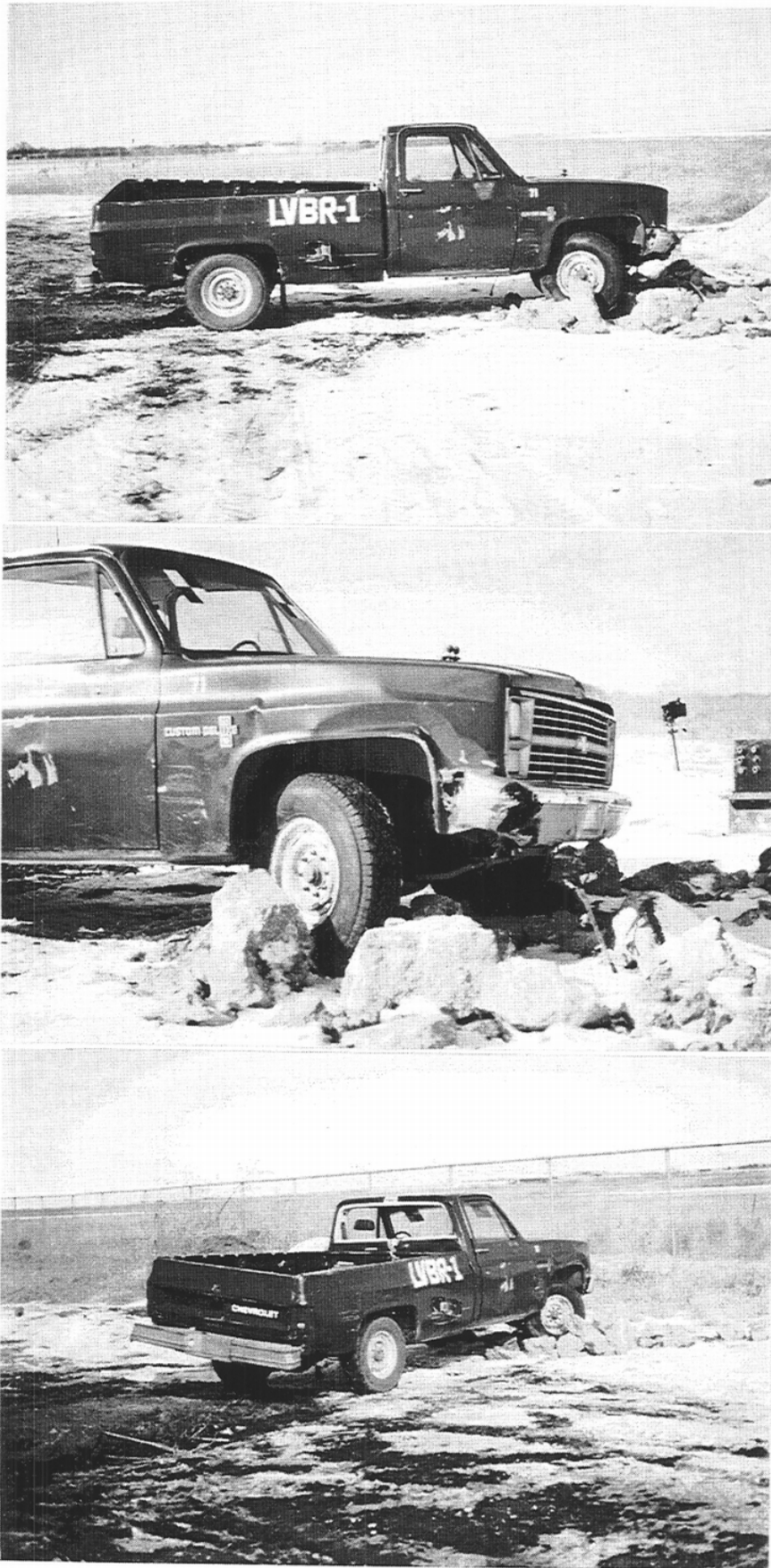
Figure 20. Vehicle Damage, Test LVBR-1
