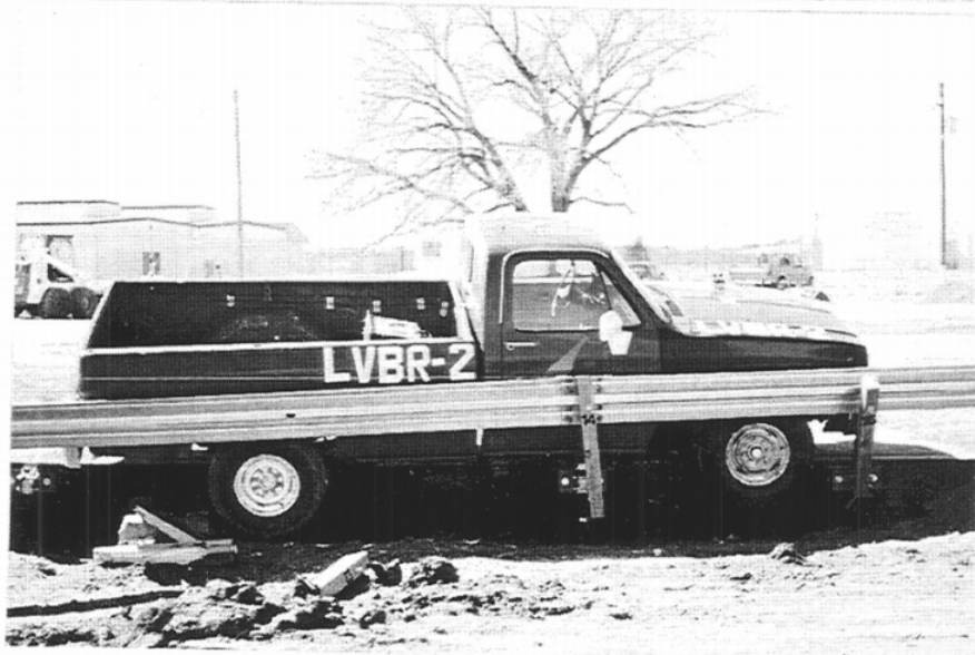
Figure 33. Vehicle Damage, Test LVBR-2
