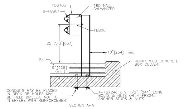
Note: Either through bolt or epoxy anchor with minimum 8" [203] embedment and minimum 1,300 psi [9.0 MPa] bond strength.
