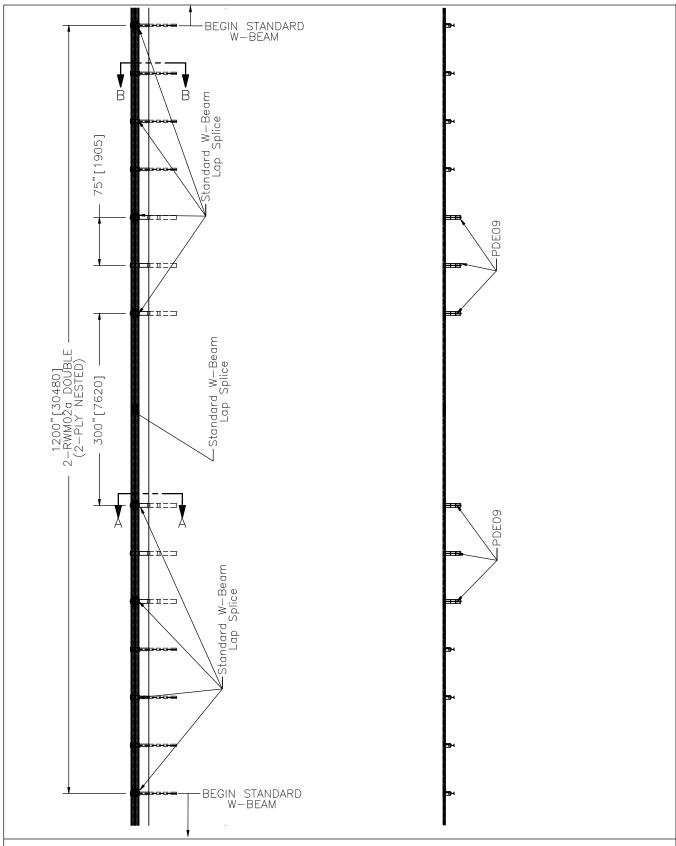
25' [7.62 m] LONG-SPAN, W-BEAM WITH 100' [30.48 m] NESTED RAIL
