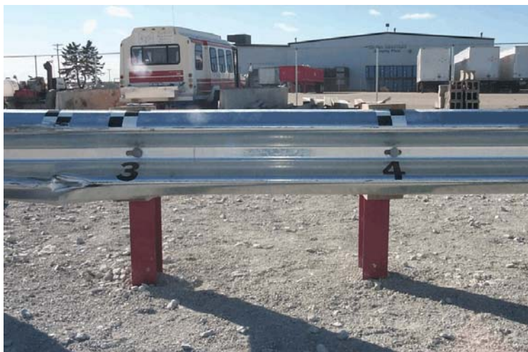
Figure 125. Barrier Damage, Test WRBP-2
