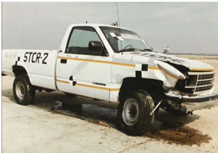
Figure 81. Vehicle Damage, Test STCR-2
