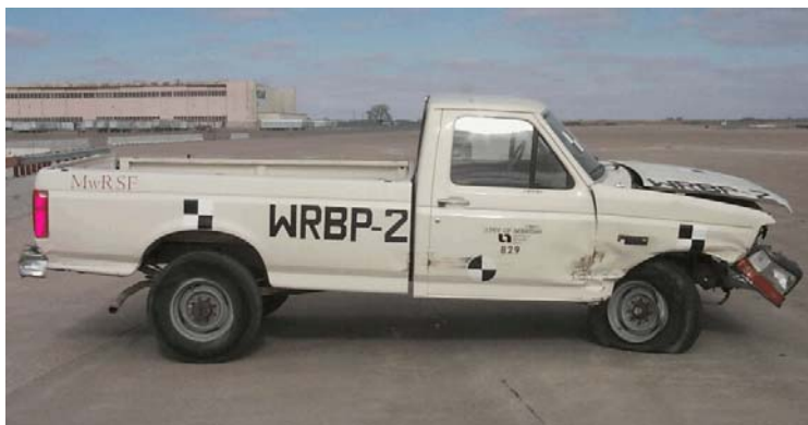
Figure 128. Vehicle Damage, Test WRBP-2
