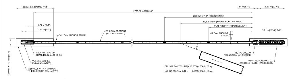
EQUIVALENT EN 1317 TEST TB51(H2) CONDUCTED IN SUB-STITUTION FOR REQUIRED NCHRP REPORT 350 TEST 4-12
