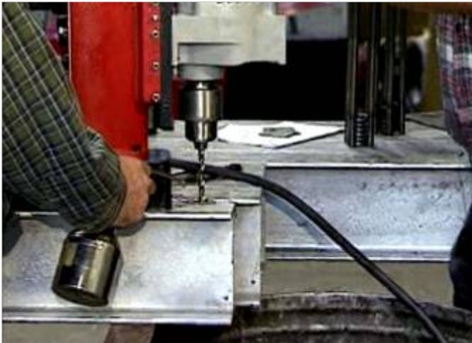
6. Drill holes for hinges & brackets into the flanges of the post section as shown in the Break-Safe Design Book page. (Your steel post supplier can also do this for you.)
