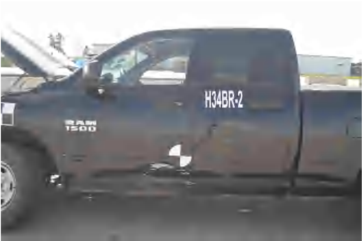
Figure 62. Vehicle Damage, Test No. H34BR-2
