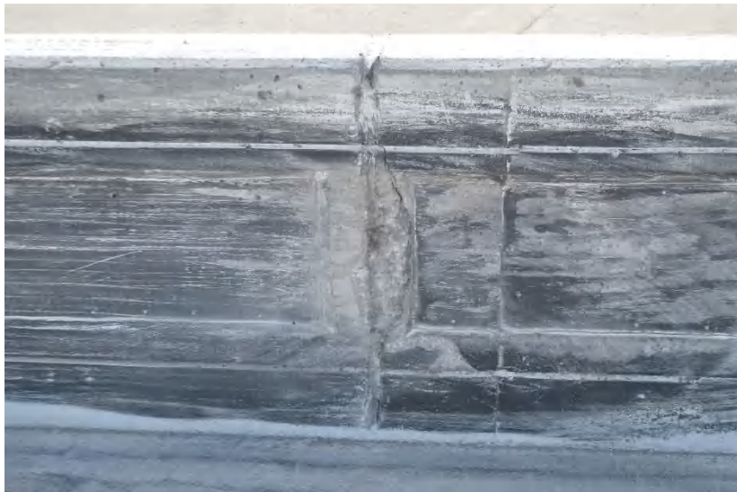
Figure 57. Traffic-Side System Damage, Test No. H34BR-2
