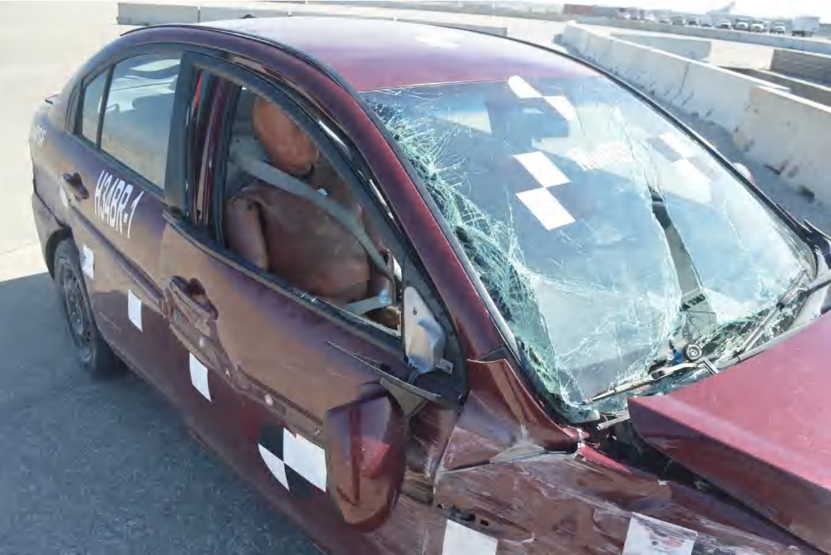
Figure 43. Vehicle Damage, Test No. H34BR-1
