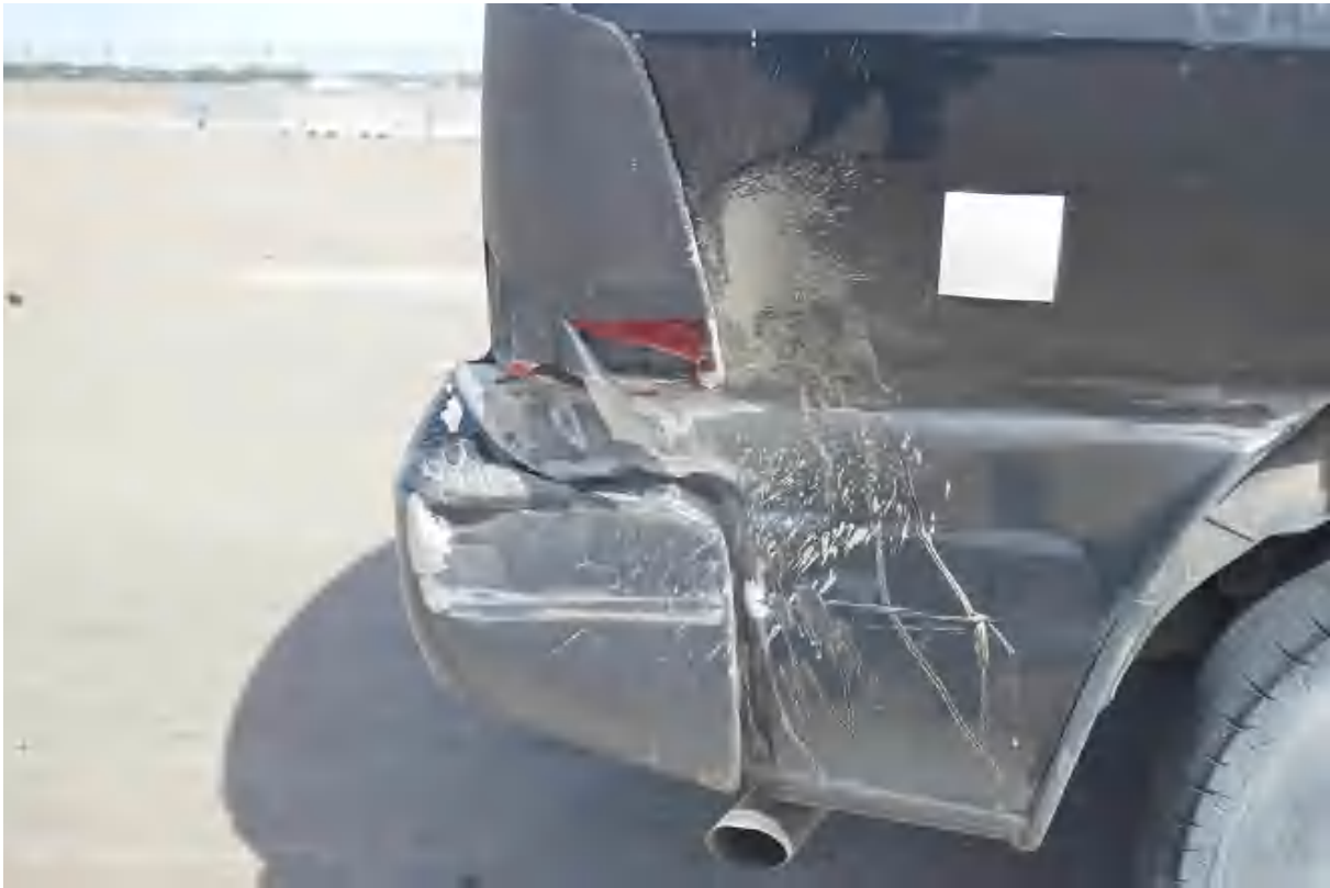
Figure 61. Vehicle Damage, Test No. H34BR-2
