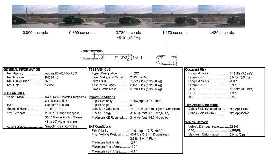
\*MASH 2016 Table 2-5 has a unit conversion discrepancy in the "Acceptable KE" (impact severity) maximum value for Test 3-60. The value in the table is 41 kJ, however 34 kip-ft. converts to 46 kJ
