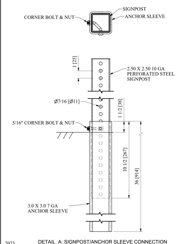
DETAIL A: SIGNPOST/ANCHOR SLEEVE CONNECTION
